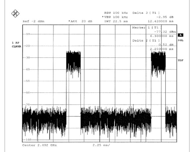
$20\log(\text{Duty cycle}) = 20\log\frac{2.25 \text{ ms}}{12.42 \text{ ms}} = -14.83 \text{dB}$
