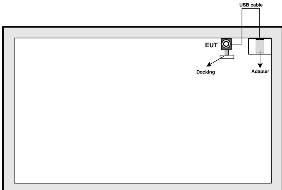
**Test Setup Diagram - Radiated Emission Below 1GHz (Mode 2)**
