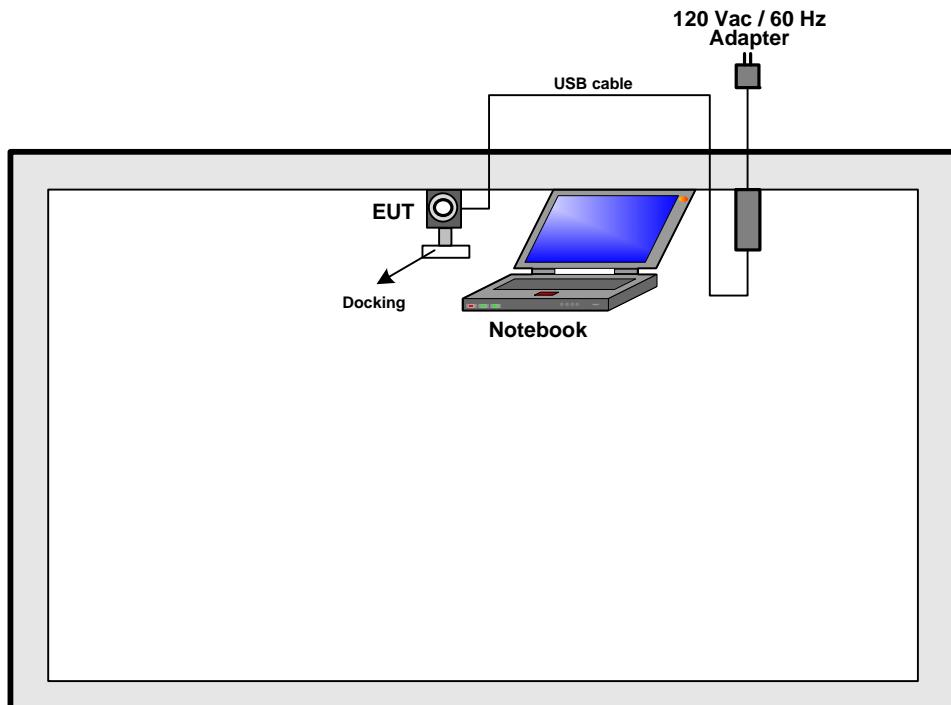
**Test Setup Diagram - Radiated Emission Above 1GHz (Mode 1)**
