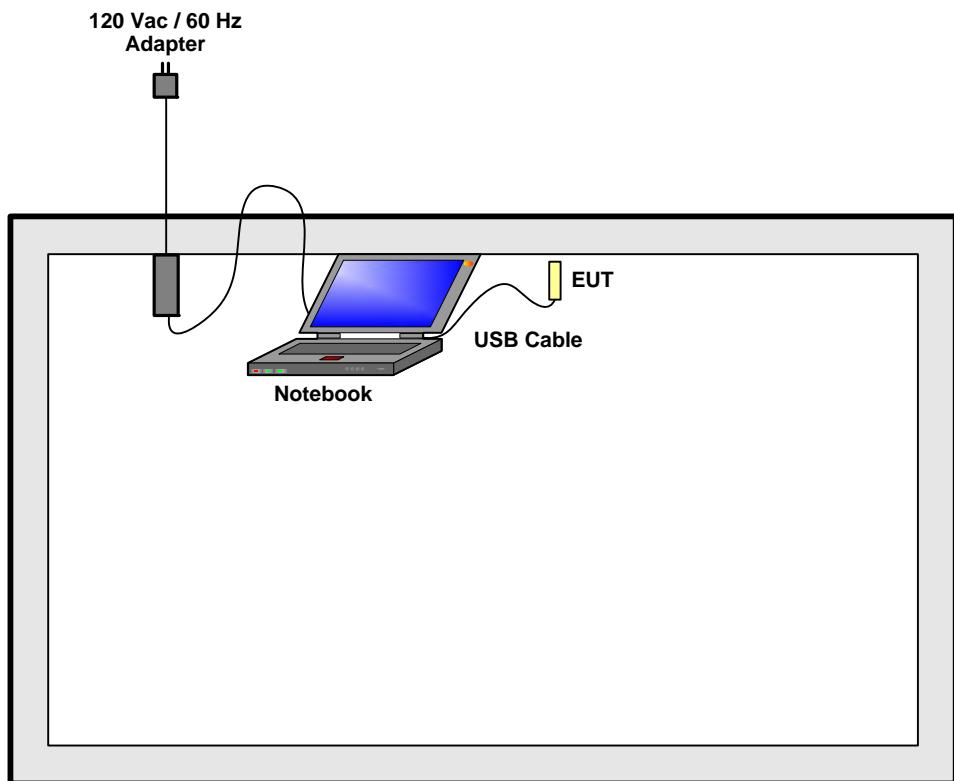
**Test Setup Diagram - Radiated Emission (Above 1GHz)**
