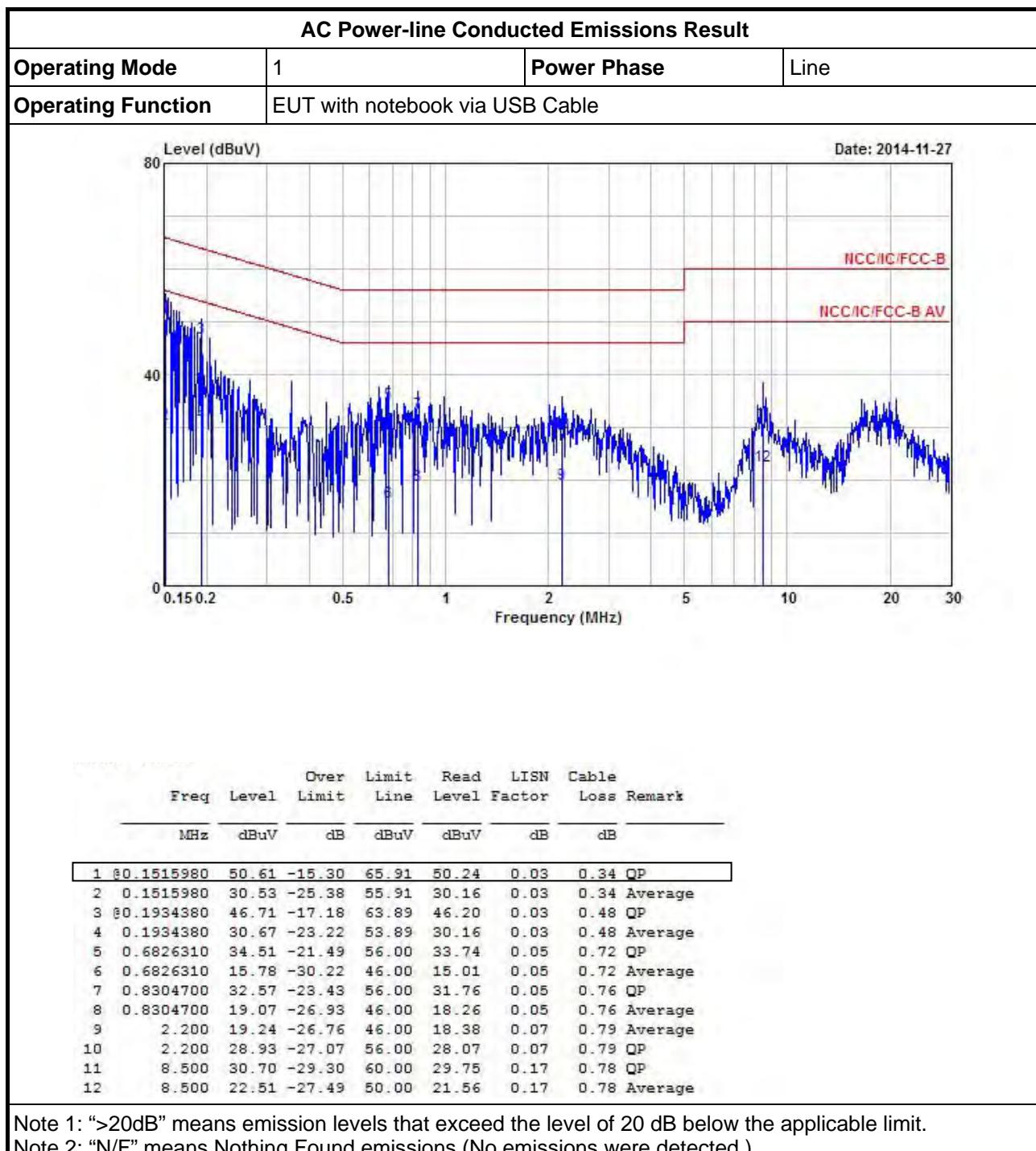
Note 1: ">20dB" means emission levels that exceed the level of 20 dB below the applicable limit.
