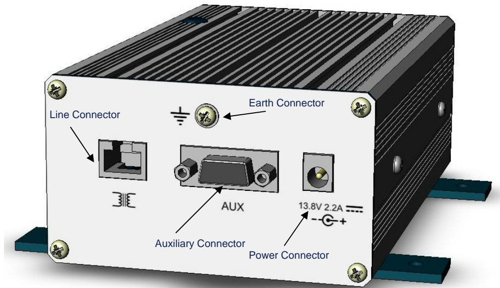
The transmitter requires 13.8VDC at about 2.1A. The DC input to the transmitter is via a 2.1mm connector. To fit the locking type connector to the transmitter, push the connector in and turn it until the two locking lugs enter the socket and none of the connector barrel is visible. Then turn the connector a quarter turn clockwise.
