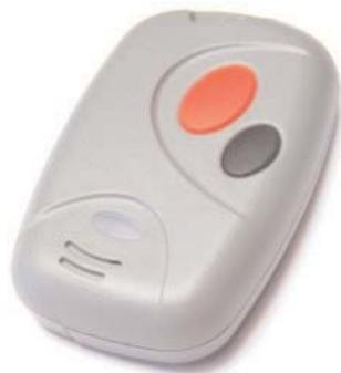
Enabling of Call Fob features is by Hub configuration. All Call Fobs are physically identical and support the same features (if enabled at the Hub).
