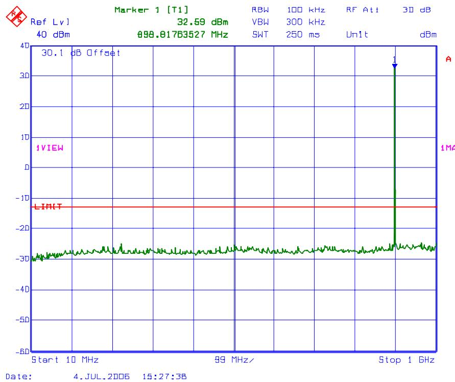
**PLOT # 84    Conducted Spurious Emissions with 3 RF signal inputs/outputs**
