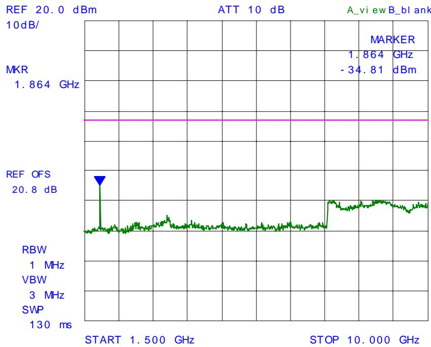
**PLOT # 111 Conducted Spurious Emissions with 2 RF signal inputs/outputs**
