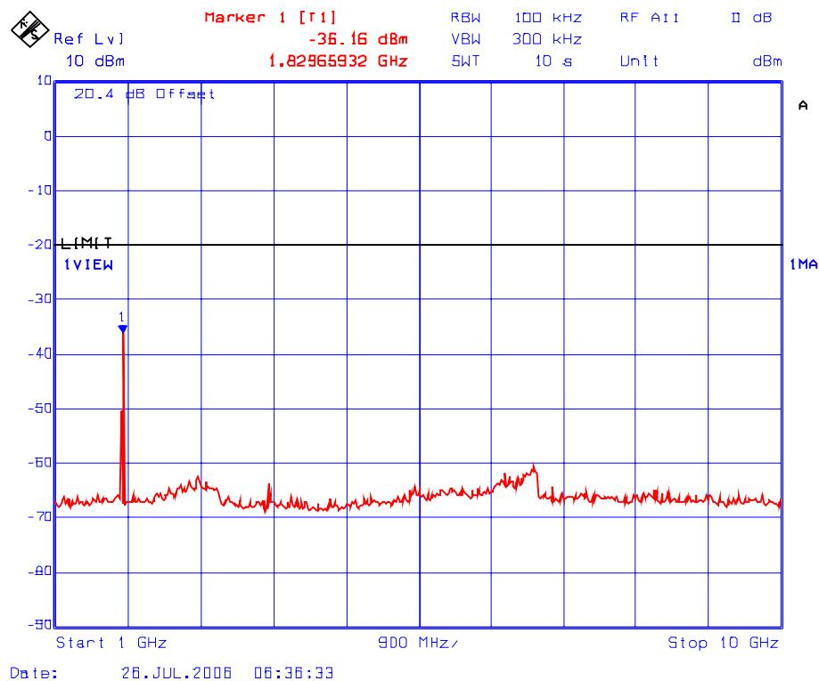
**PLOT # 97    Conducted Spurious Emissions with 1 RF signal input/output
