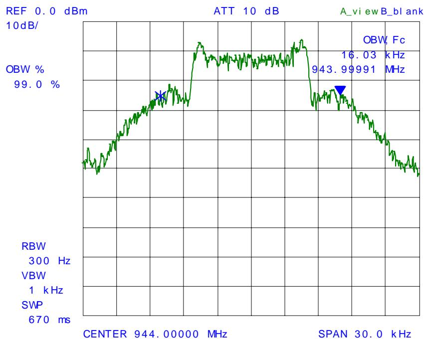
**PLOT # 54** 99% Occupied Bandwidth – RF Output Signal
