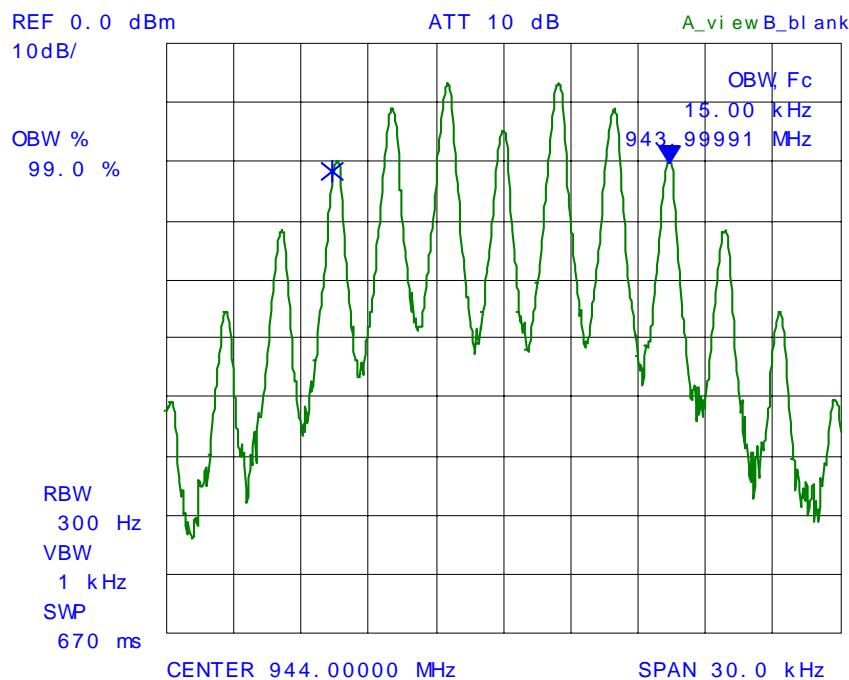
**PLOT # 50 99% Occupied Bandwidth – RF Output Signal**
