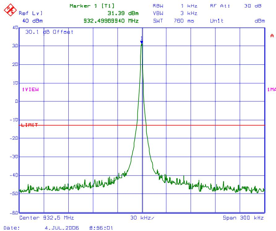
PLOT #: 23 Intermodulation with 2 RF signal inputs/outputs
