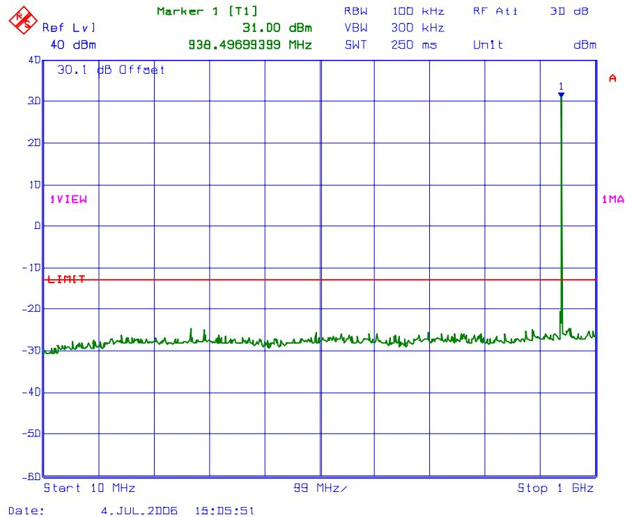
**PLOT # 104 Conducted Spurious Emissions with 1 RF signal input/output
