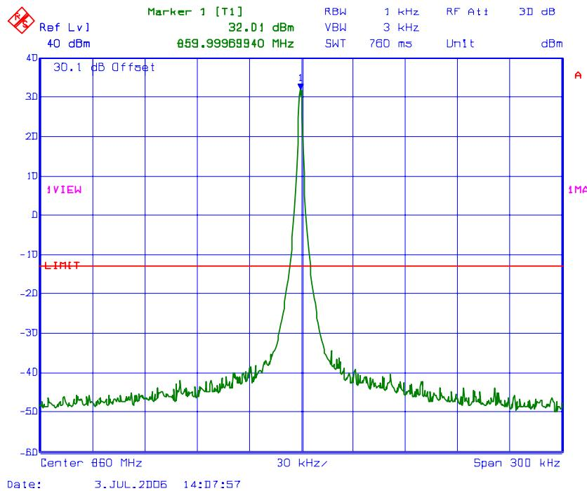
**PLOT#:** 8 **Intermodulation with 2 RF signal inputs/outputs**
