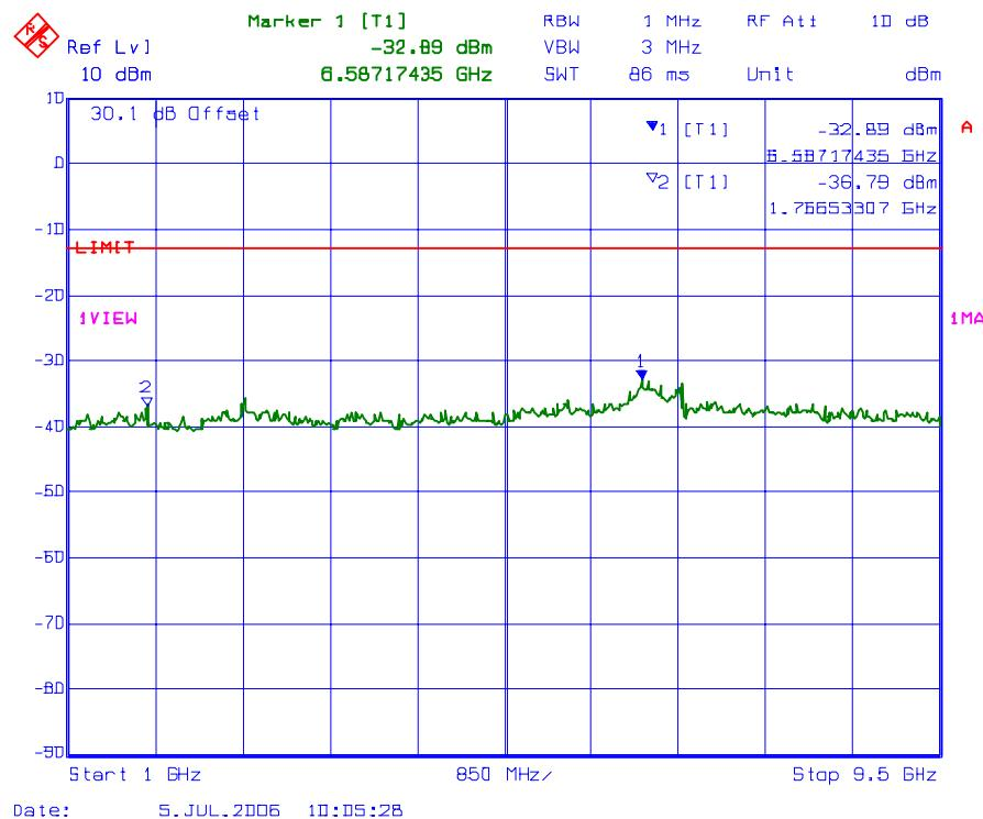
**PLOT # 79    Conducted Spurious Emissions with 1 RF signal input/output
