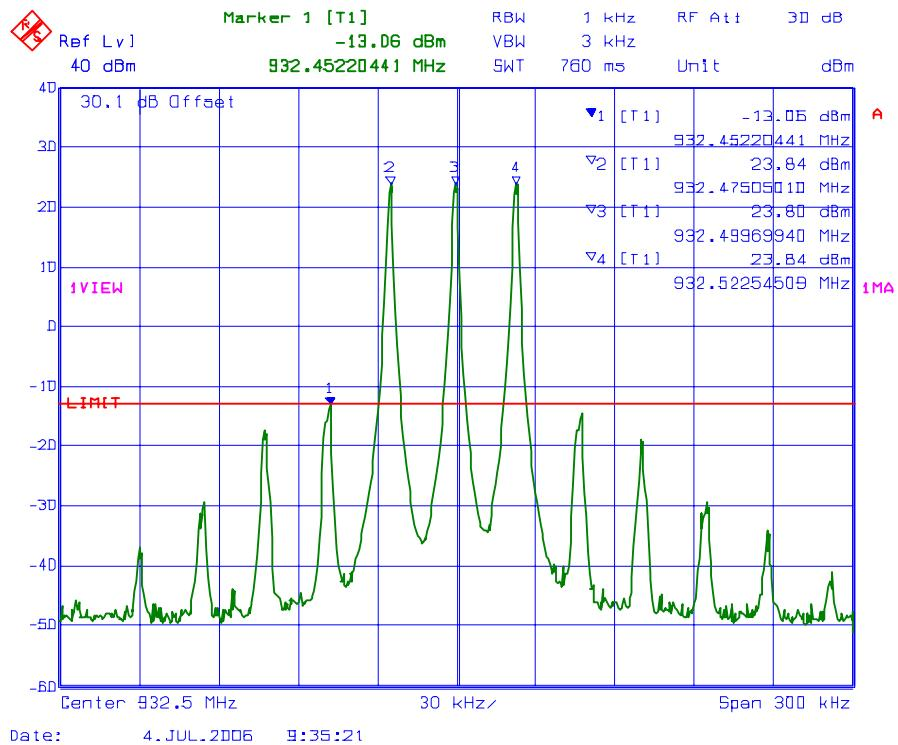
**PLOT #: 25** Intermodulation with 1 RF signal input/output
