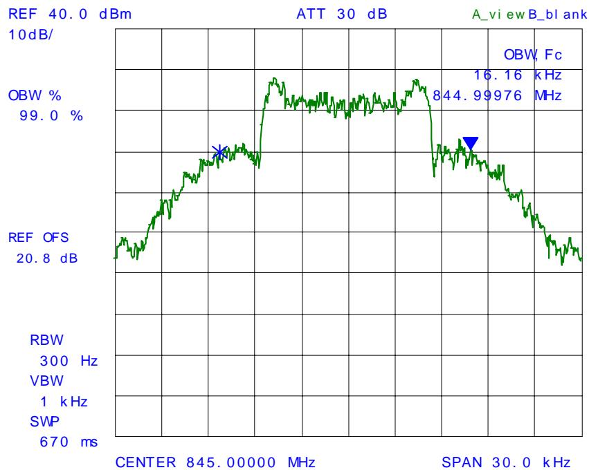
**PLOT # 47 99% Occupied Bandwidth – RF Input Signal**
