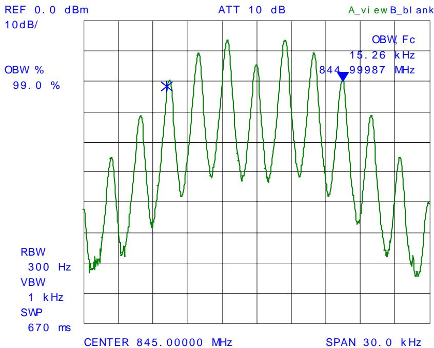
**PLOT # 42** 99% Occupied Bandwidth – RF Output Signal
