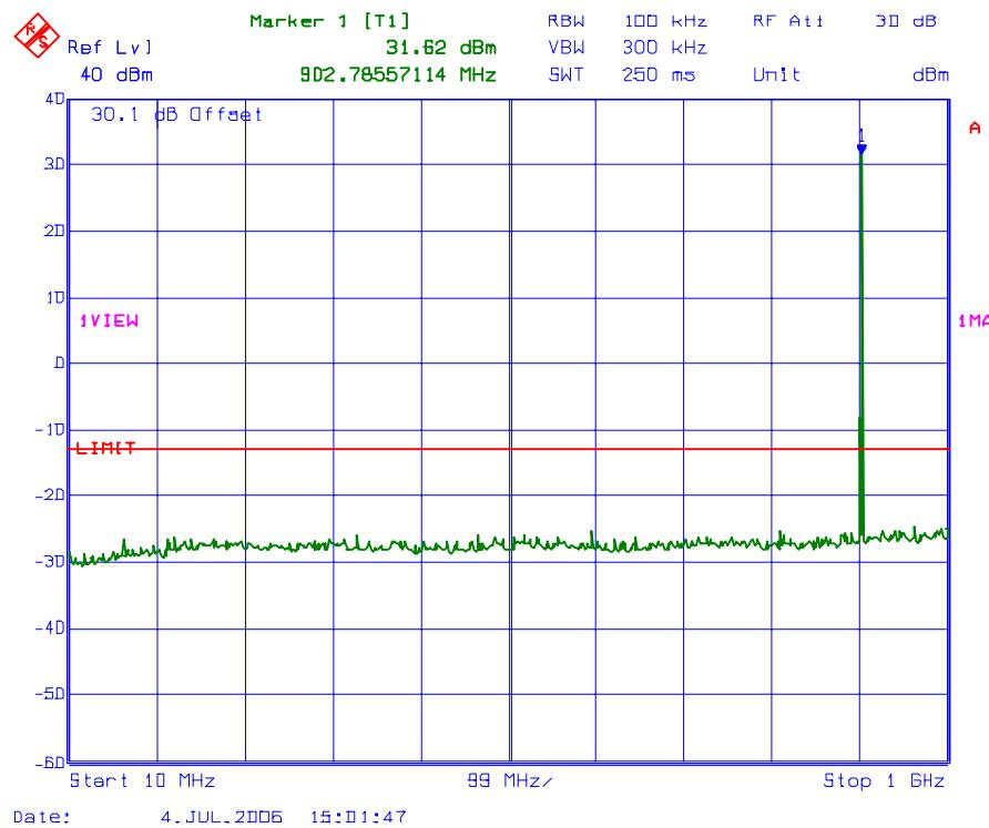
**PLOT # 86    Conducted Spurious Emissions with 1 RF signal input/output
