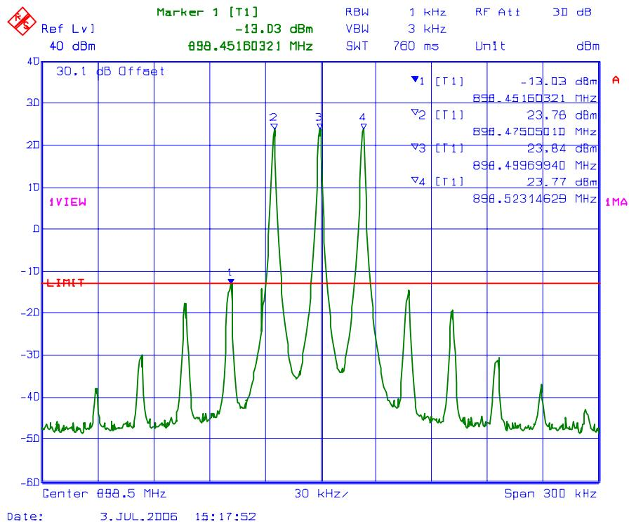
**PLOT #: 16 Intermodulation with 1 RF signal input/output**
