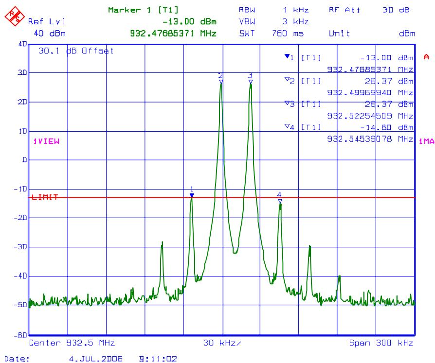
**PLOT #: 24** Intermodulation with 3 RF signal inputs/outputs
