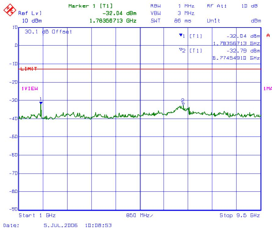
**PLOT # 85    Conducted Spurious Emissions with 1 RF signal input/output
