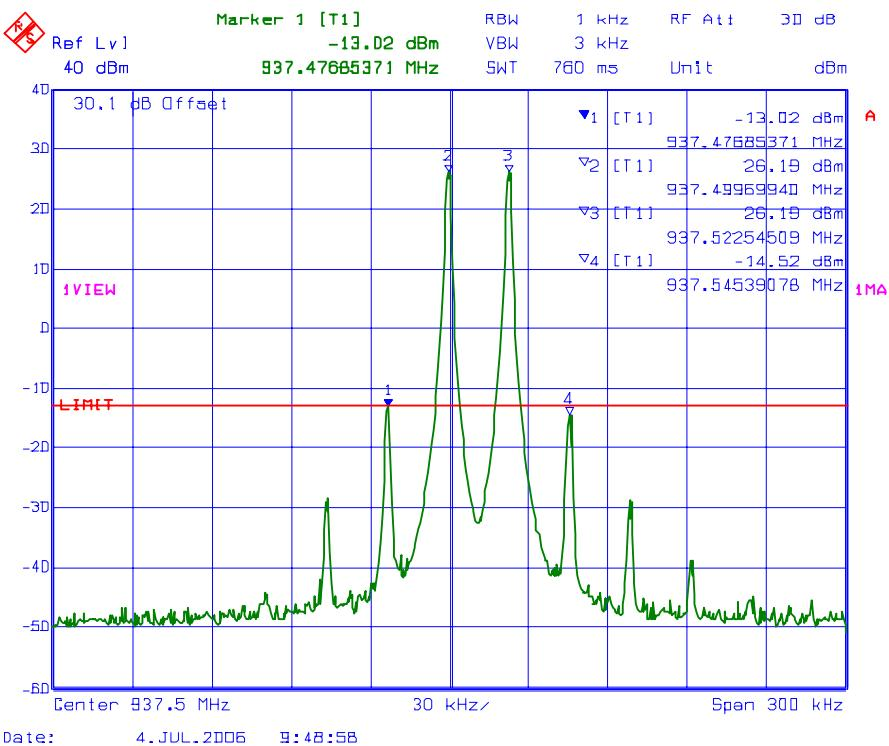
**PLOT #: 27** Intermodulation with 3 RF signal inputs/outputs
