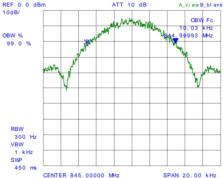
**PLOT # 44 99% Occupied Bandwidth – RF Output Signal**
