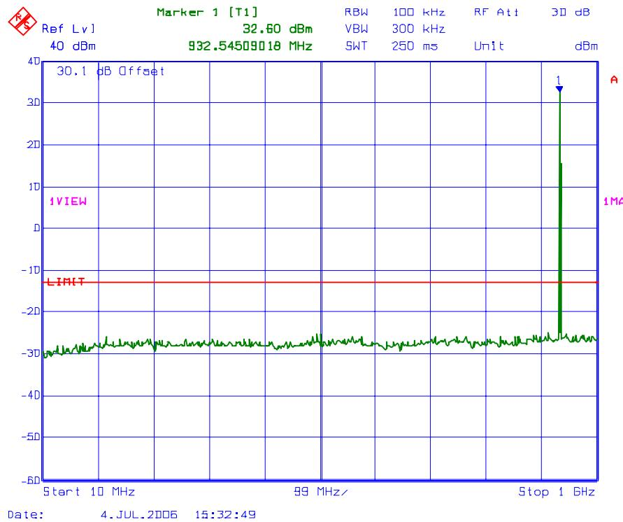
**PLOT # 102 Conducted Spurious Emissions with 3 RF signal inputs/outputs**
