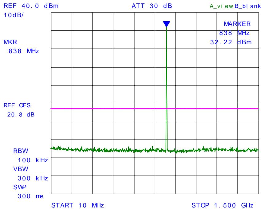
**PLOT # 62      Conducted Spurious Emissions with 1 RF signal input/output
