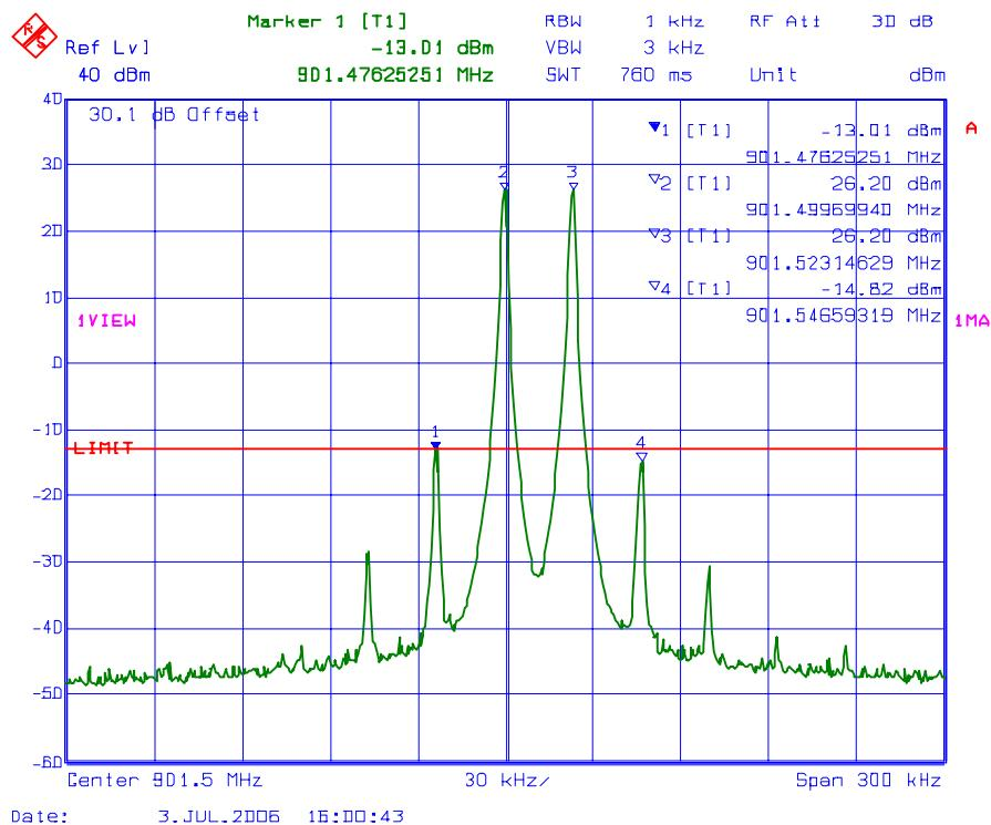
**PLOT #: 18** Intermodulation with 3 RF signal inputs/outputs
