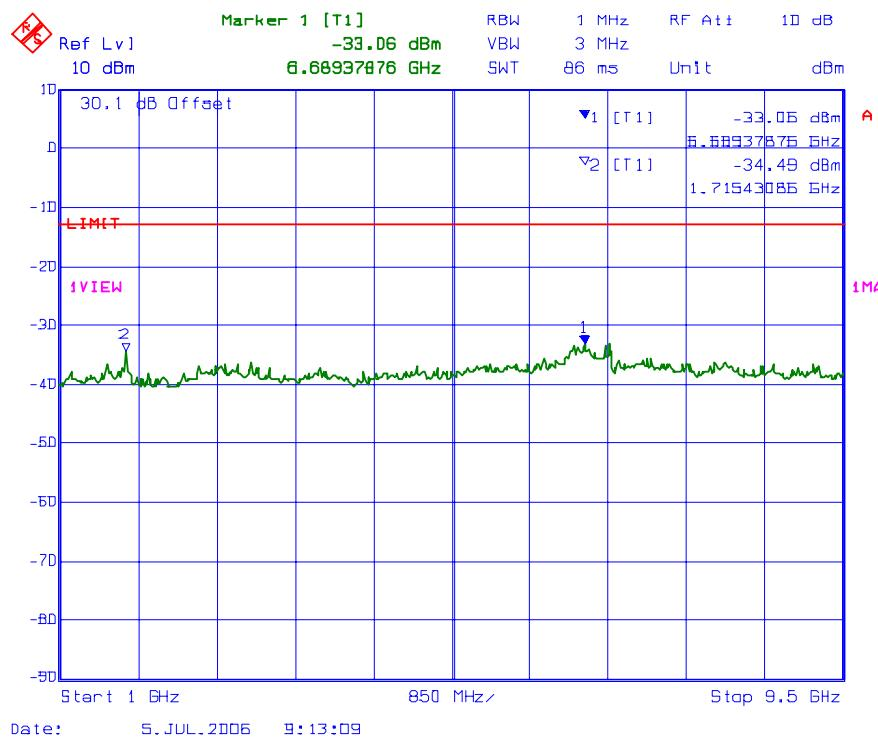
**PLOT # 71    Conducted Spurious Emissions with 3 RF signal inputs/outputs**
