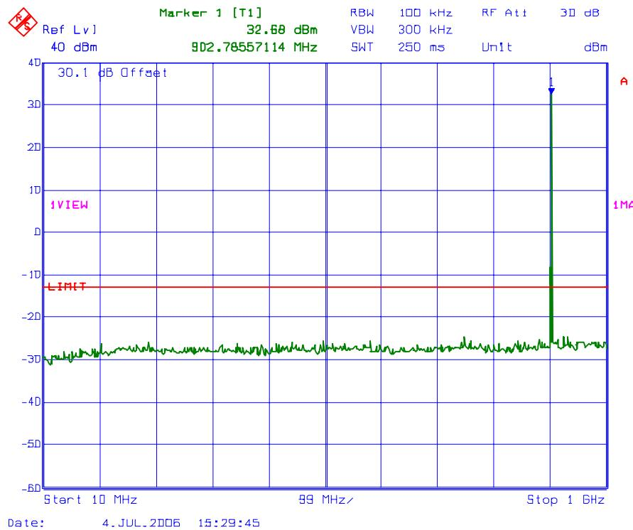
**PLOT # 90    Conducted Spurious Emissions with 3 RF signal inputs/outputs**
