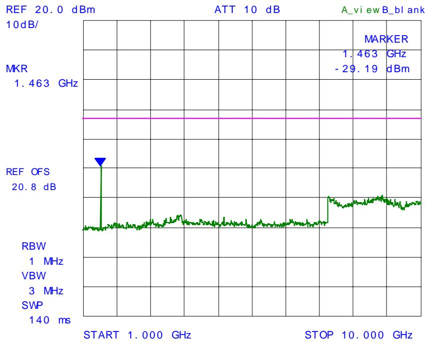
**PLOT # 61      Conducted Spurious Emissions with 1 RF signal input/output
