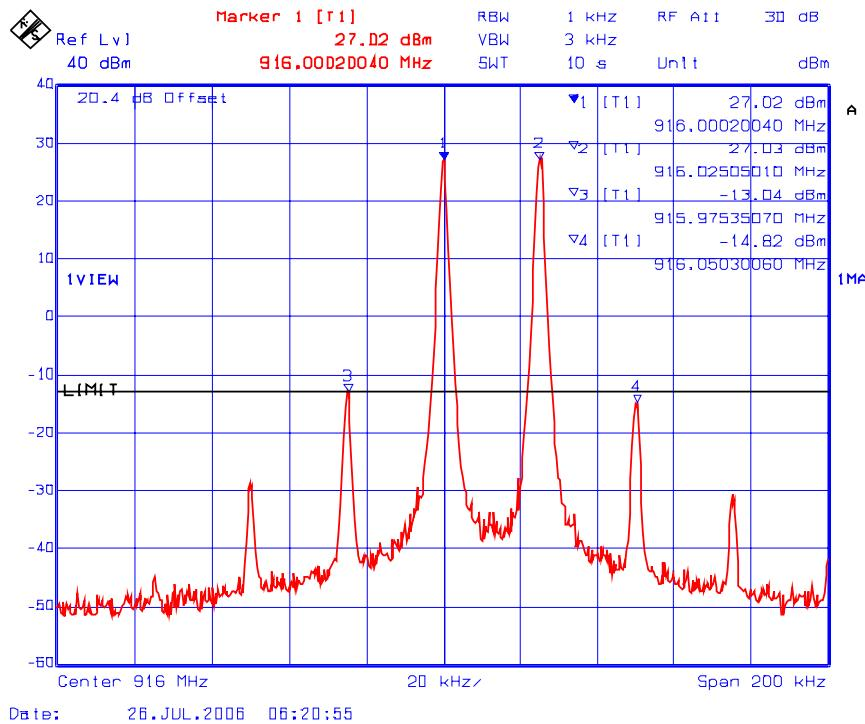
**PLOT #: 21** Intermodulation with 3 RF signal inputs/outputs
