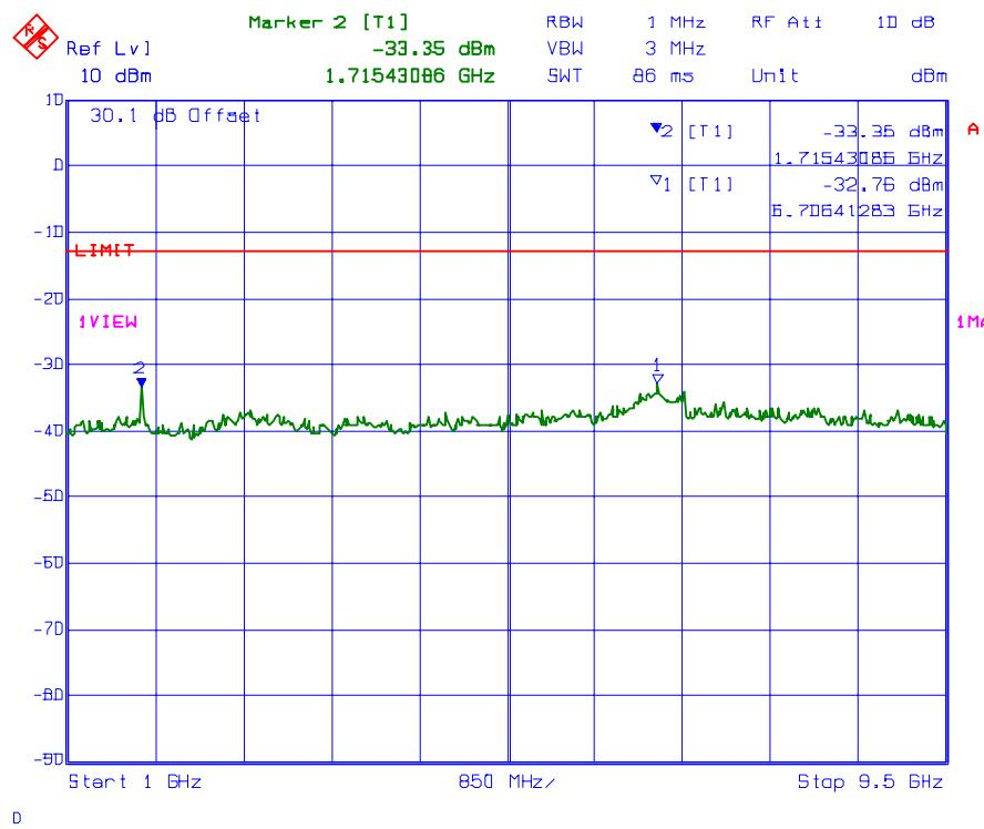
**PLOT # 69    Conducted Spurious Emissions with 2 RF signal inputs/outputs**
