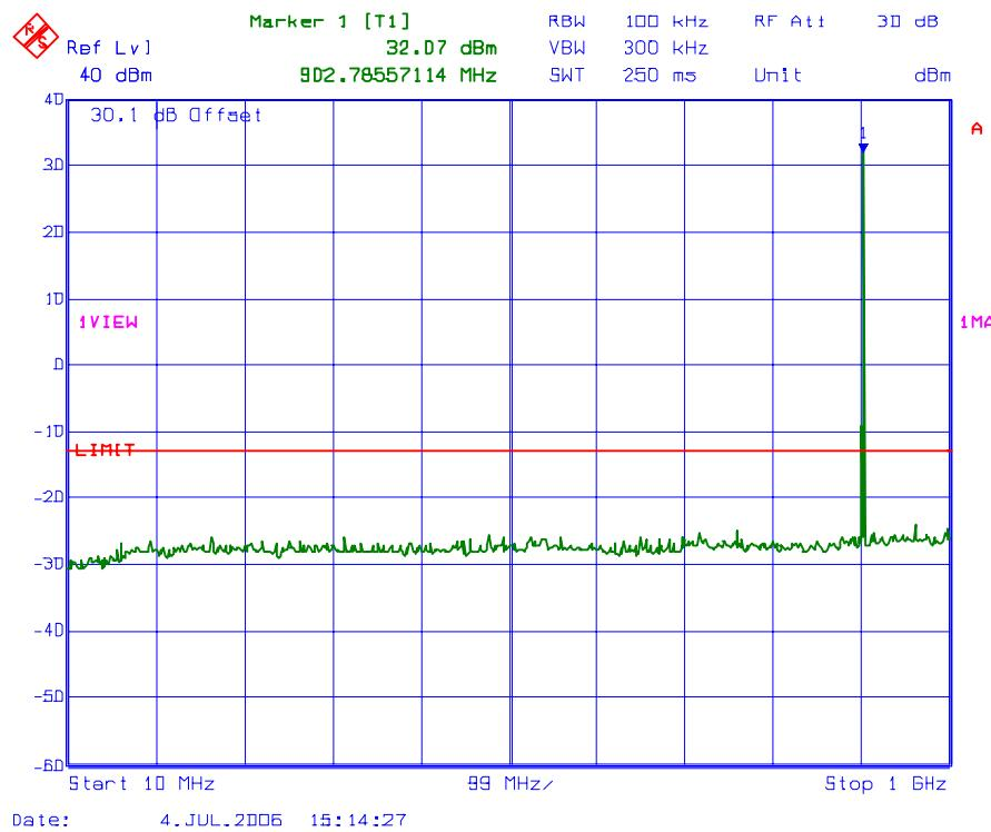
**PLOT # 88    Conducted Spurious Emissions with 2 RF signal inputs/outputs**
