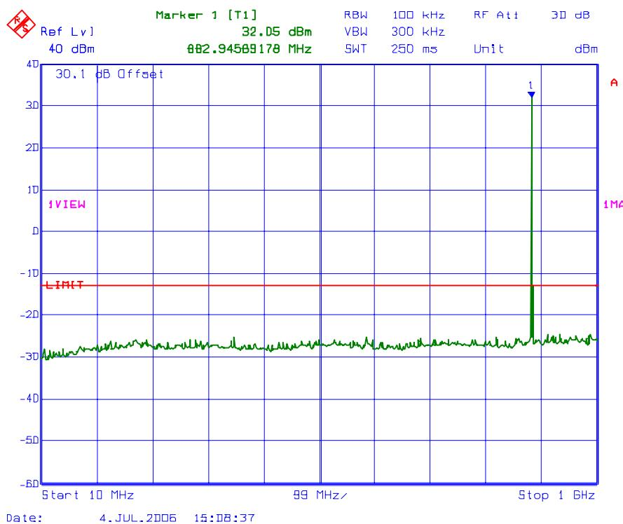
**PLOT # 76    Conducted Spurious Emissions with 2 RF signal inputs/outputs**
