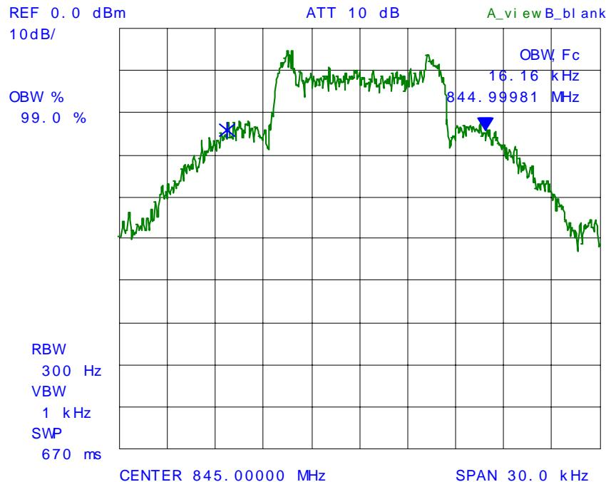
**PLOT # 46 99% Occupied Bandwidth – RF Output Signal**
