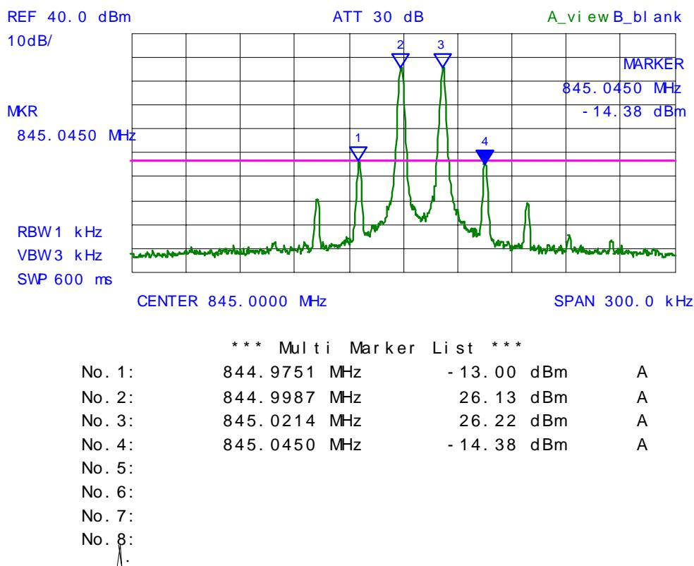
**PLOT #: 6** Intermodulation with 3 RF signal inputs/outputs
