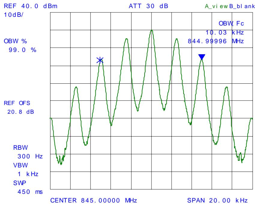
**PLOT # 41 99% Occupied Bandwidth – RF Input Signal**
