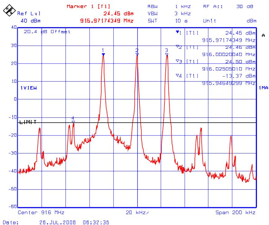
**PLOT #: 22 Intermodulation with 1 RF signal input/output**
