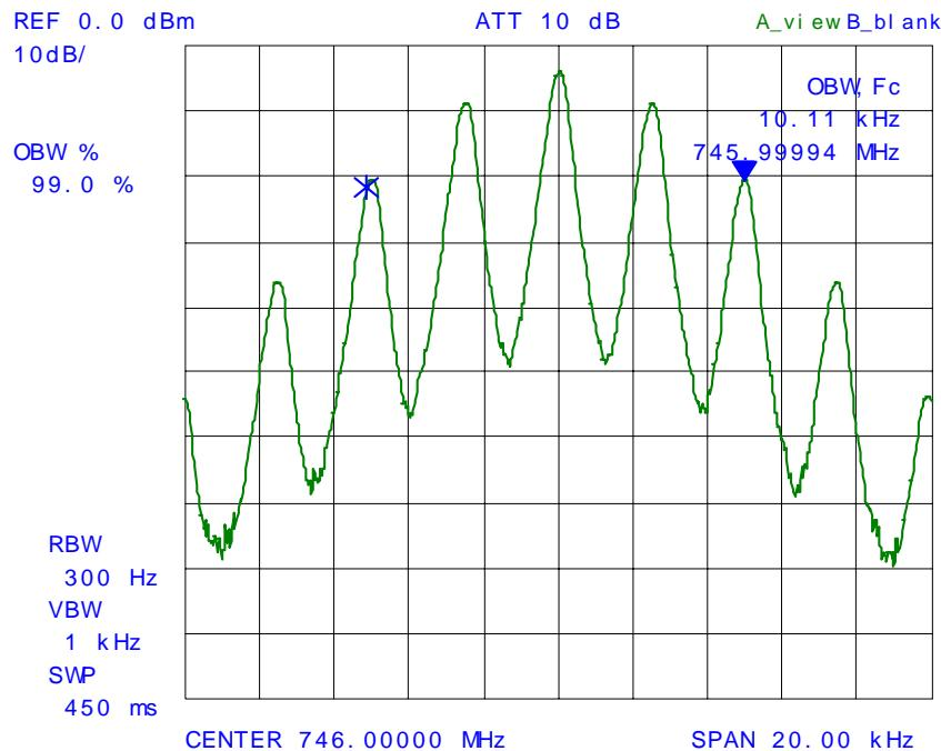
**PLOT # 32** 99% Occupied Bandwidth – RF Output Signal
