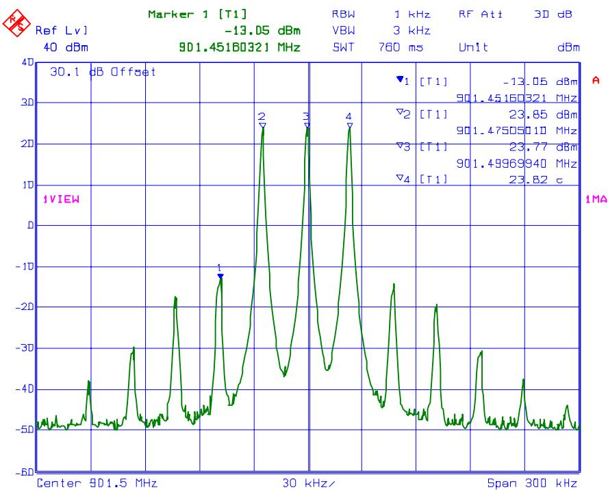
**PLOT#:** 19 **Intermodulation with 1 RF signal input/output**
