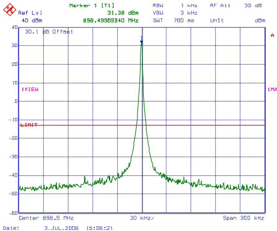
**PLOT#:** 14 **Intermodulation with 2 RF signal inputs/outputs**
