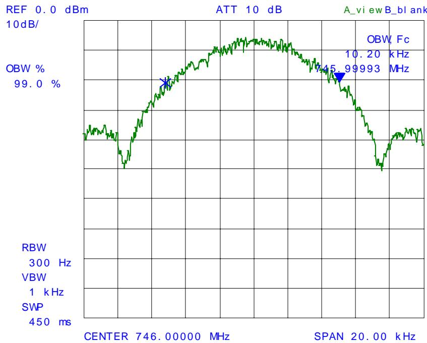
**PLOT # 36 99% Occupied Bandwidth – RF Output Signal**
