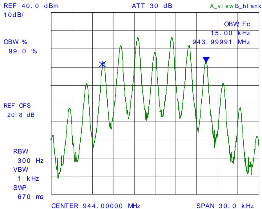
**PLOT # 51 99% Occupied Bandwidth – RF Input Signal**
