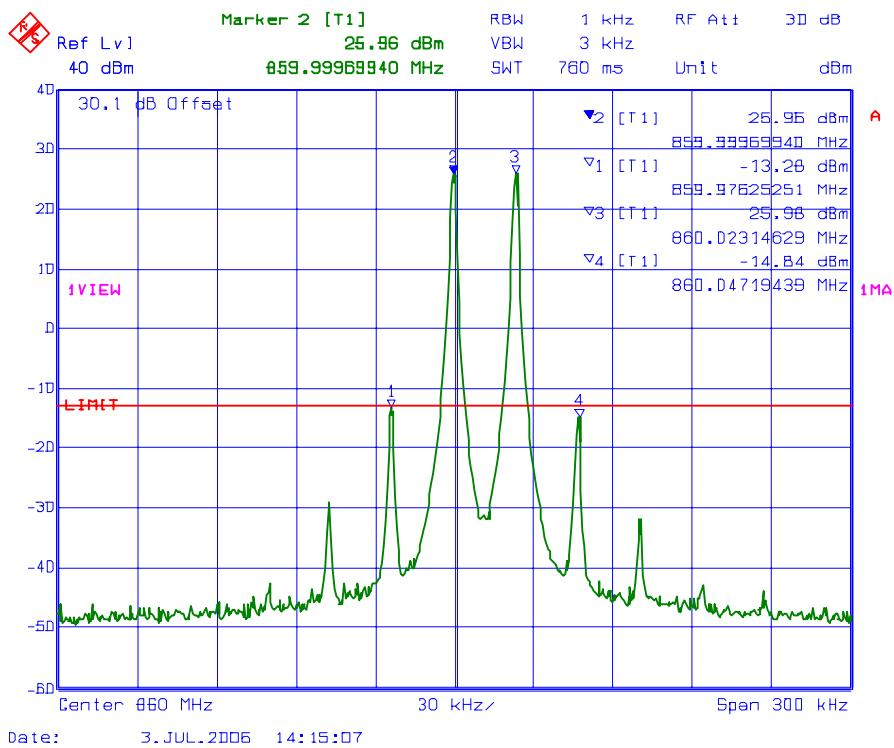
**PLOT #:** 9    **Intermodulation with 3 RF signal inputs/outputs**
