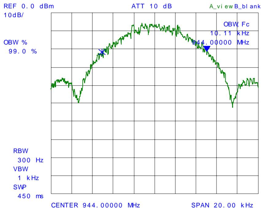
**PLOT # 52 99% Occupied Bandwidth – RF Output Signal**
