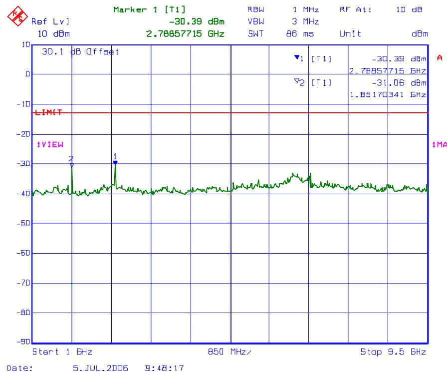
**PLOT # 101 Conducted Spurious Emissions with 3 RF signal inputs/outputs**
