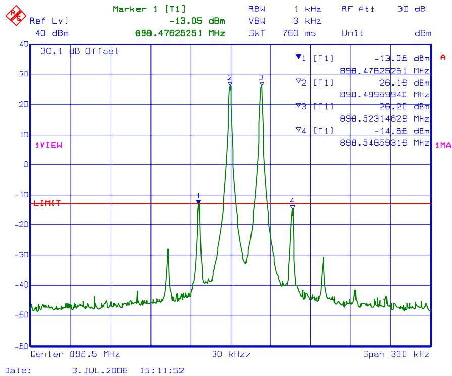
**PLOT #: 15 Intermodulation with 3 RF signal inputs/outputs**
