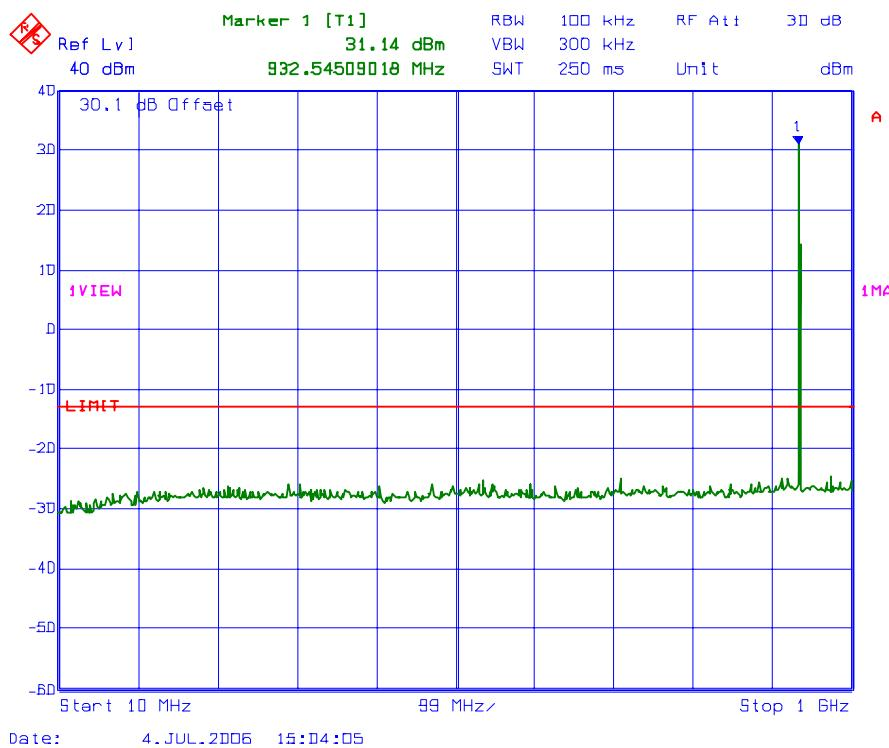
**PLOT # 98    Conducted Spurious Emissions with 1 RF signal input/output
