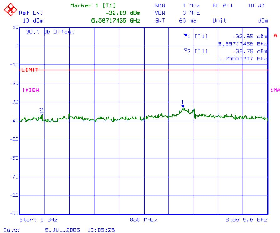
**PLOT # 77    Conducted Spurious Emissions with 3 RF signal inputs/outputs**
