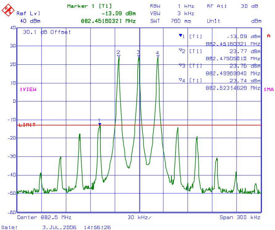
**PLOT#:** 13   **Intermodulation with 1 RF signal input/output**
