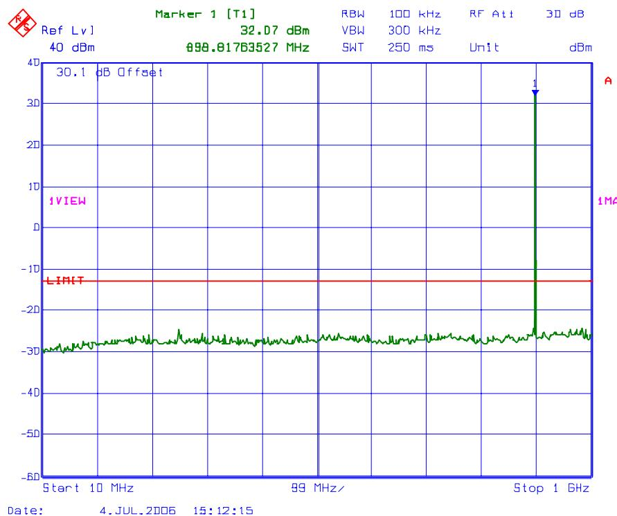
**PLOT # 82    Conducted Spurious Emissions with 2 RF signal inputs/outputs**
