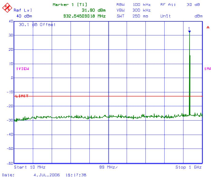
**PLOT # 100 Conducted Spurious Emissions with 2 RF signal inputs/outputs**
