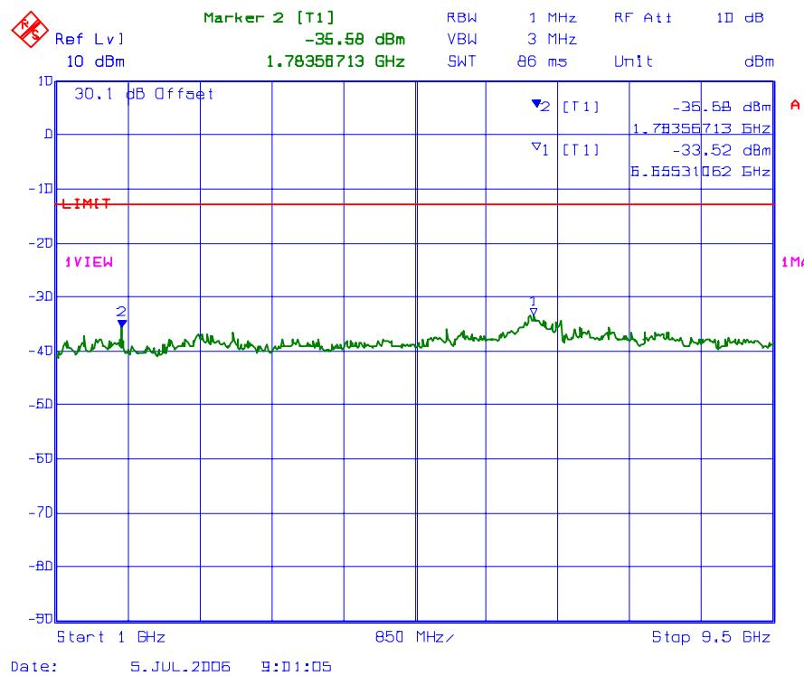
**PLOT # 81    Conducted Spurious Emissions with 2 RF signal inputs/outputs**
