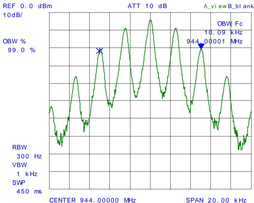
**PLOT # 48 99% Occupied Bandwidth – RF Output Signal**
