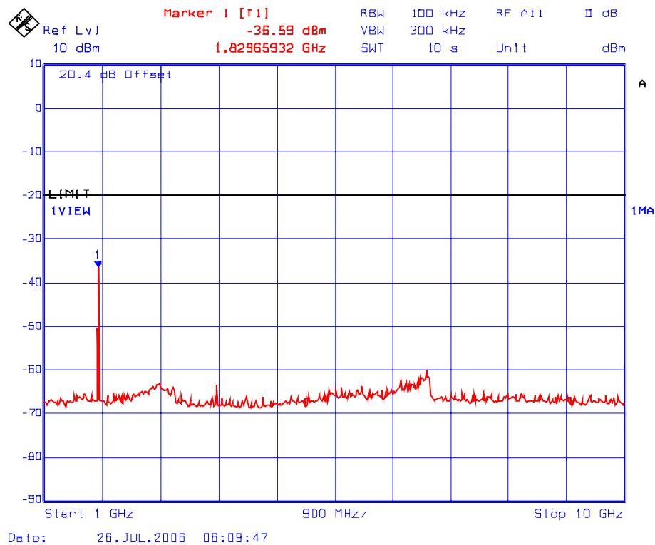
**PLOT # 93    Conducted Spurious Emissions with 2 RF signal inputs/outputs**
