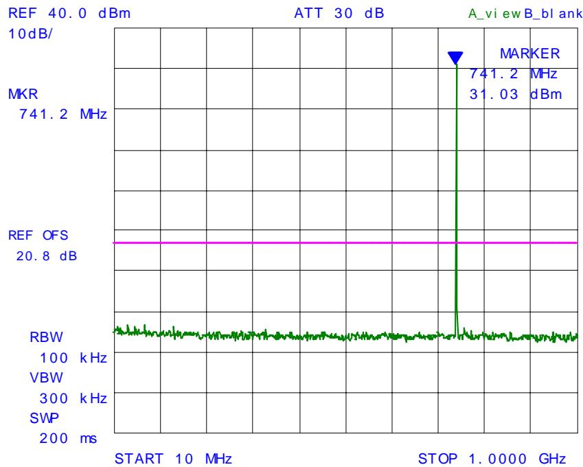
**PLOT # 58      Conducted Spurious Emissions with 2 RF signal inputs/outputs**
