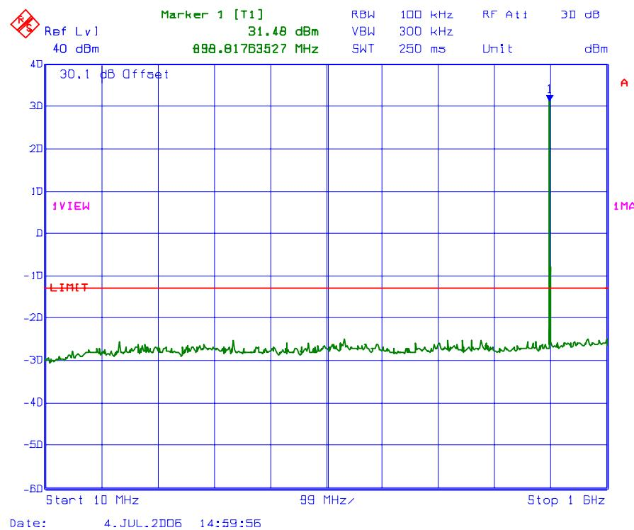
**PLOT # 80    Conducted Spurious Emissions with 1 RF signal input/output
