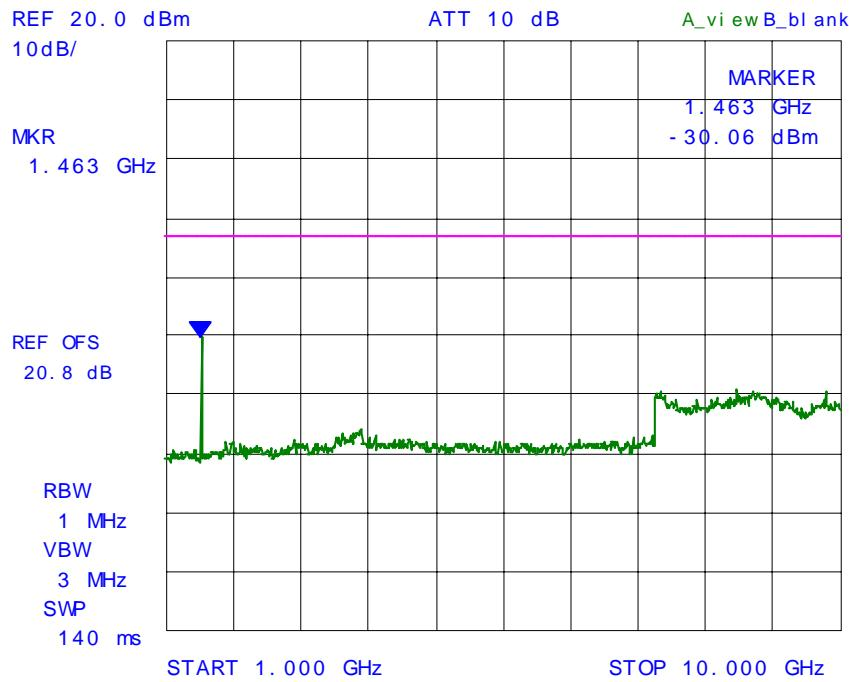
**PLOT # 59      Conducted Spurious Emissions with 3 RF signal inputs/outputs**
