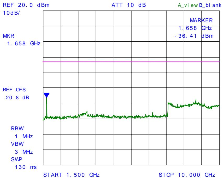
**PLOT # 67    Conducted Spurious Emissions with 1 RF signal input/output
