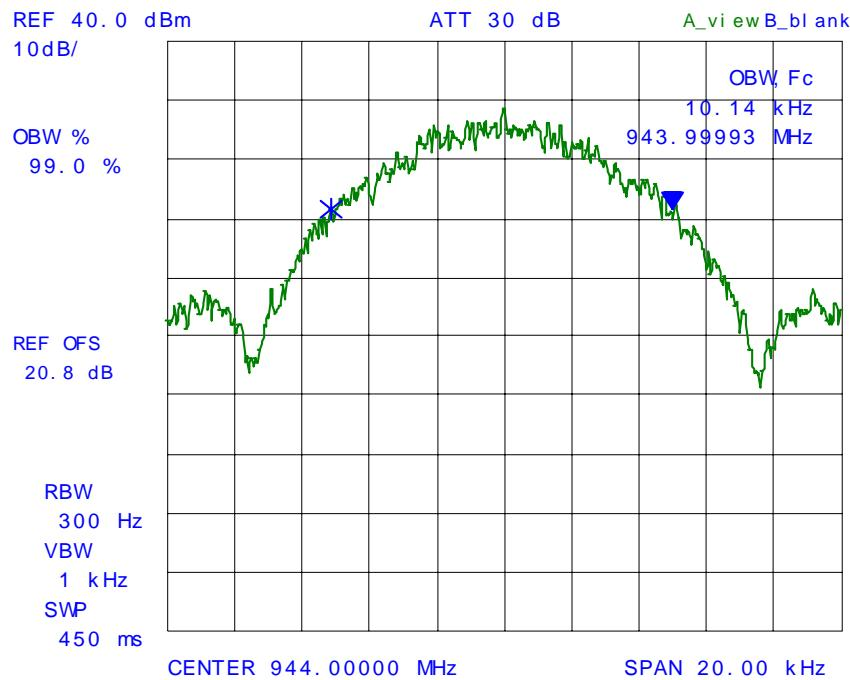
**PLOT # 53 99% Occupied Bandwidth – RF Input Signal**
