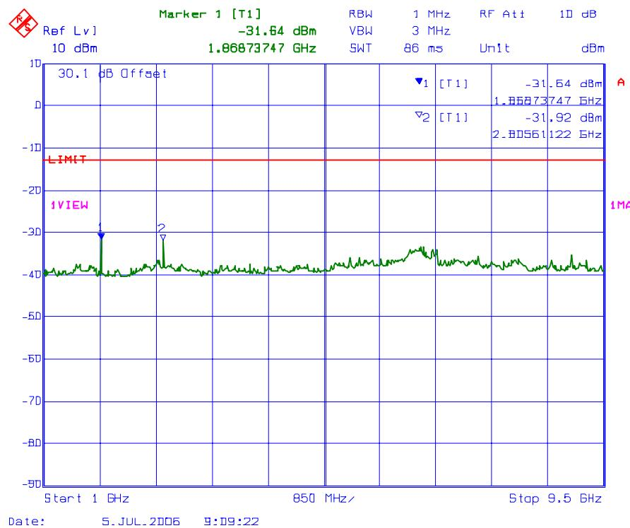
**PLOT # 105 Conducted Spurious Emissions with 2 RF signal inputs/outputs**
