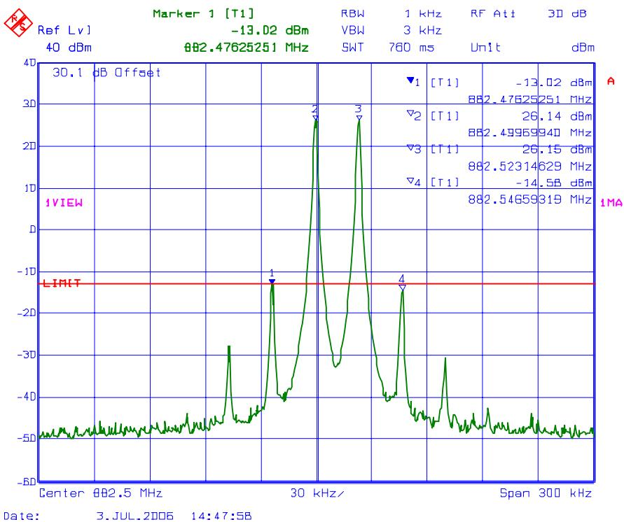
**PLOT #: 12** Intermodulation with 3 RF signal inputs/outputs
