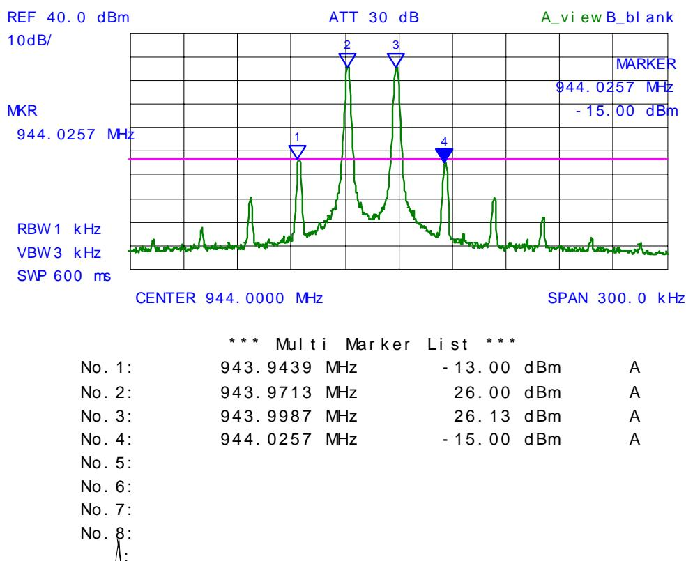
**PLOT #: 30 Intermodulation with 3 RF signal inputs/outputs**
