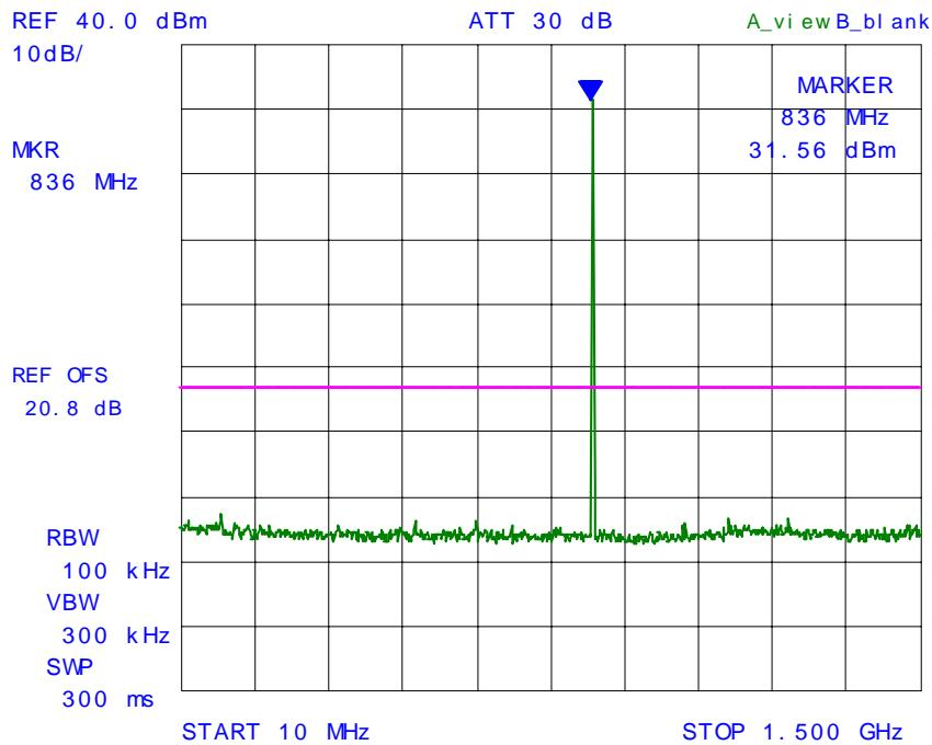
**PLOT # 64      Conducted Spurious Emissions with 2 RF signal inputs/outputs**
