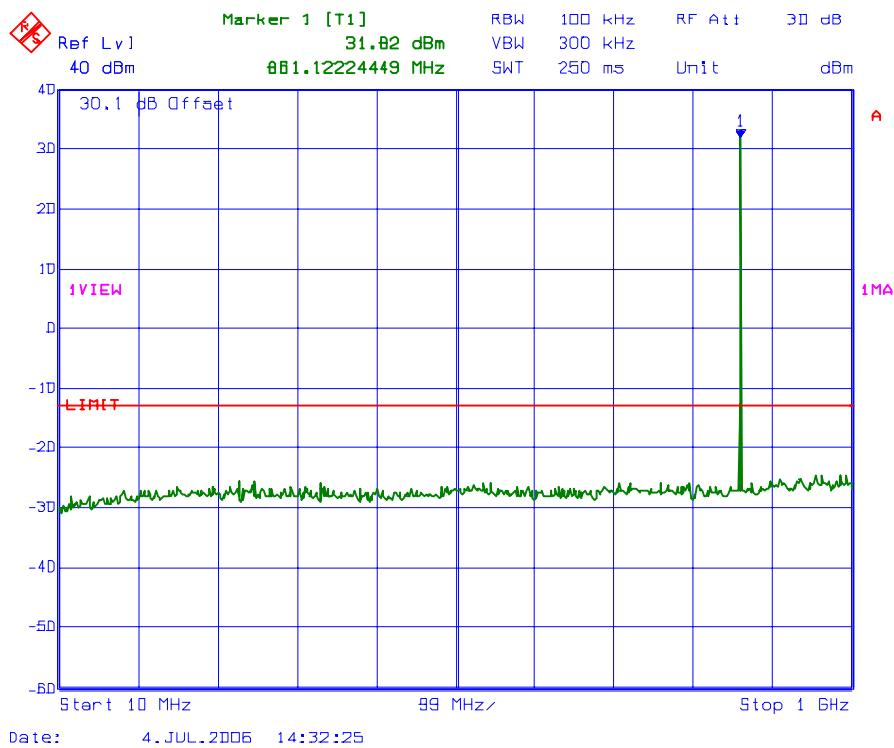
**PLOT # 70    Conducted Spurious Emissions with 2 RF signal inputs/outputs**
