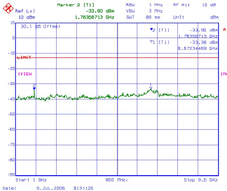
**PLOT # 83      Conducted Spurious Emissions with 3 RF signal inputs/outputs**
