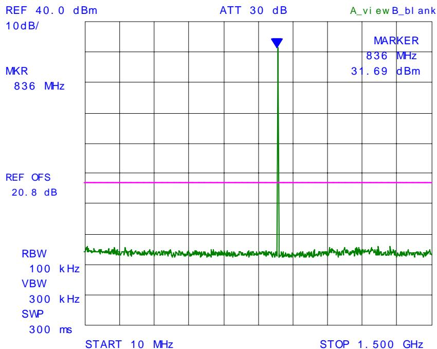
**PLOT # 66      Conducted Spurious Emissions with 3 RF signal inputs/outputs**
