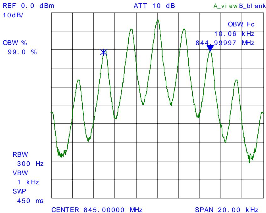
**PLOT # 40 99% Occupied Bandwidth – RF Output Signal**
