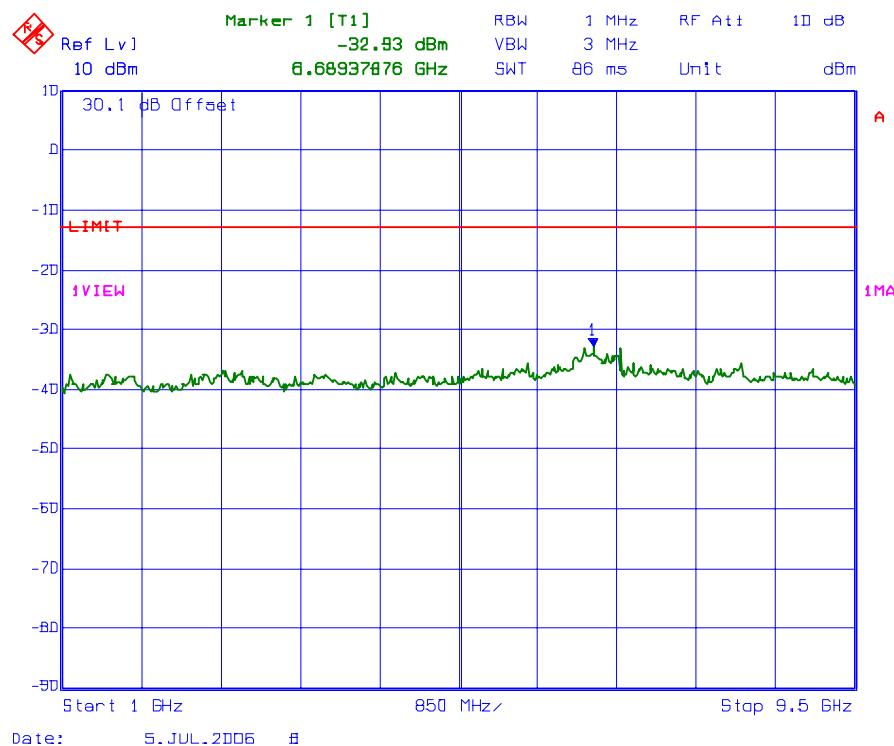
**PLOT # 75    Conducted Spurious Emissions with 2 RF signal inputs/outputs**
