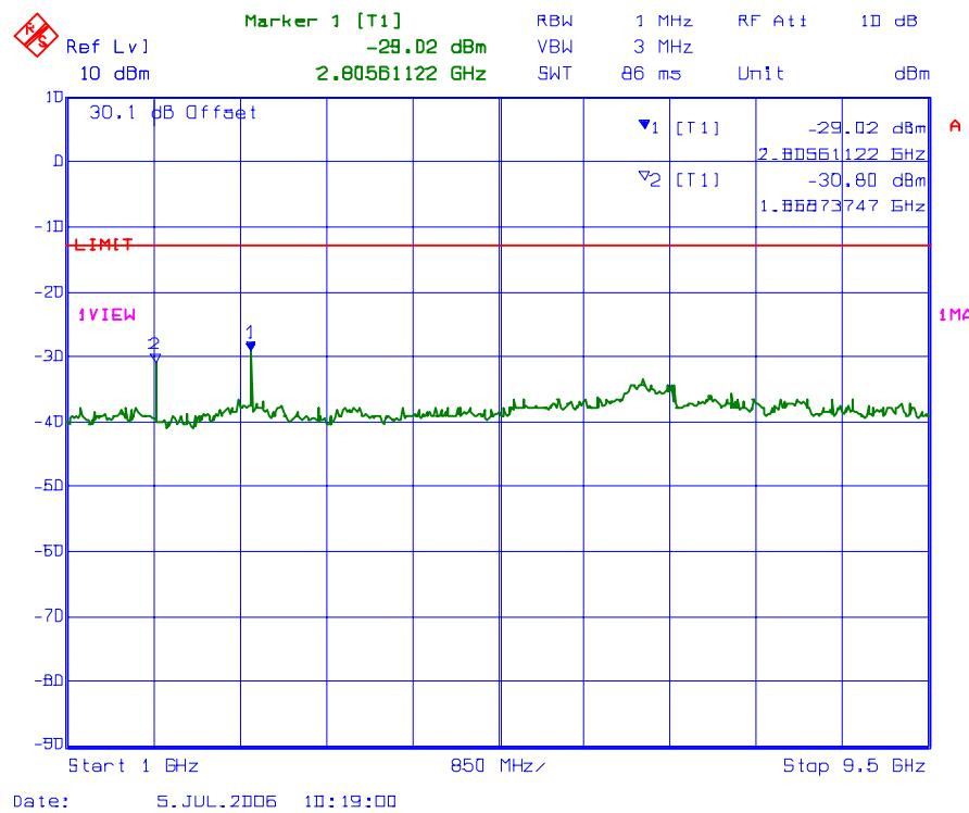
**PLOT # 109 Conducted Spurious Emissions with 1 RF signal input/output
