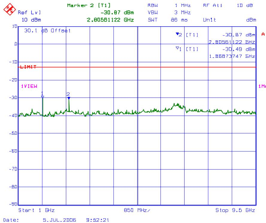
**PLOT # 107 Conducted Spurious Emissions with 3 RF signal inputs/outputs**
