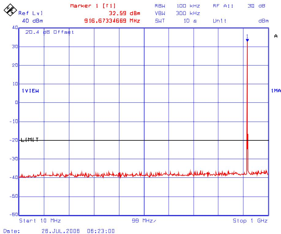
**PLOT # 94    Conducted Spurious Emissions with 2 RF signal inputs/outputs**
