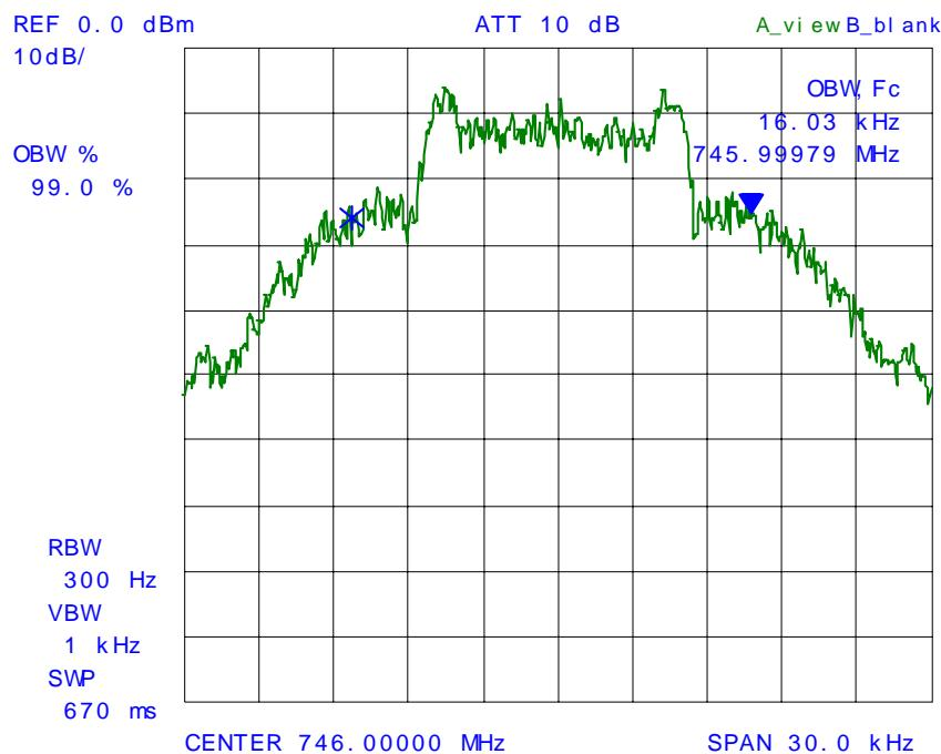
**PLOT # 38 99% Occupied Bandwidth – RF Output Signal**
