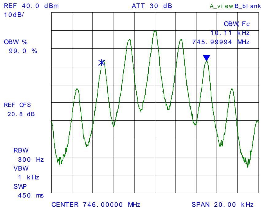
**PLOT # 33 99% Occupied Bandwidth – RF Input Signal**
