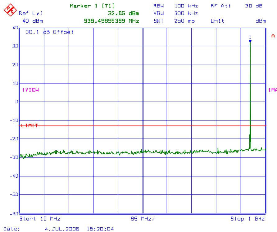
**PLOT # 106 Conducted Spurious Emissions with 2 RF signal inputs/outputs**
