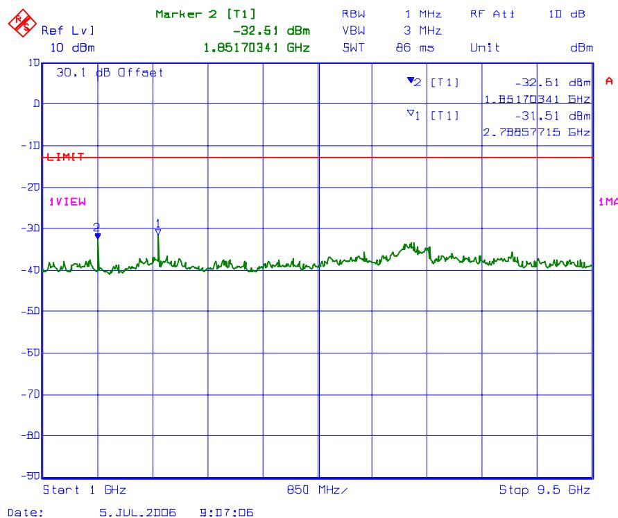
**PLOT # 99    Conducted Spurious Emissions with 2 RF signal inputs/outputs**
