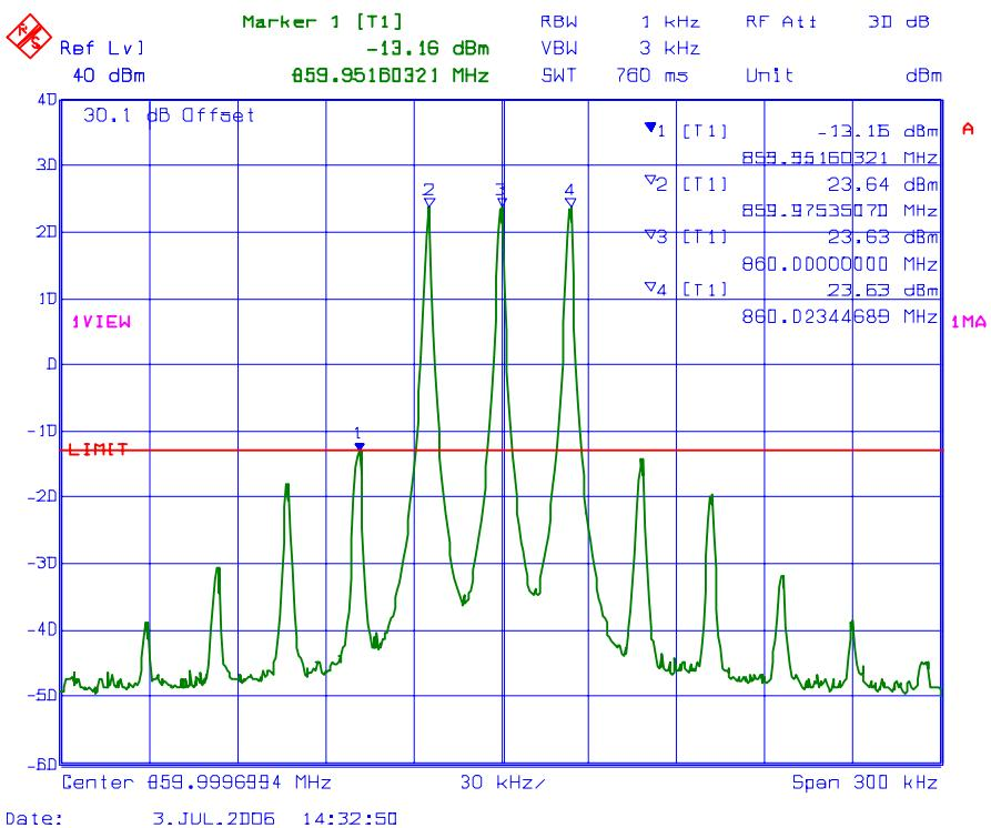
**PLOT #: 10 Intermodulation with 1 RF signal input/output**
