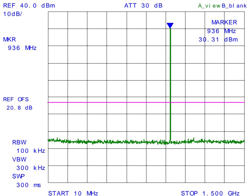
**PLOT # 110 Conducted Spurious Emissions with 1 RF signal input/output
