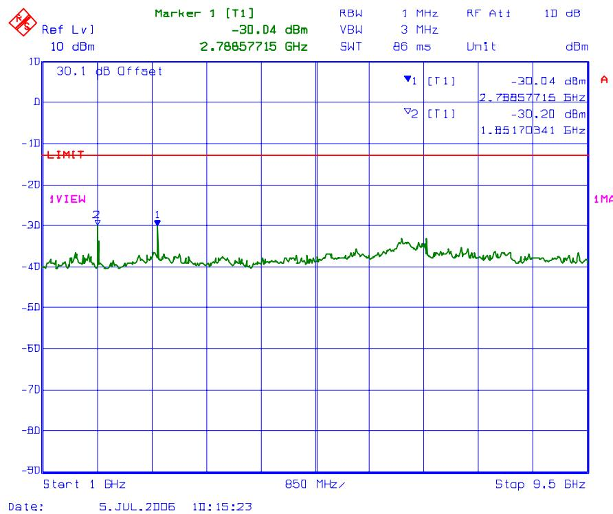
**PLOT # 103 Conducted Spurious Emissions with 1 RF signal input/output
