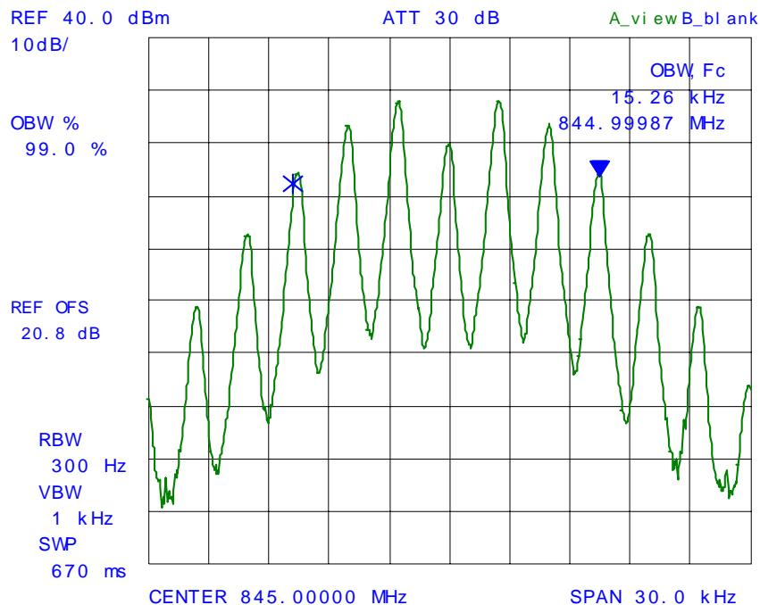
**PLOT # 43 99% Occupied Bandwidth – RF Input Signal**
