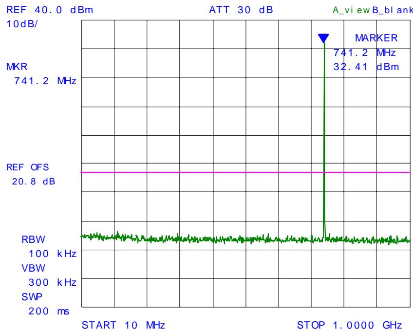
**PLOT # 56    Conducted Spurious Emissions with 1 RF signal input/output
