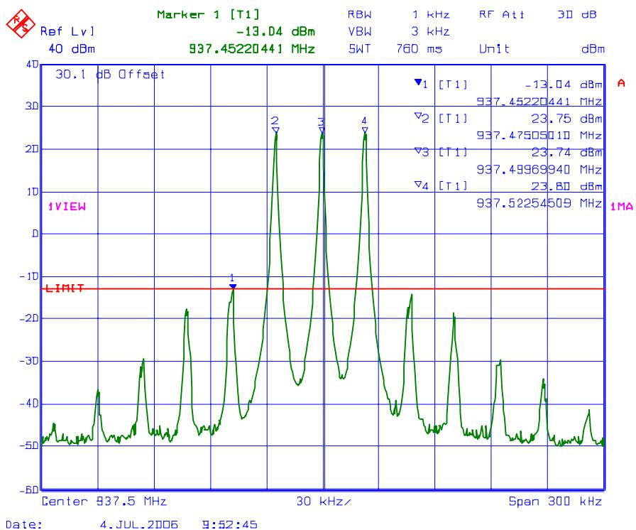
**PLOT #: 28 Intermodulation with 1 RF signal input/output**
