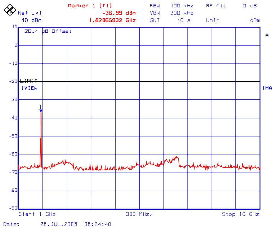
**PLOT # 95    Conducted Spurious Emissions with 3 RF signal inputs/outputs**
