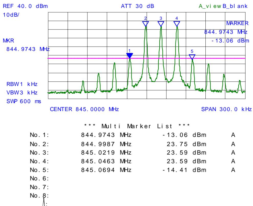
**PLOT#:** 7    **Intermodulation with 1 RF signal input/output**
