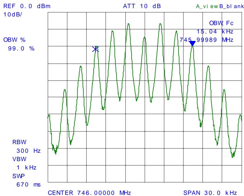
**PLOT # 34 99% Occupied Bandwidth – RF Output Signal**
