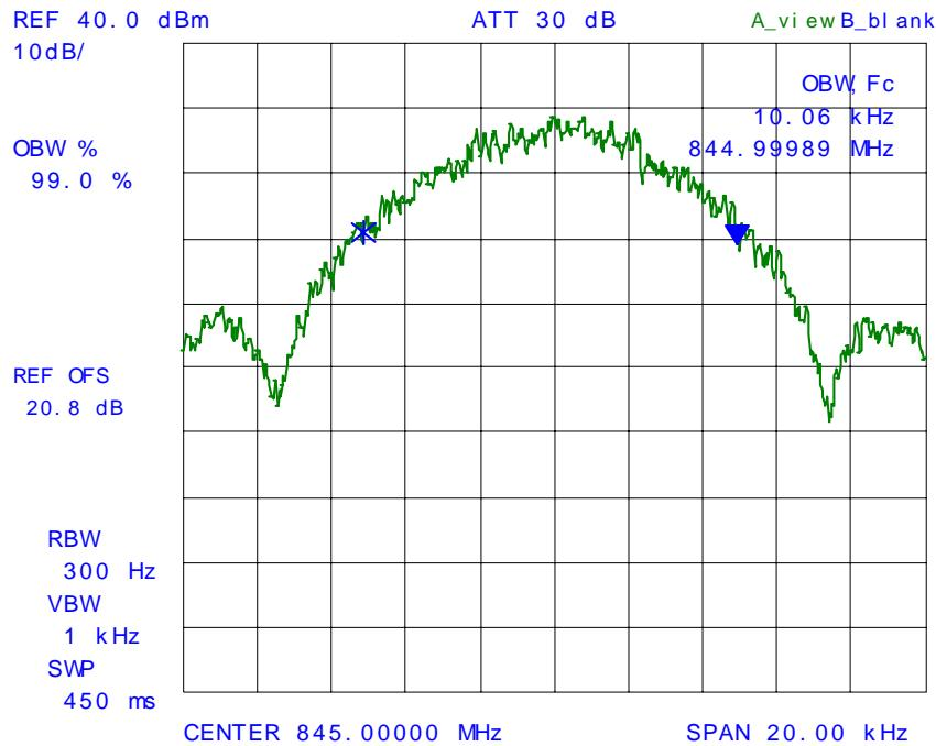
**PLOT # 45 99% Occupied Bandwidth – RF Input Signal**
