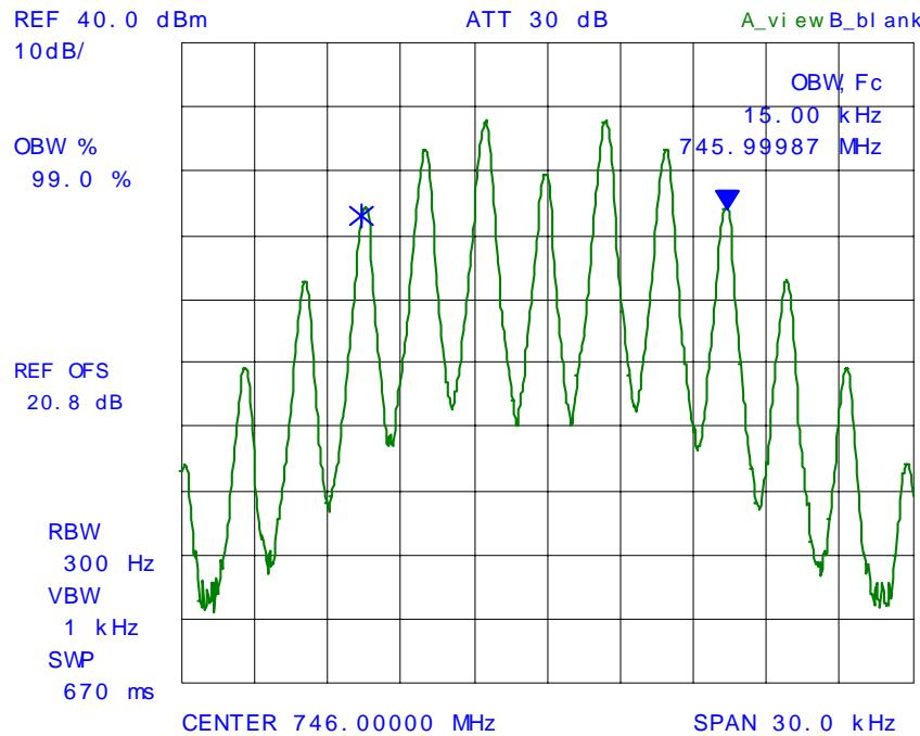
**PLOT # 35 99% Occupied Bandwidth – RF Input Signal**
