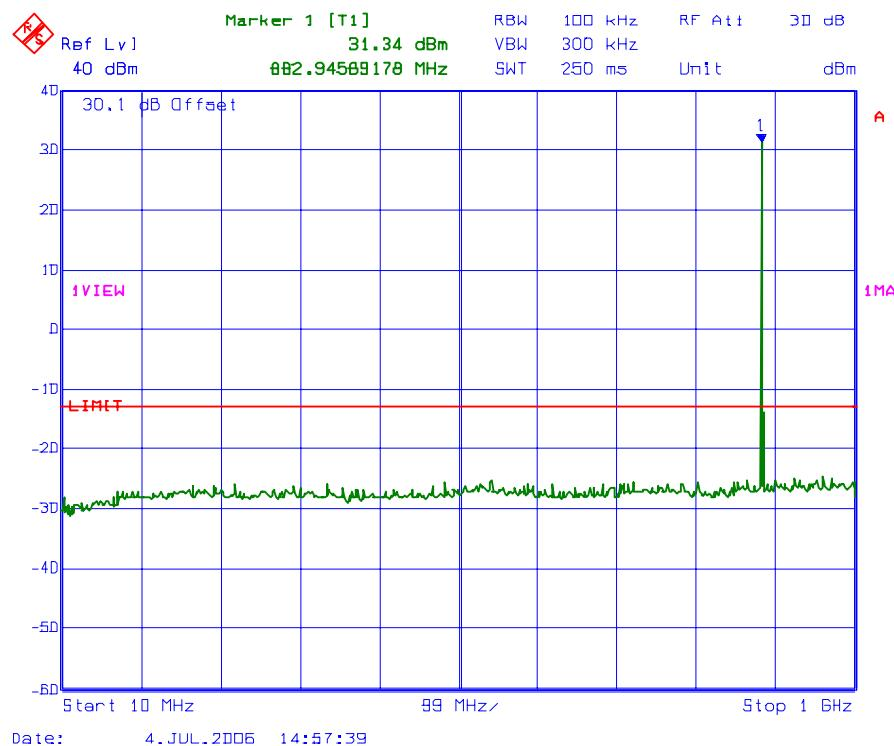
**PLOT # 74    Conducted Spurious Emissions with 1 RF signal input/output
