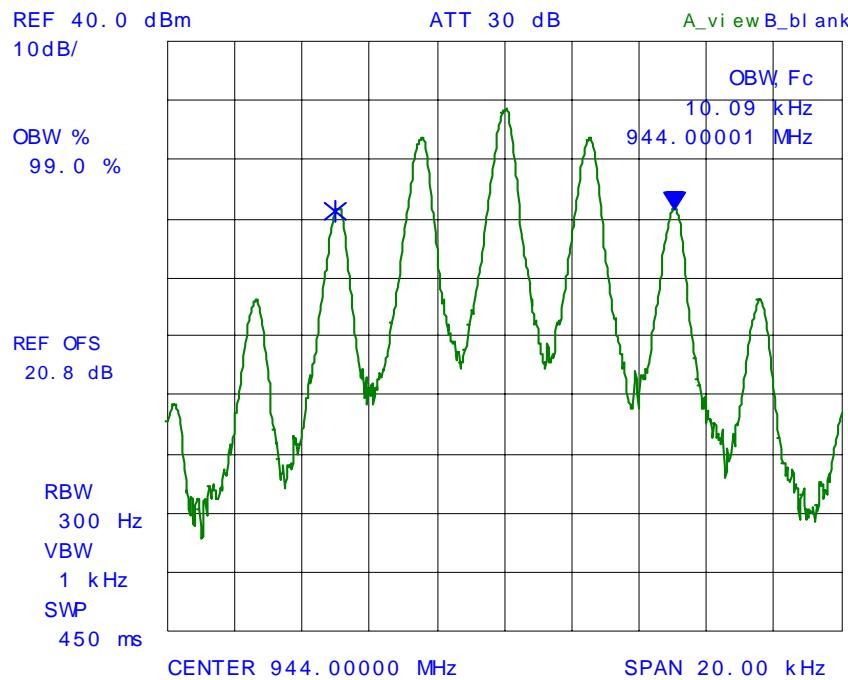
**PLOT # 49 99% Occupied Bandwidth – RF Input Signal**
