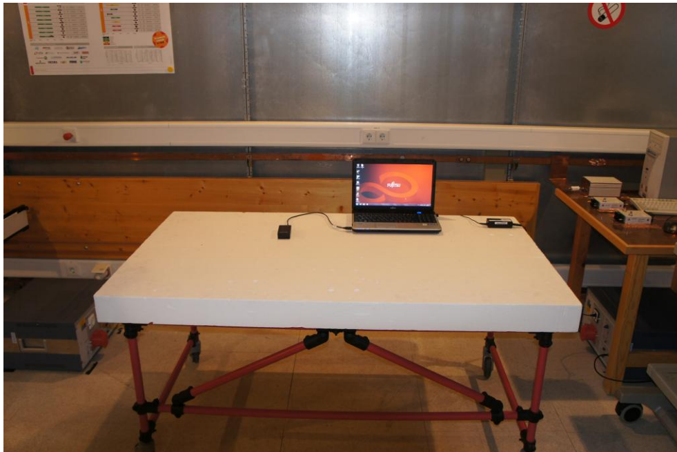
Picture 3: EUT test setup conducted emission test (front view)
