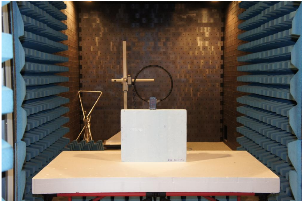
Picture 1: EUT test setup radiated emission test (9kHz to 30MHz)
