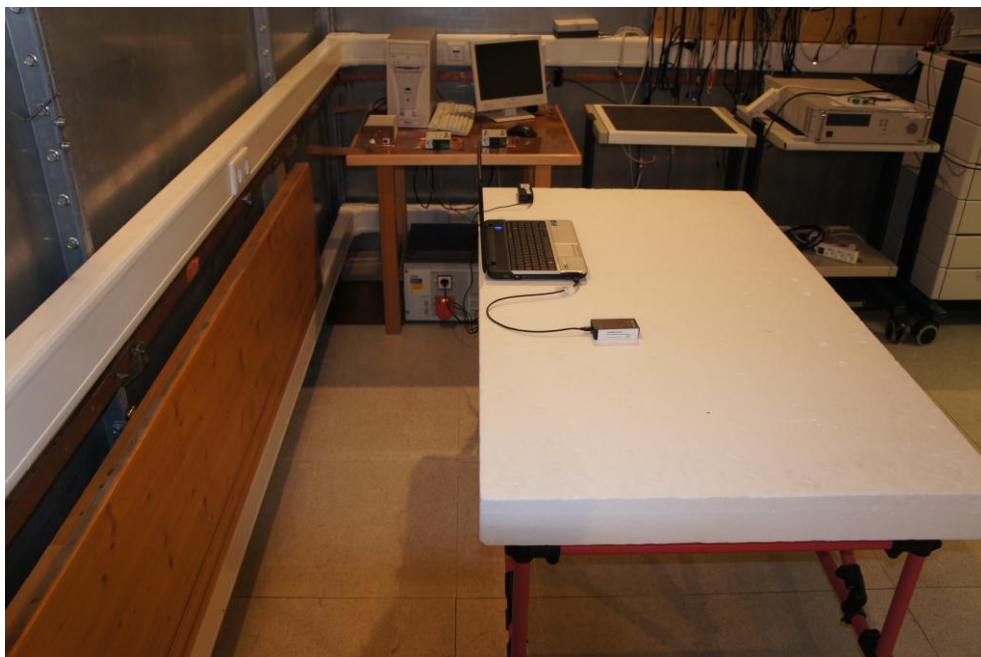
Picture 4: EUT test setup conducted emission test (side)
