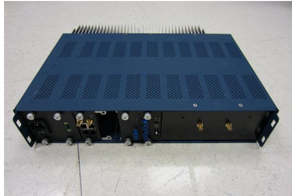
Figure 2: Master Station Chassis. The SDM9-1 modules may be installed in any free peripheral slot of this chassis.
