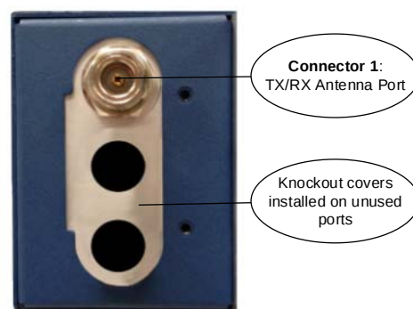
Figure 5: Internal Duplexer (or internal T/R switch), Single N connector
