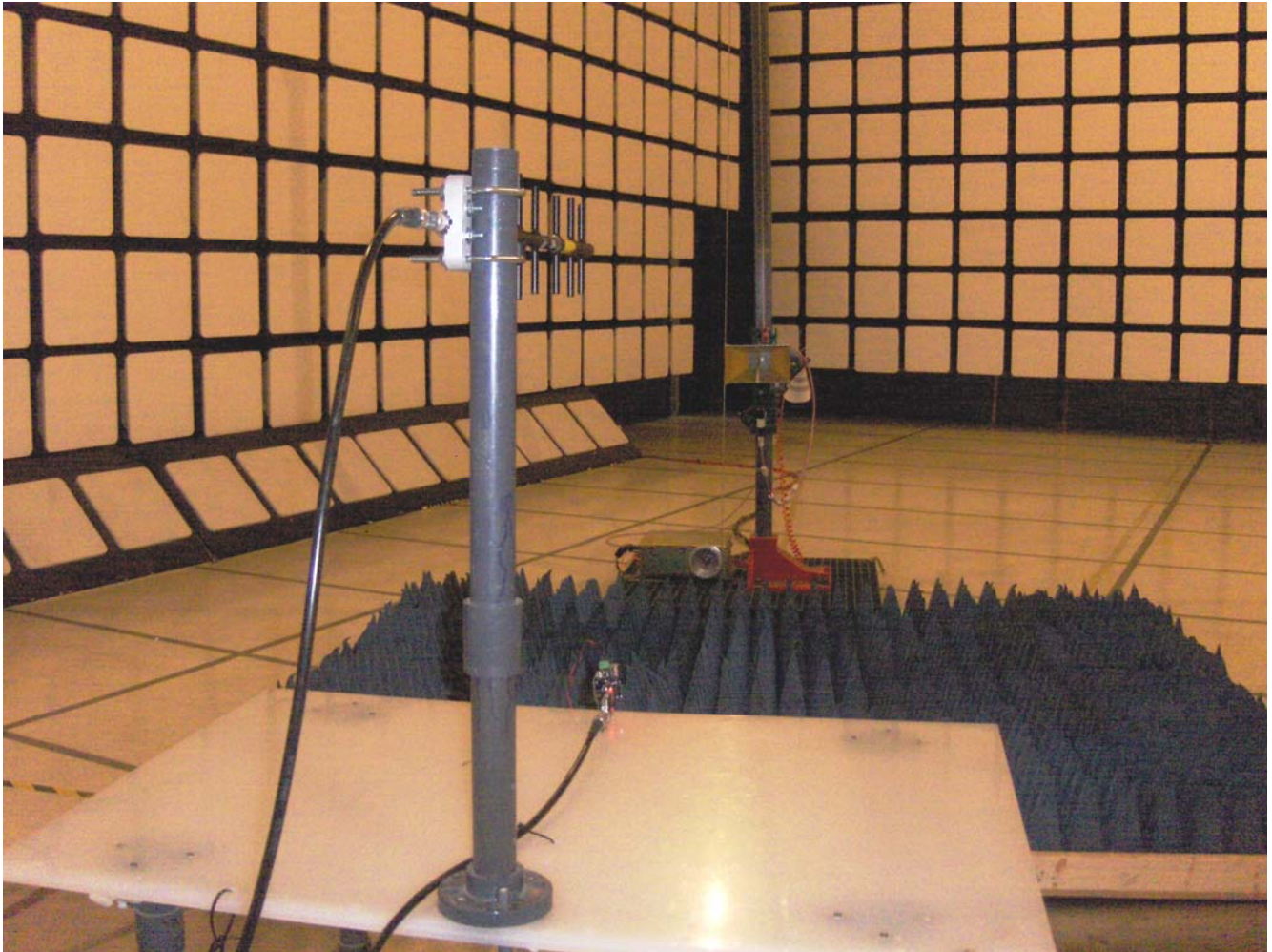
Radiated Emission Setup (Yagi Antenna)
