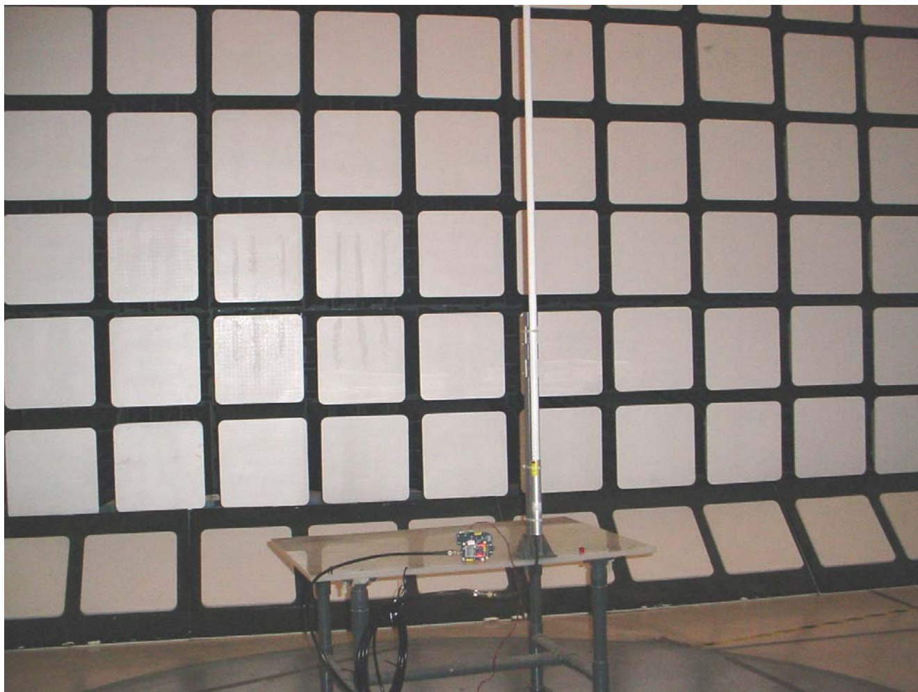
Radiated Emission Setup (Omni Antenna)
