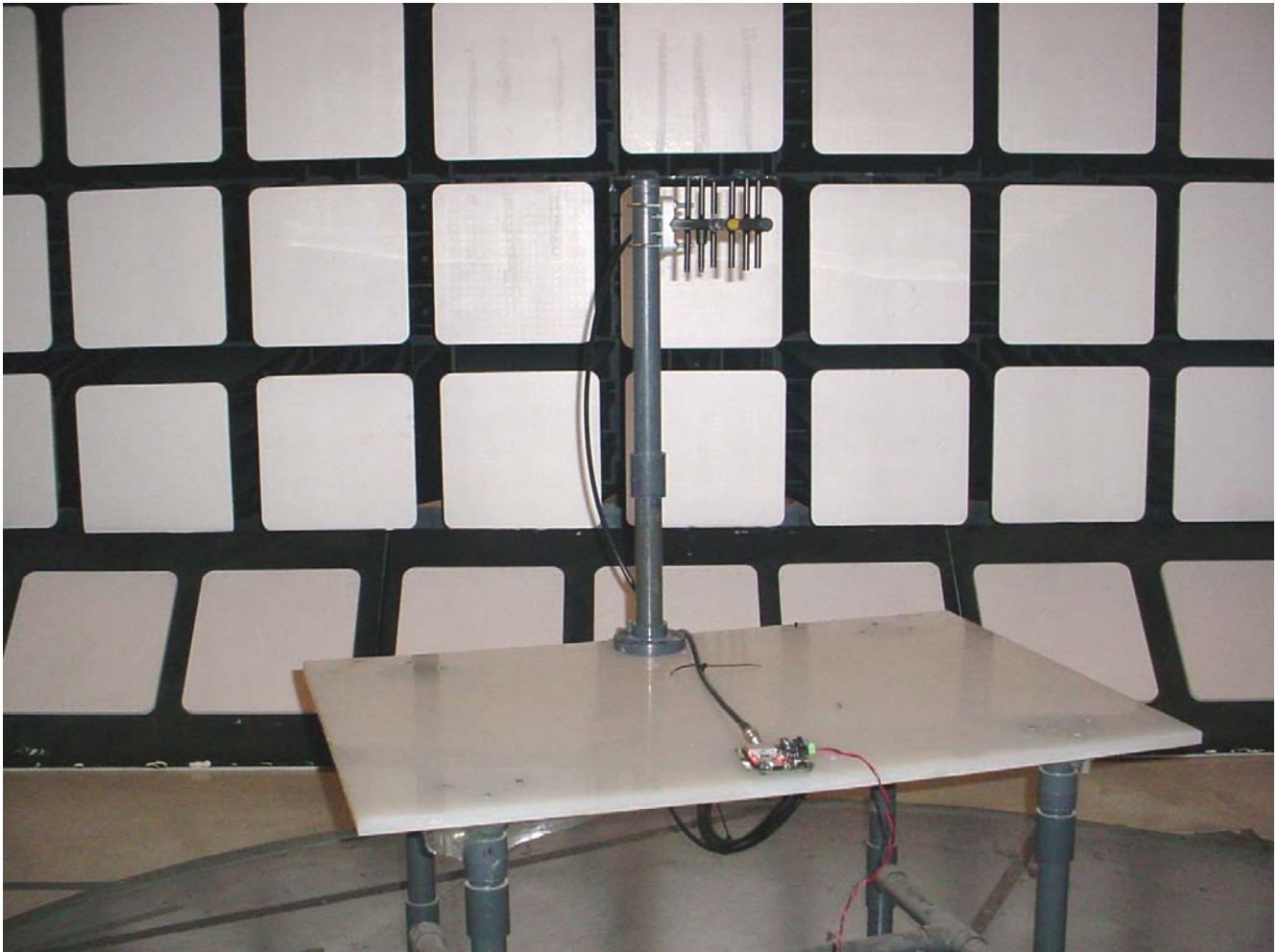
Radiated Emission Setup (Yagi Antenna)
