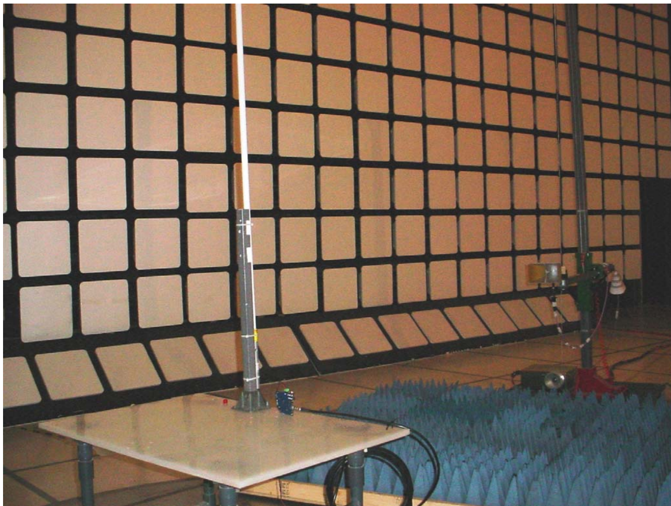
Radiated Emission Setup (Omni Antenna)
