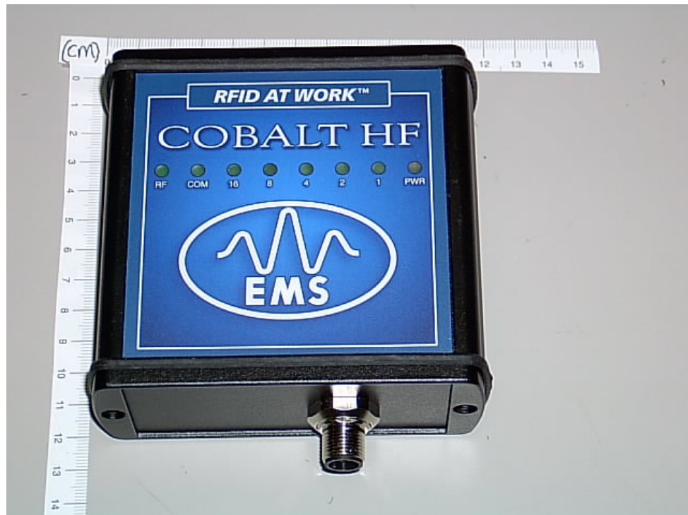
HF-CNTL-422-01 Enclosure Front/ Connectors
