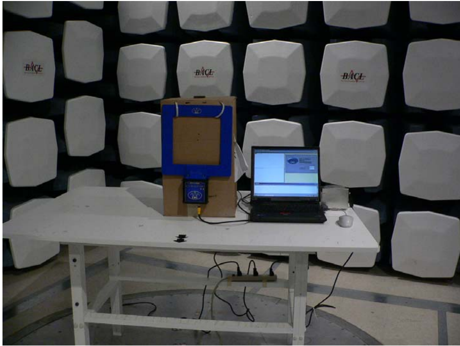
Radiated Emission Less than 30MHz – Front View
