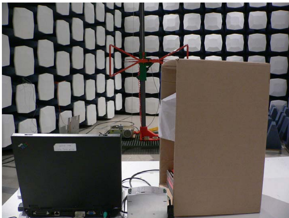
Radiated Emission Greater than 30MHz – Rear View
