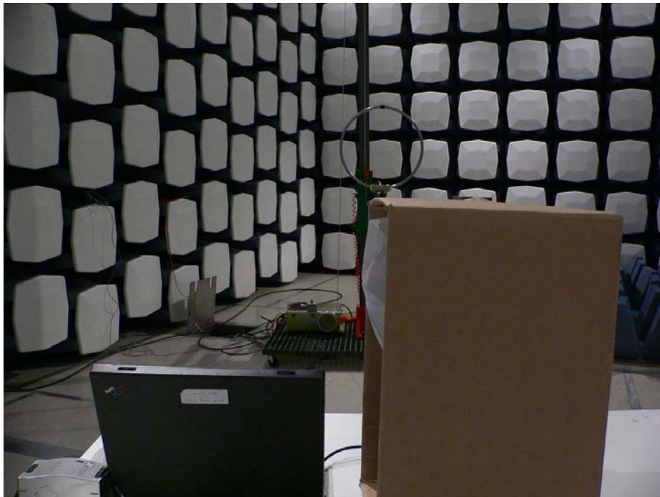
Radiated Emission Less than 30MHz – Rear View
