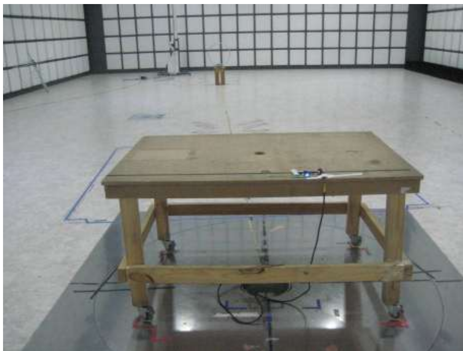
Figure 1. Photo of Radiated Emission Test Setup
