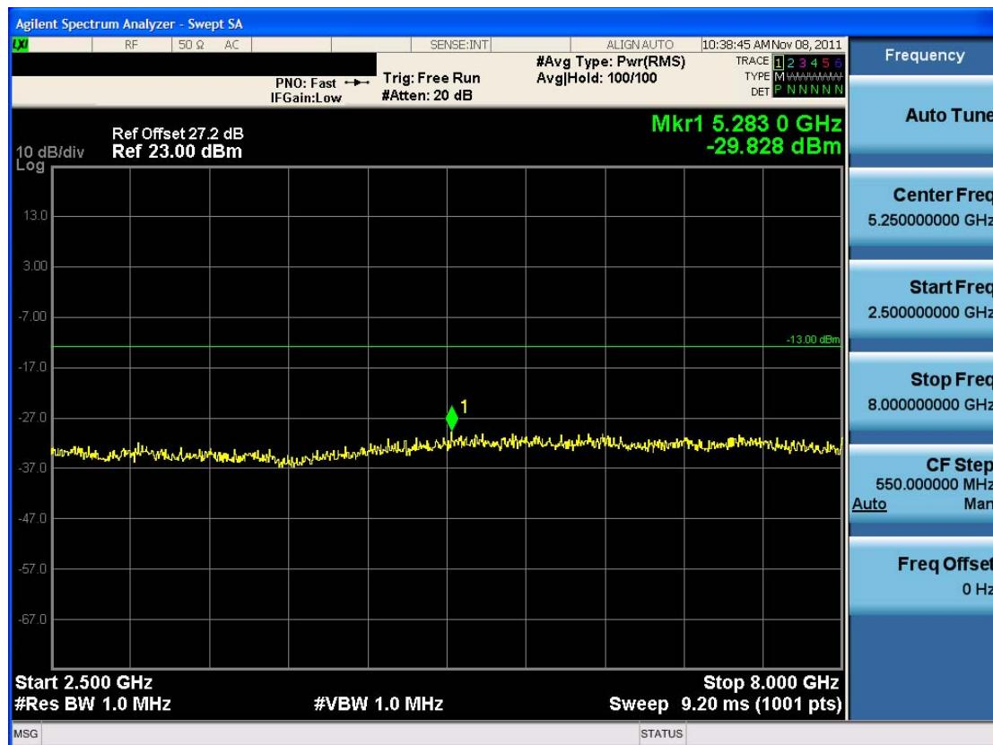
■ Conducted Spurious Emission (16-QAM – RB Size 1, RB Offset 0)-1
