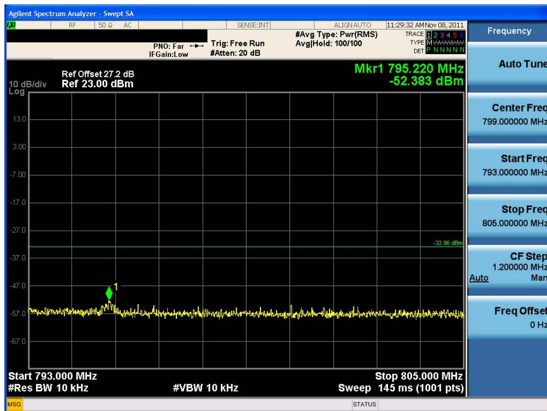
■ Upper Emission Mask (793 MHz – 805 MHz) 16-QAM –RB Size 50
