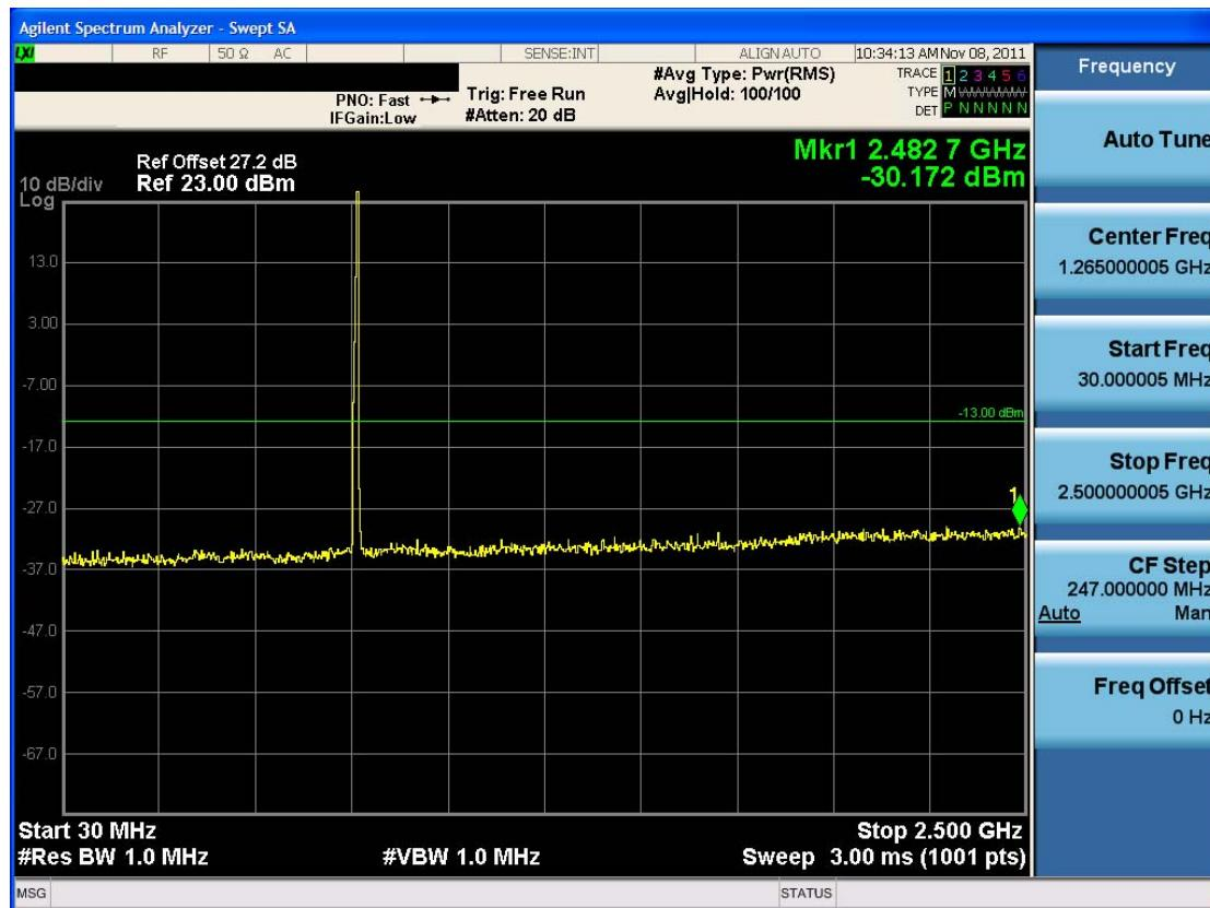
■ Conducted Spurious Emission (16-QAM – RB Size 1, RB Offset 49)-2
