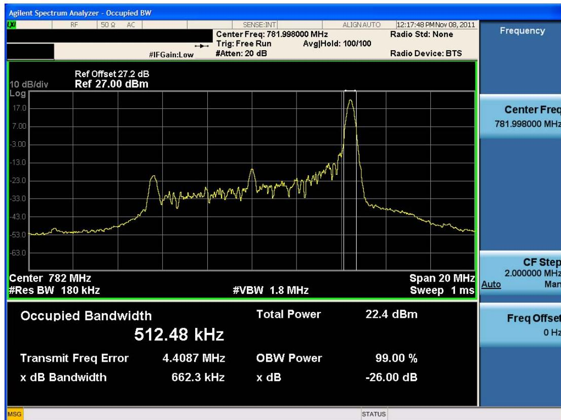
■ Occupied Bandwidth (16-QAM – RB Size 25, RB Offset 12)
