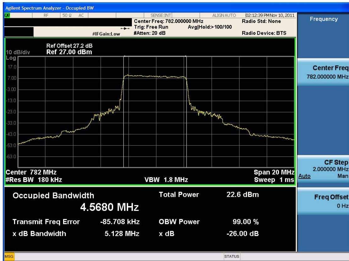
■ Occupied Bandwidth (QPSK – RB Size 50)
