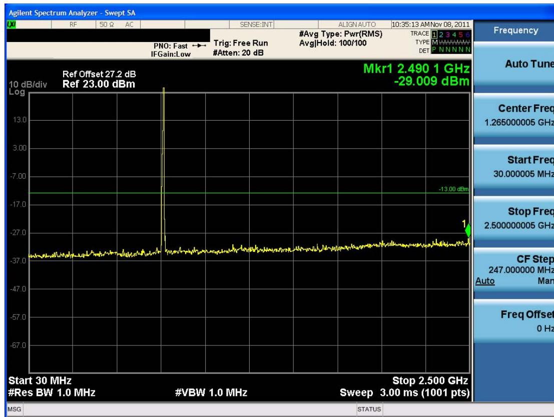
■ Conducted Spurious Emission (QPSK – RB Size 1, RB Offset 49)-2
