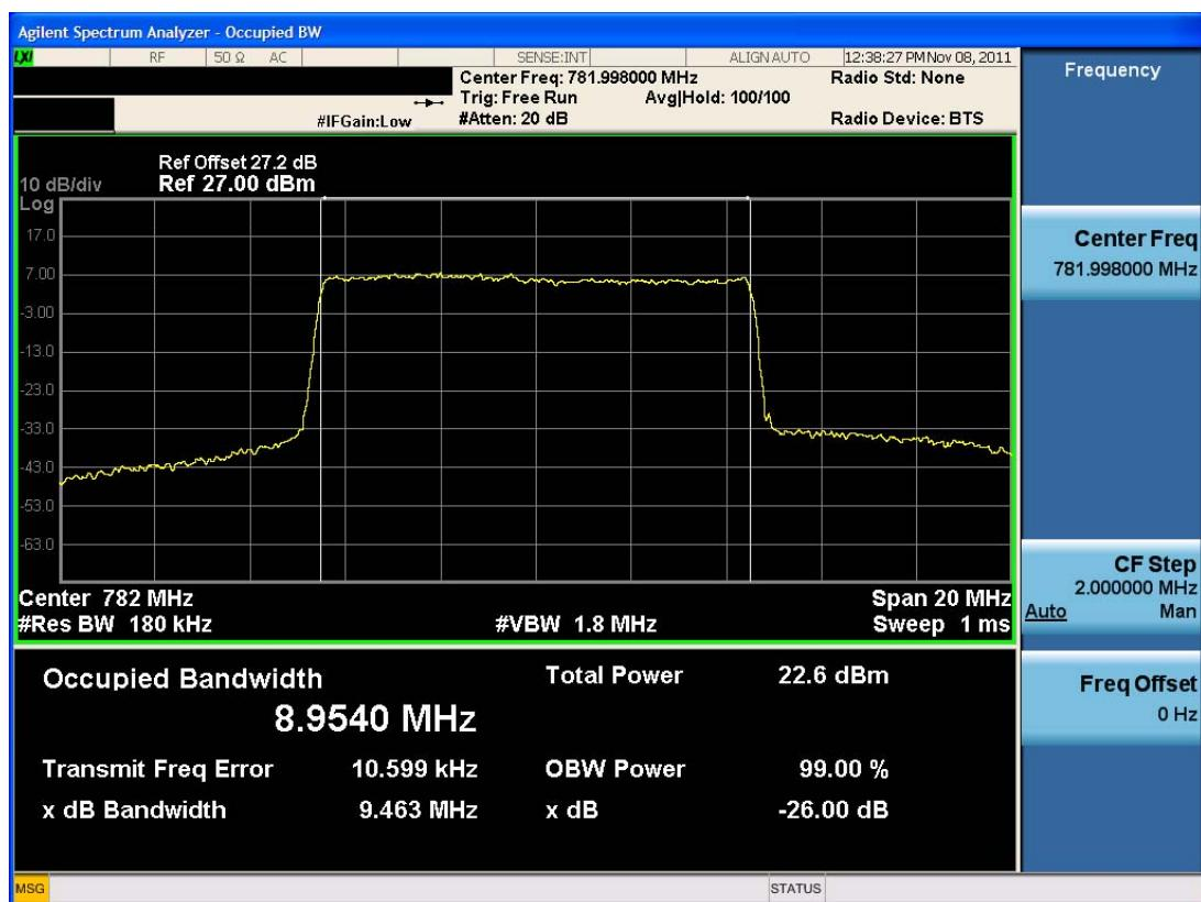
■ Occupied Bandwidth (16-QAM – RB Size 1, RB Offset 0)
