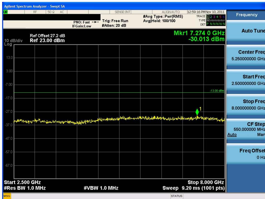
■ Conducted Spurious Emission (16-QAM – RB Size 50)-1
