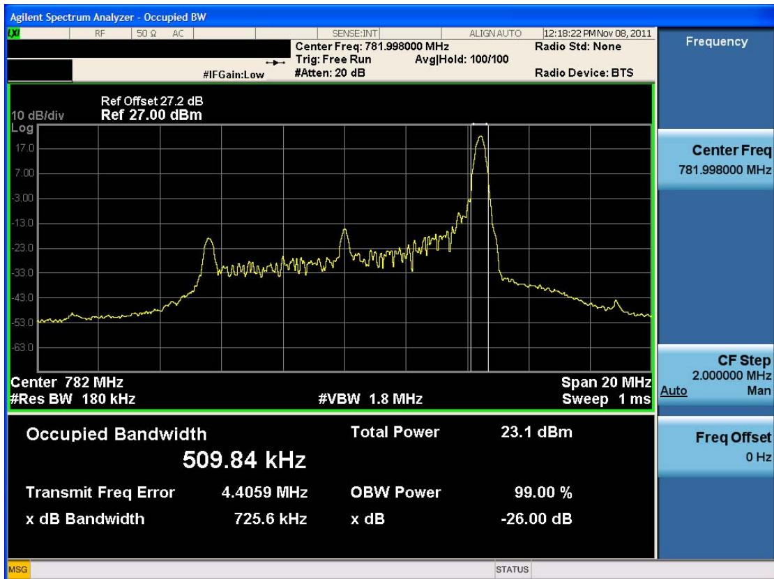
■ Occupied Bandwidth (QPSK – RB Size 25, RB Offset 12)
