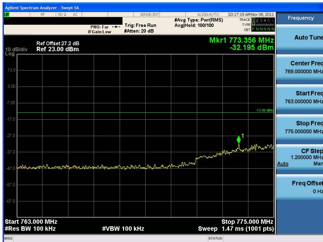
■ Upper Emission Mask (793 MHz – 805 MHz) 16-QAM – RB Size 1, RB Offset 49
