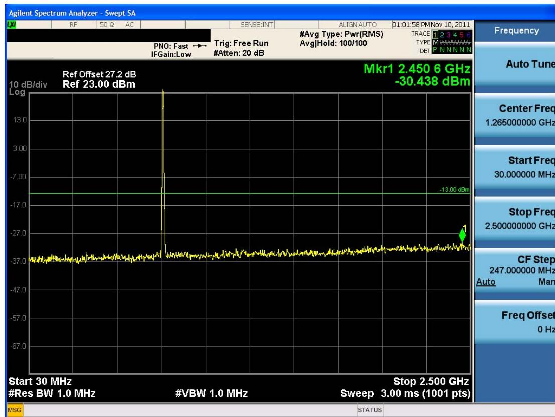
■ Conducted Spurious Emission (16-QAM – RB Size 25, RB Offset 12)-2
