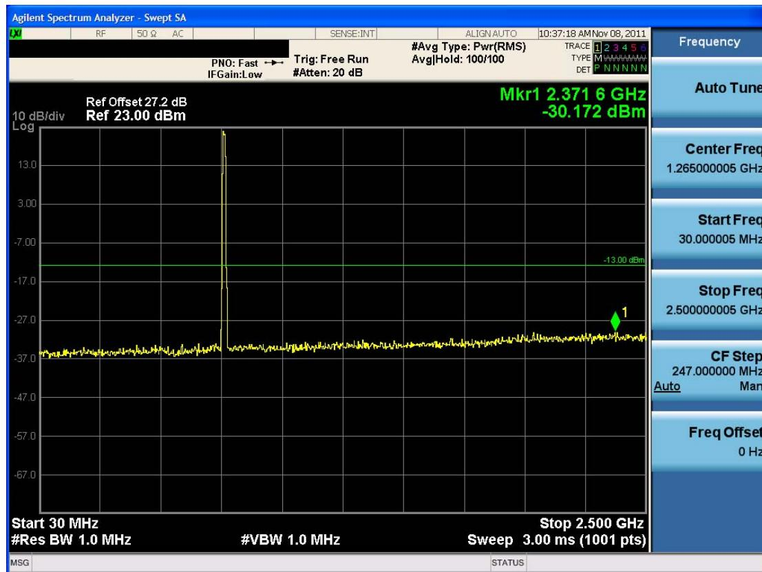
■ Conducted Spurious Emission (QPSK – RB Size 50)-2
