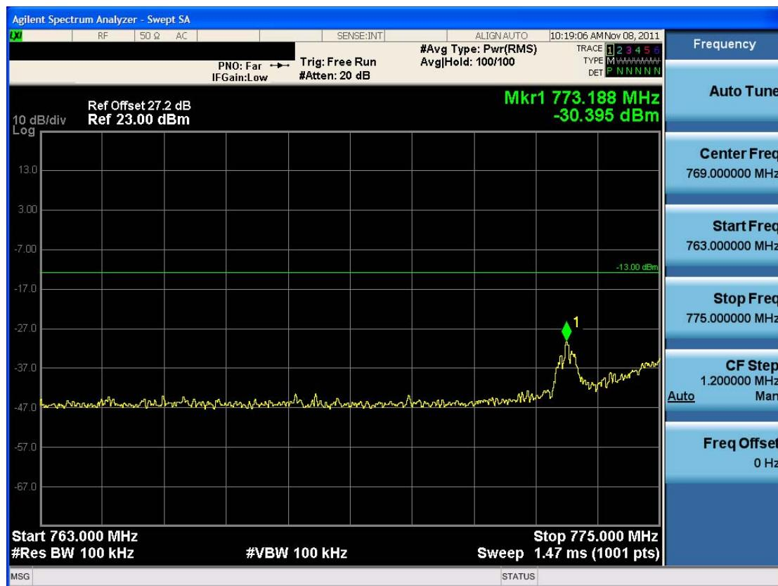
■ Low Emission Mask (763 MHz – 775 MHz) 16-QAM –RB Size 50
