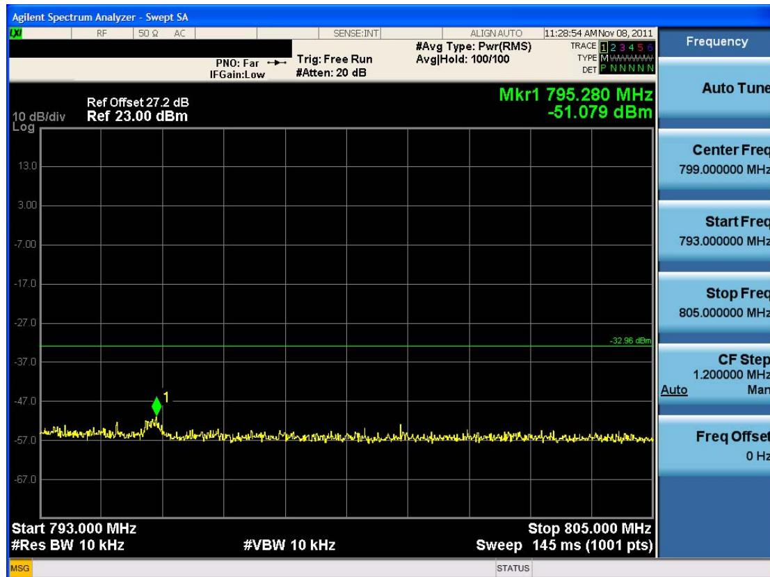
■ Upper Emission Mask (793 MHz – 805 MHz) QPSK –RB Size 50
