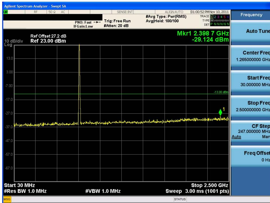
■ Conducted Spurious Emission (QPSK – RB Size 25, RB Offset 12)-2
