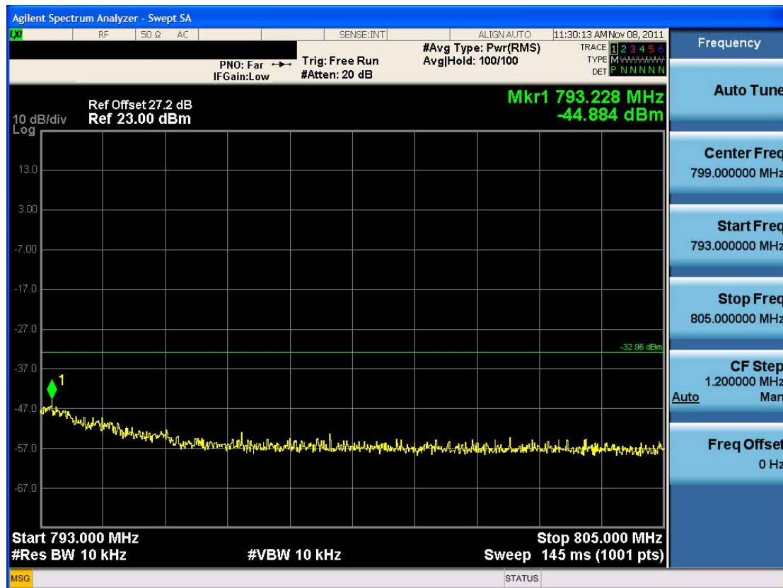
■ Conducted Spurious Emission (QPSK – RB Size 1, RB Offset 0)-1
