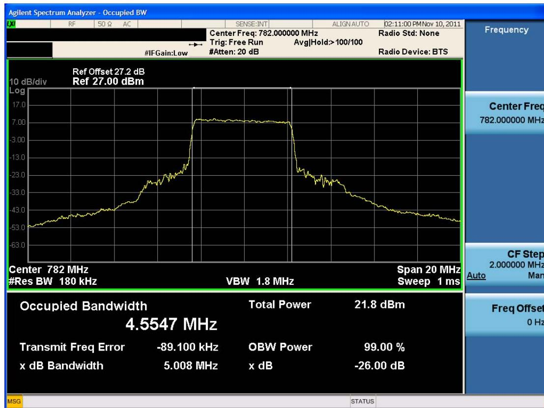
■ Occupied Bandwidth (16-QAM – RB Size 50)
