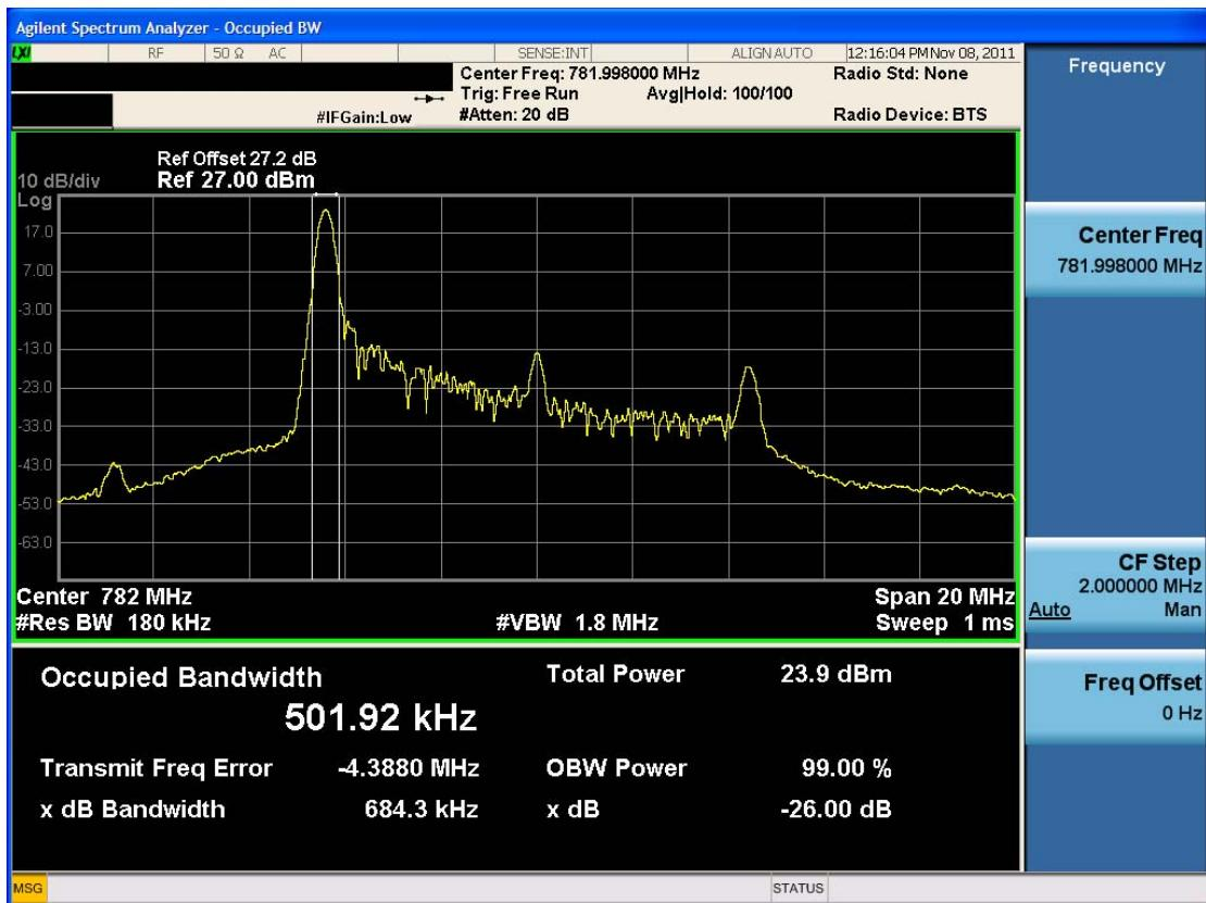
■ Occupied Bandwidth (QPSK – RB Size 1, RB Offset 49)
