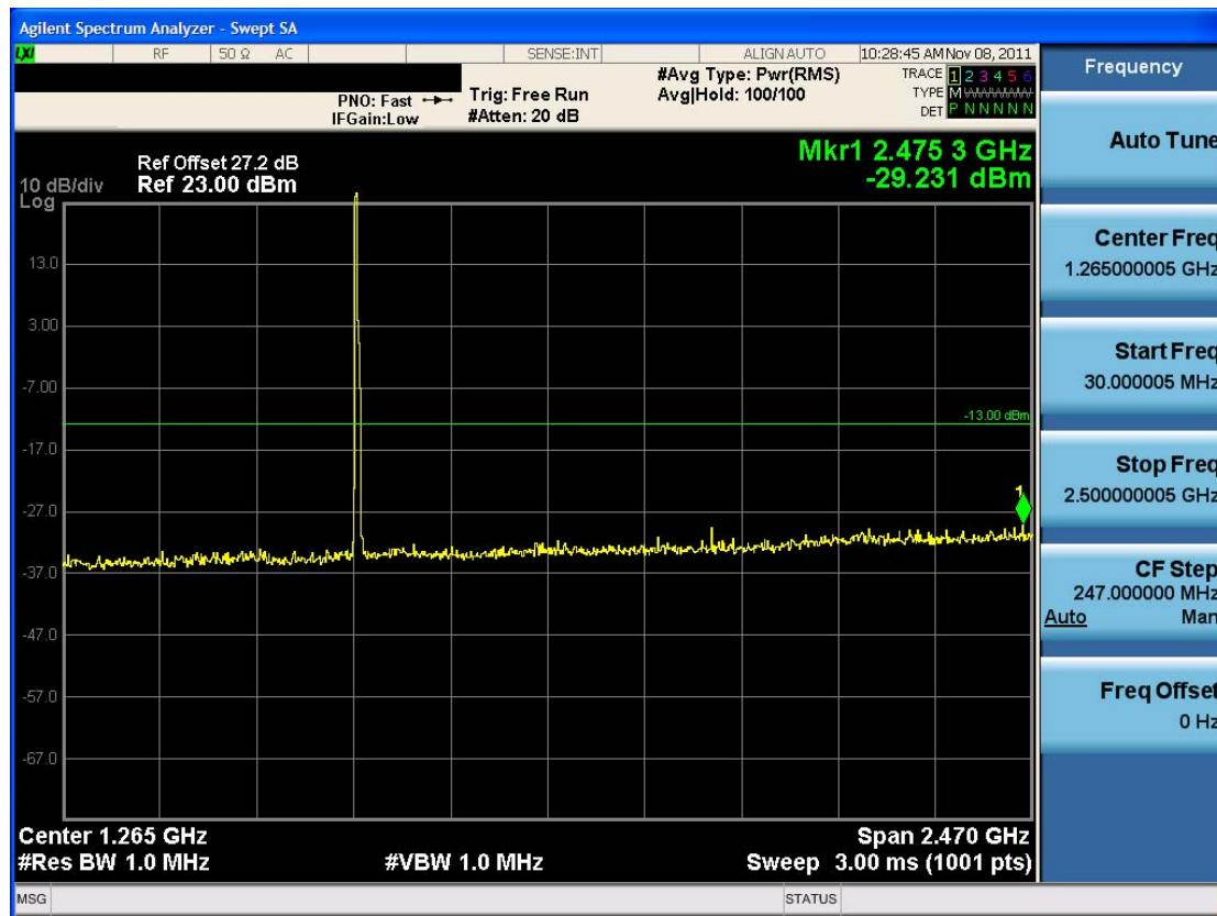
■ Conducted Spurious Emission (QPSK – RB Size 1, RB Offset 0)-2
