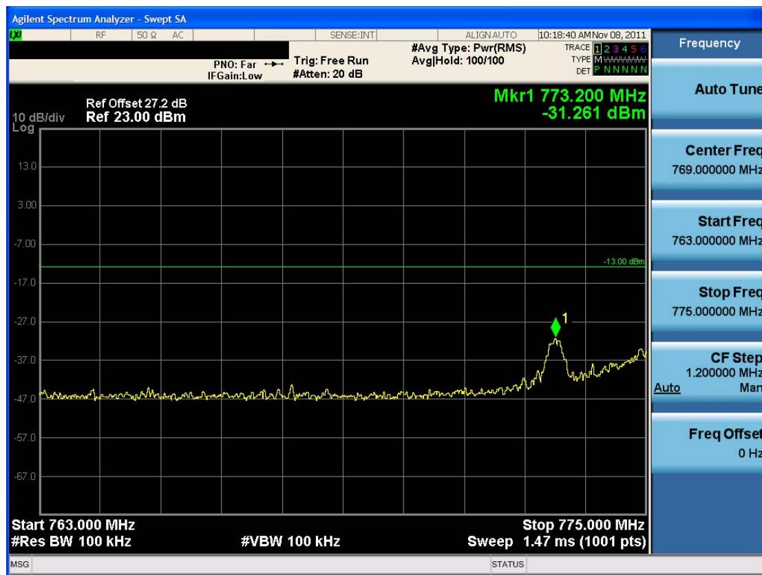
■ Low Emission Mask (763 MHz – 775 MHz) QPSK –RB Size 50
