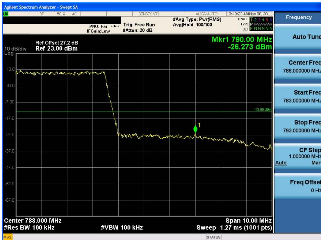
■ Low Emission Mask (763 MHz – 775 MHz) QPSK – RB Size 1, RB Offset 0)
