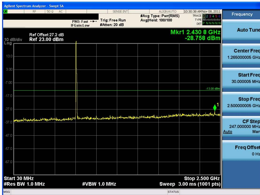
■ Conducted Spurious Emission (16-QAM – RB Size 1, RB Offset 0)-2
