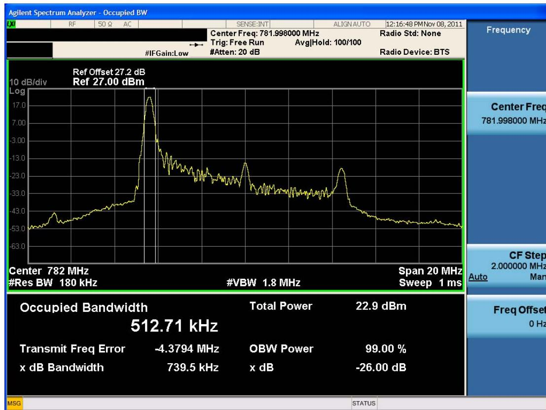
■ Occupied Bandwidth (16-QAM – RB Size 1, RB Offset 49)
