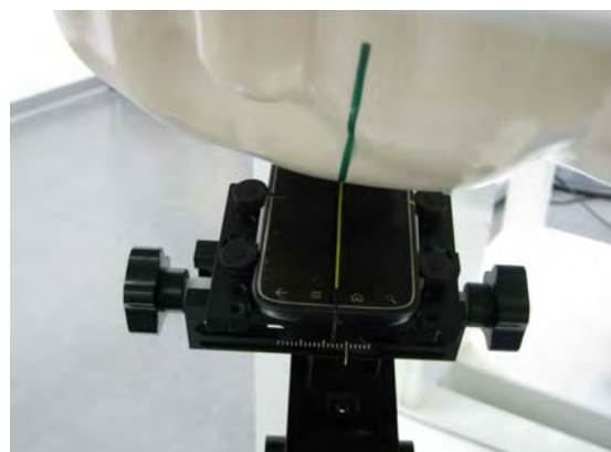
Fig.4 Right Head Section / Ear-Tilt Position(15°)
