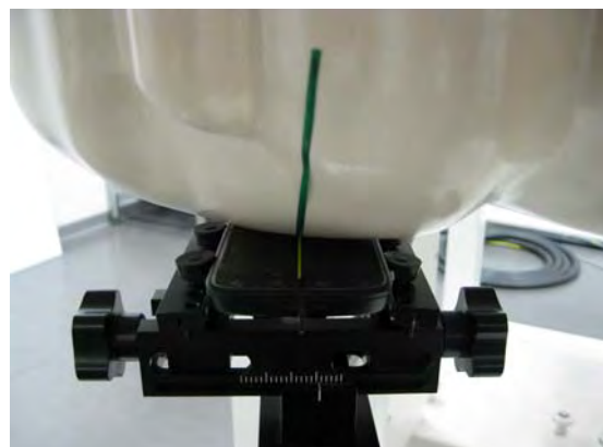
Fig.3 Right Head Section / Cheek-Touch Position
