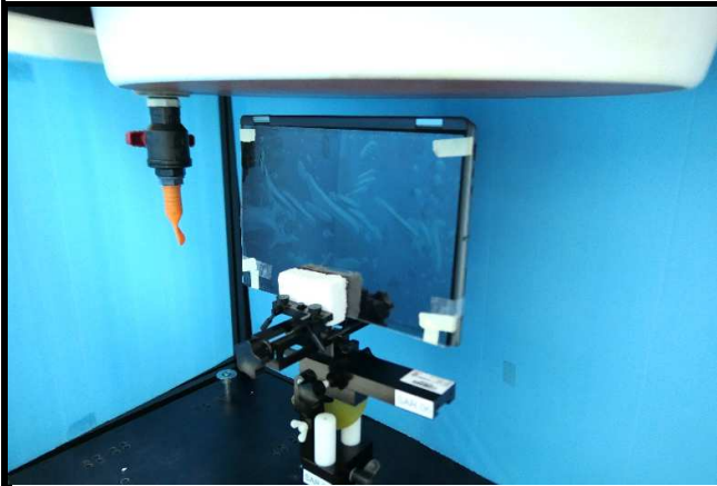
Bottom Side of Tablet Mode Tested at 19 mm
