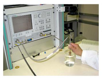
Tissue used during the SAR assessment is calibrated prior to the measurement process. APREL Laboratories use the co-axial probe method for all tissue calibration exercises. Tissue which is being used over a period of 24 hours is recalibrated to ensure that no dielectric change to the properties will affect the SAR measurement process. The table below provides details of the results from the tissue equivalent dielectric calibration.
