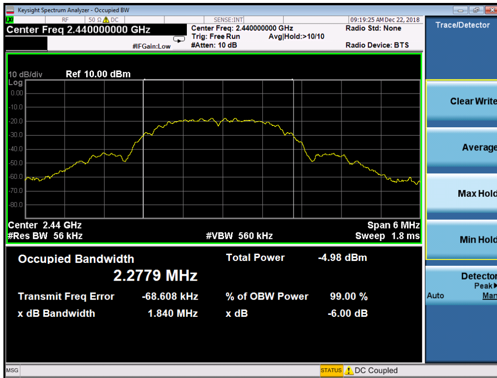
Occupied Bandwidth, Mid Channel
