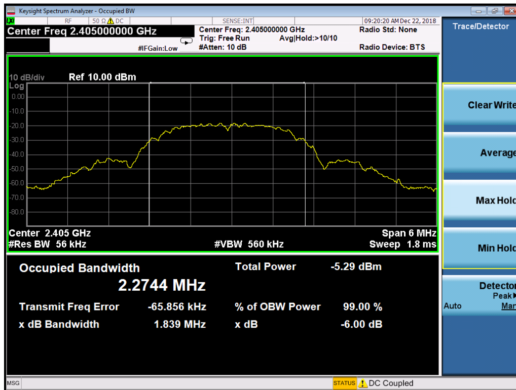
Occupied Bandwidth, Low Channel
