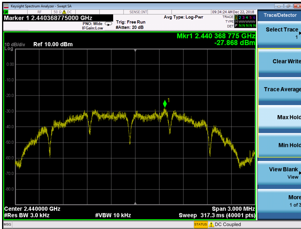
Power Spectral Density, Mid Channel
