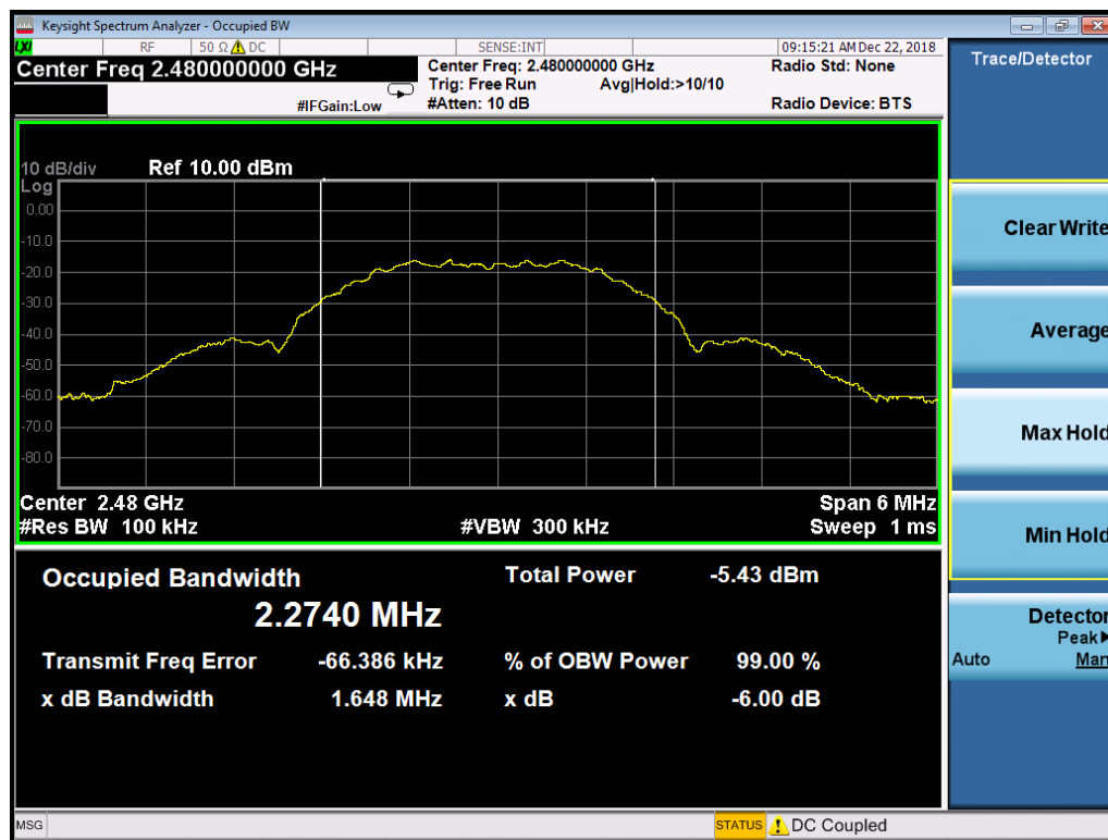
DTS Bandwidth, High Channel
