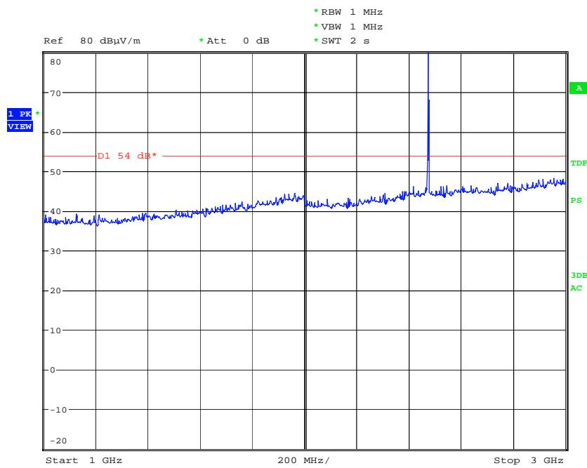
Note: The peak shown in the plot is the carrier frequency.
