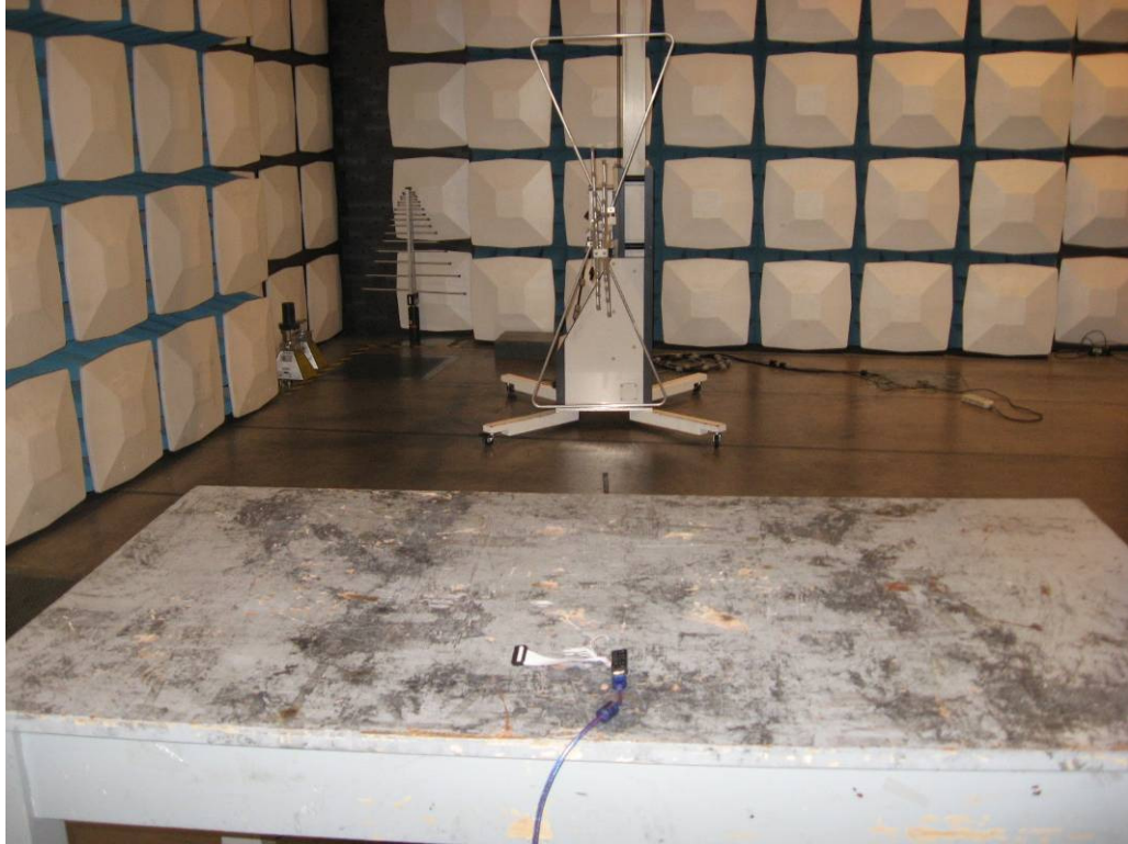
Photograph 6: Set-up for Spurious Emissions (1GHz-18GHz)
