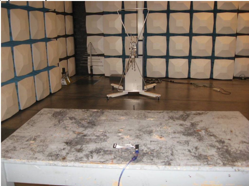
Photograph 2: Set-up for Radiated Emissions
