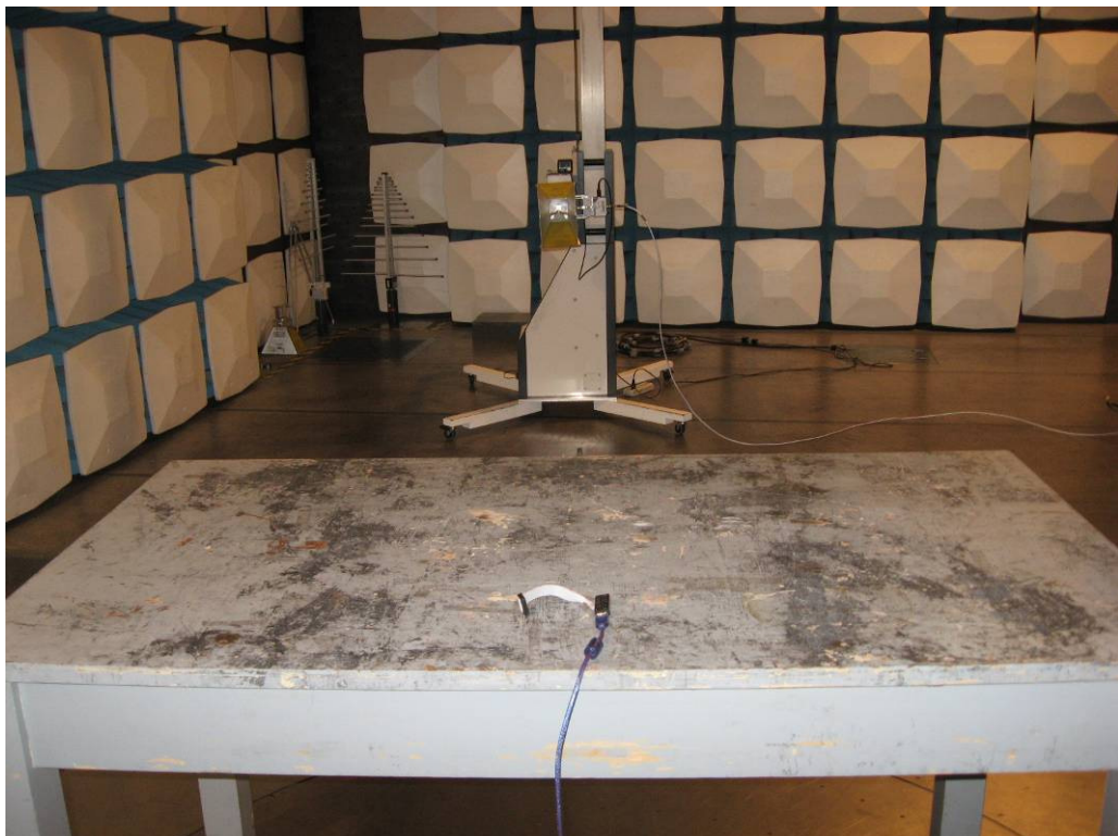
Photograph 6: Set-up for Spurious Emissions (1GHz-18GHz)
