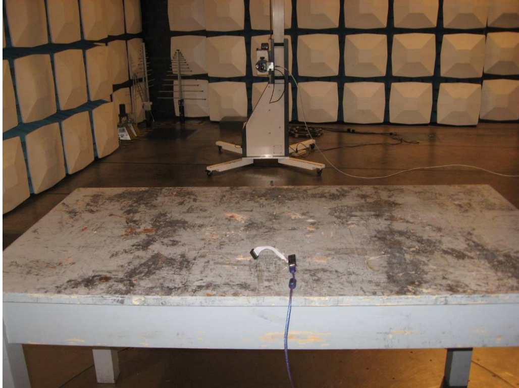
Photograph 7: Set-up for Spurious Emissions (18GHz-26GHz)
