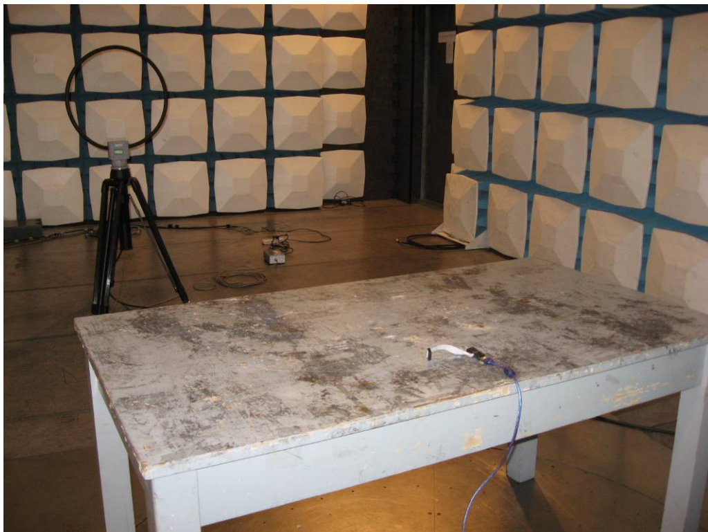
Photograph 4: Set-up for Spurious Emissions (9kHz-30MHz)
