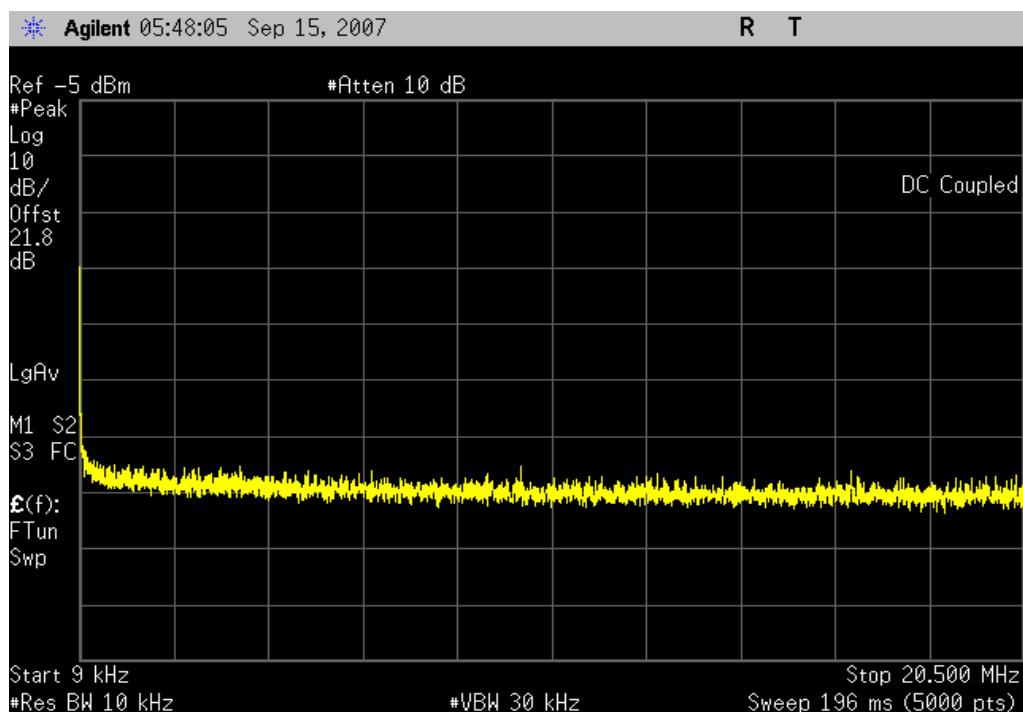
Bluetooth, 8DPSK, 3DH5, Mid channel, 2441MHz, 20 MHz - 3.1 GHz
