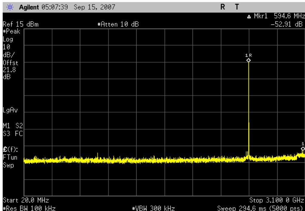
Bluetooth, pi/4-DQPSK, 2DH5, High channel, 2480MHz, 3 GHz - 6.6 GHz
