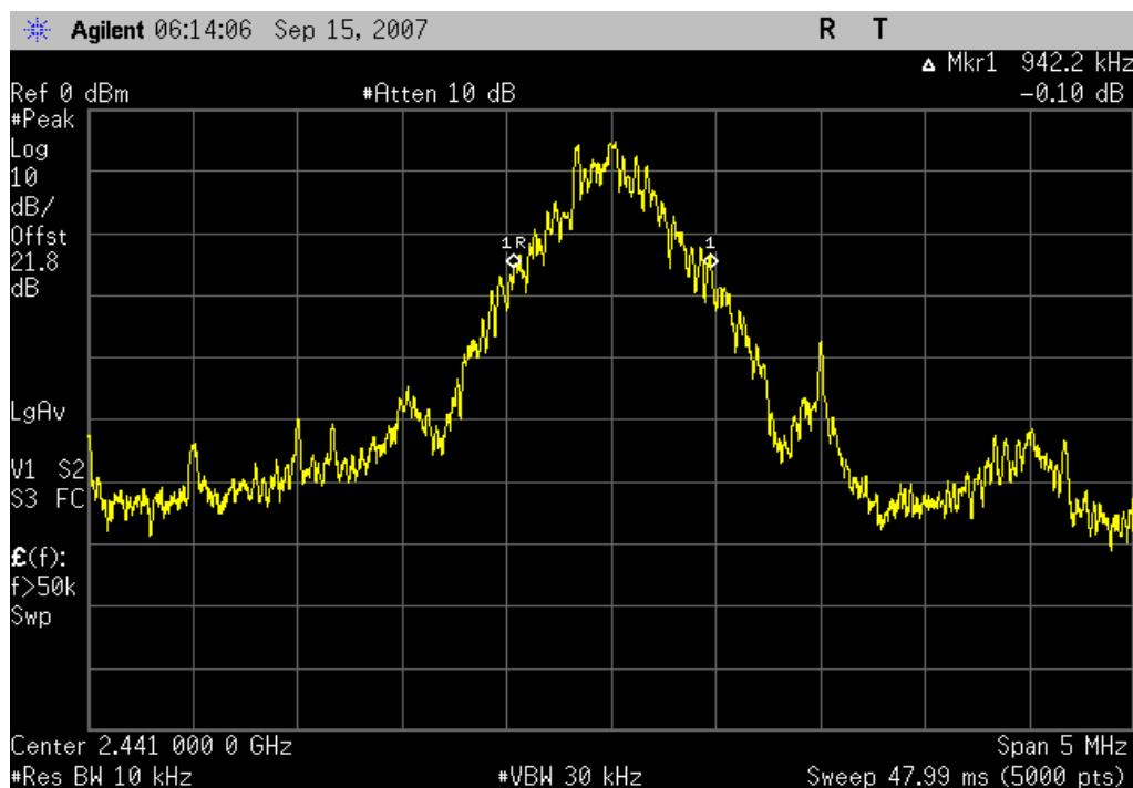
20 dB Bandwidth, Bluetooth, GFSK, DH5, High channel, 2480MHz
