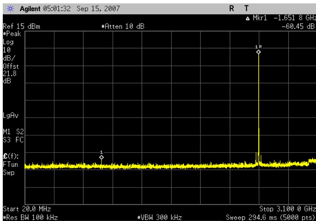
Bluetooth, 8DPSK, 3DH5, High channel, 2480MHz, 3 GHz - 6.6 GHz
