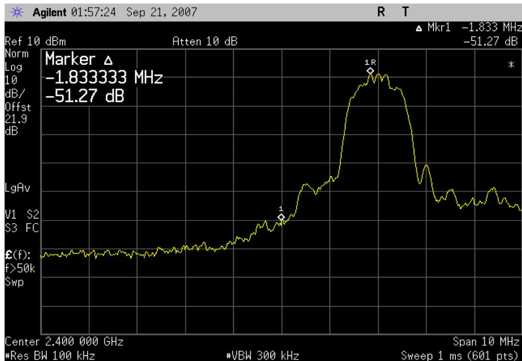
Bluetooth, 8-DPSK, 3DH5, High channel, 2480MHz
