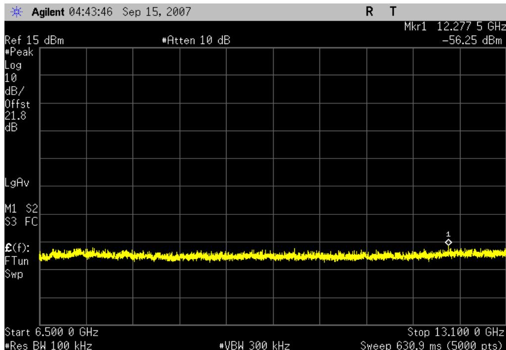
Bluetooth, 8DPSK, 3DH5, Mid channel, 2441MHz, 13 GHz - 26 GHz
