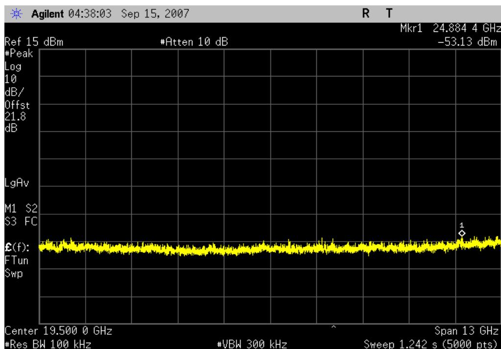
Bluetooth, 8DPSK, 3DH5, Low channel, 2402MHz, 9 kHz - 20.5 MHz
