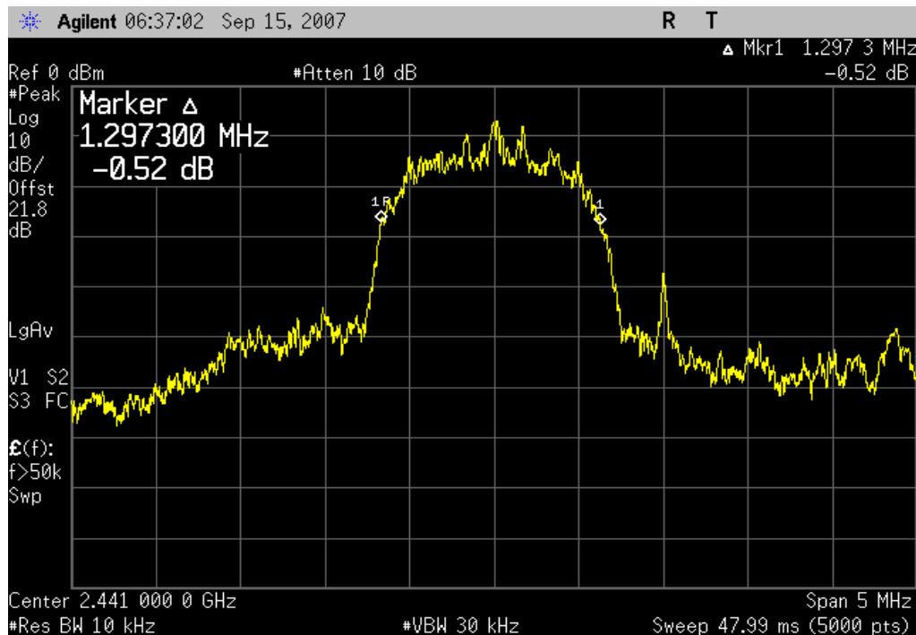
20 dB Bandwidth, Bluetooth, 8DPSK, 3DH5, High channel, 2480MHz
