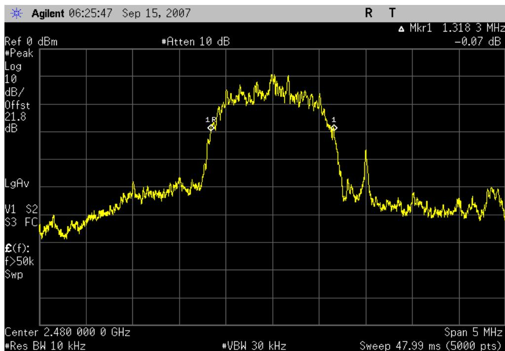
20 dB Bandwidth, Bluetooth, 8DPSK, 3DH5, Low channel, 2402MHz
