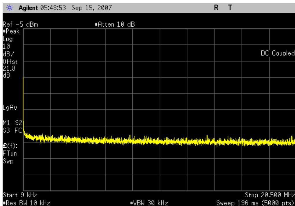
Bluetooth, 8DPSK, 3DH5, High channel, 2480MHz, 20 MHz - 3.1 GHz
