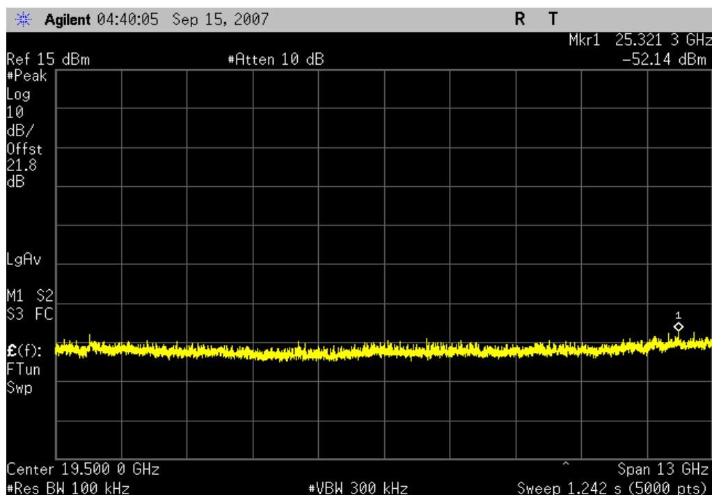
Bluetooth, 8DPSK, 3DH5, High channel, 2480MHz, 9 kHz - 20.5 MHz
