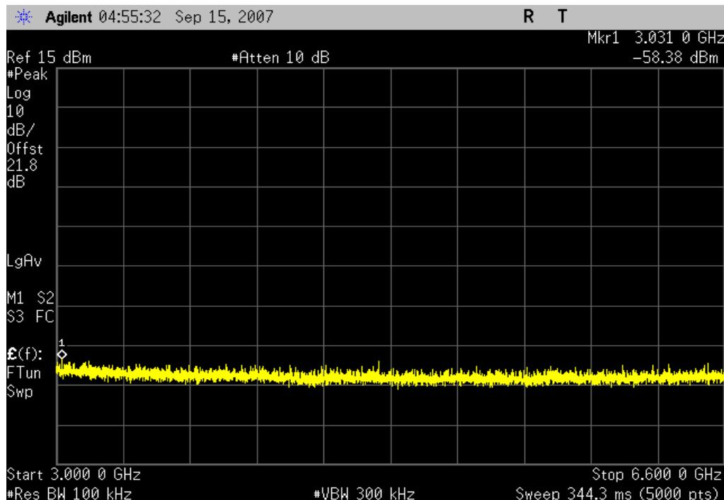
Bluetooth, 8DPSK, 3DH5, Low channel, 2402MHz, 6.5 GHz - 13.1 GHz
