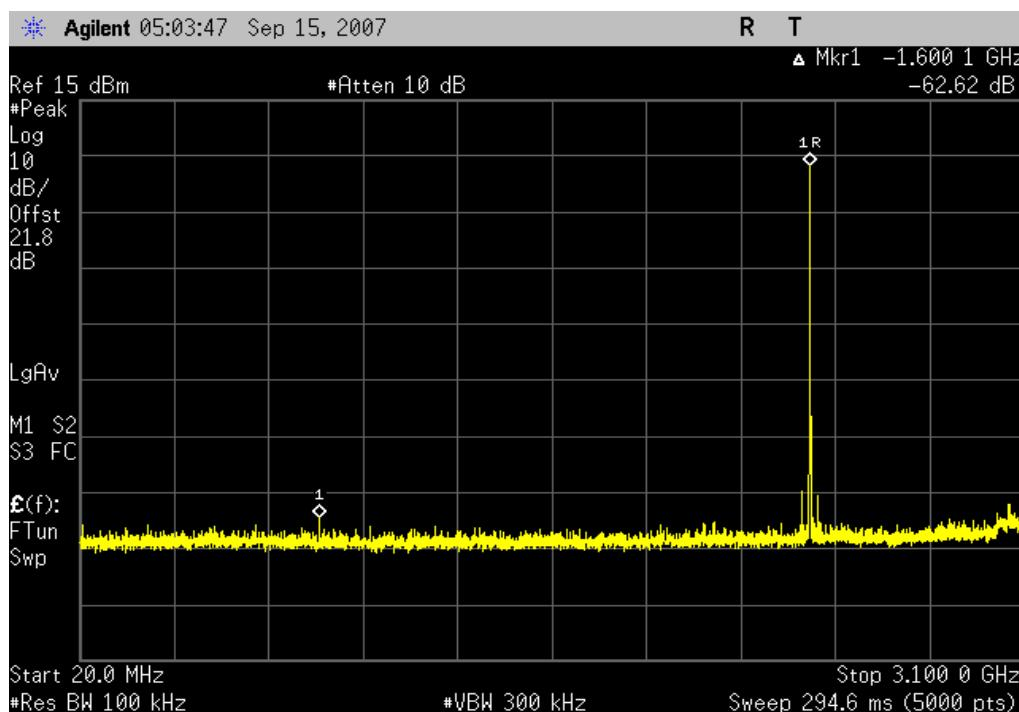
Bluetooth, 8DPSK, 3DH5, Low channel, 2402MHz, 3 GHz - 6.6 GHz
