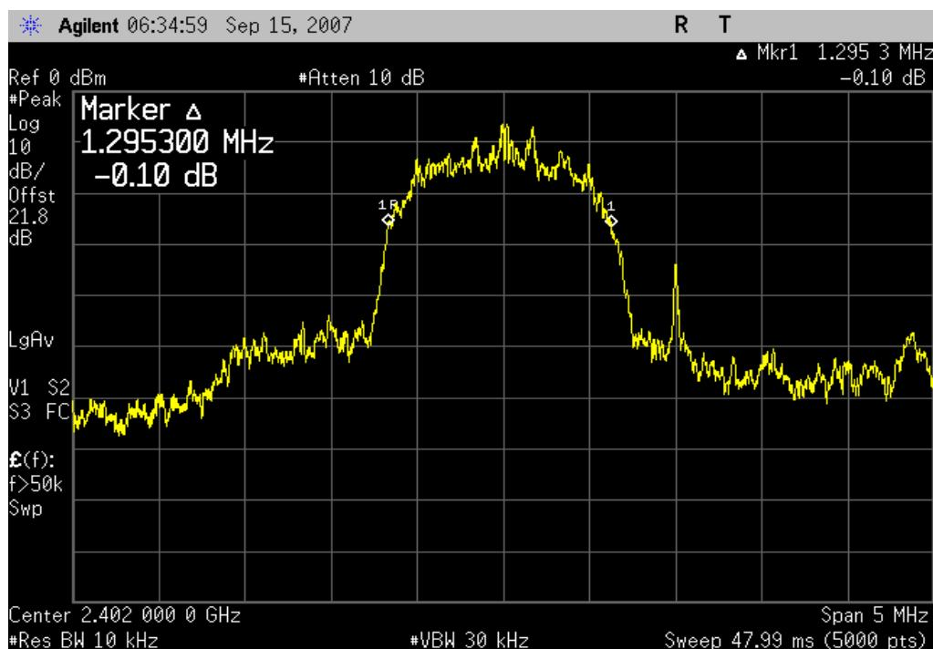
20 dB Bandwidth, Bluetooth, 8DPSK, 3DH5, Mid channel, 2441MHz
