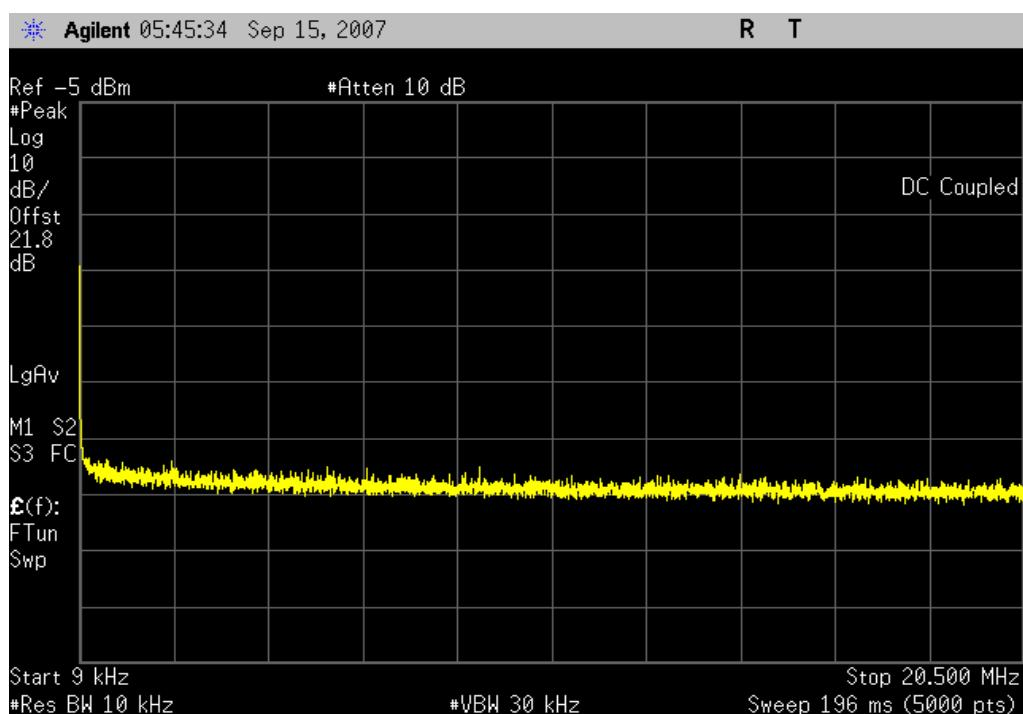
Bluetooth, pi/4-DQPSK, 2DH5, High channel, 2480MHz, 20 MHz - 3.1 GHz
