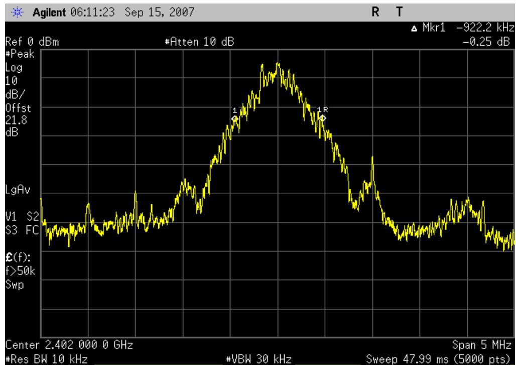
20 dB Bandwidth, Bluetooth, GFSK, DH5, Mid channel, 2441MHz
