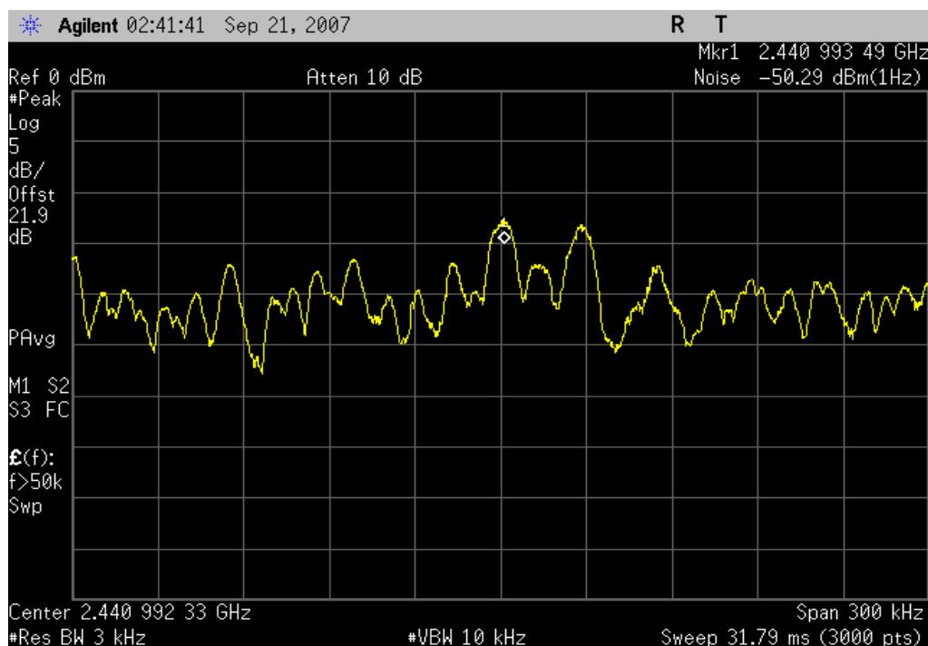
Bluetooth, 8-DPSK, 3DH5, High channel, 2480MHz
