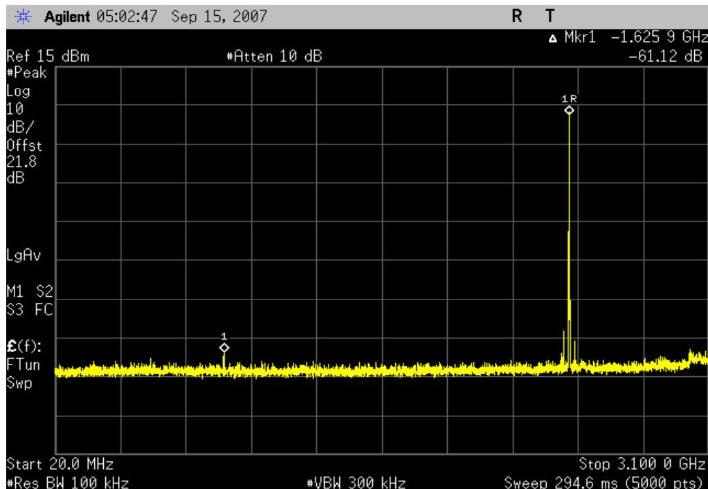
Bluetooth, 8DPSK, 3DH5, Mid channel, 2441MHz, 3 GHz - 6.6 GHz
