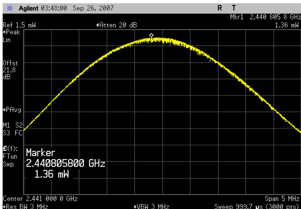
Bluetooth, 8DPSK, 3DH5, High channel, 2480MHz
