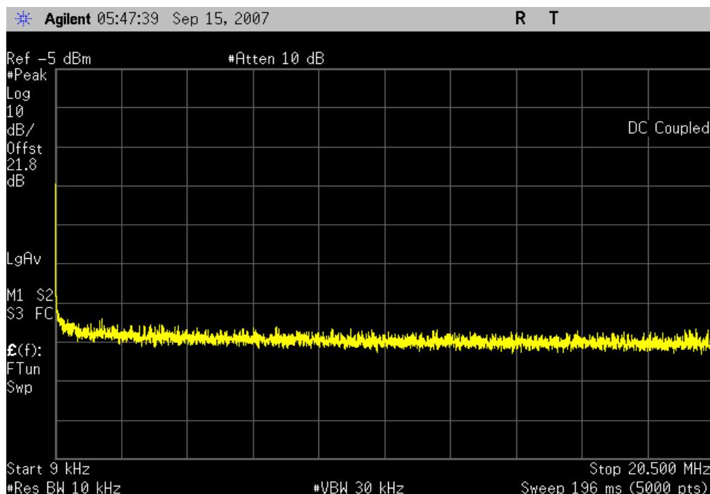
Bluetooth, 8DPSK, 3DH5, Low channel, 2402MHz, 20 MHz - 3.1 GHz
