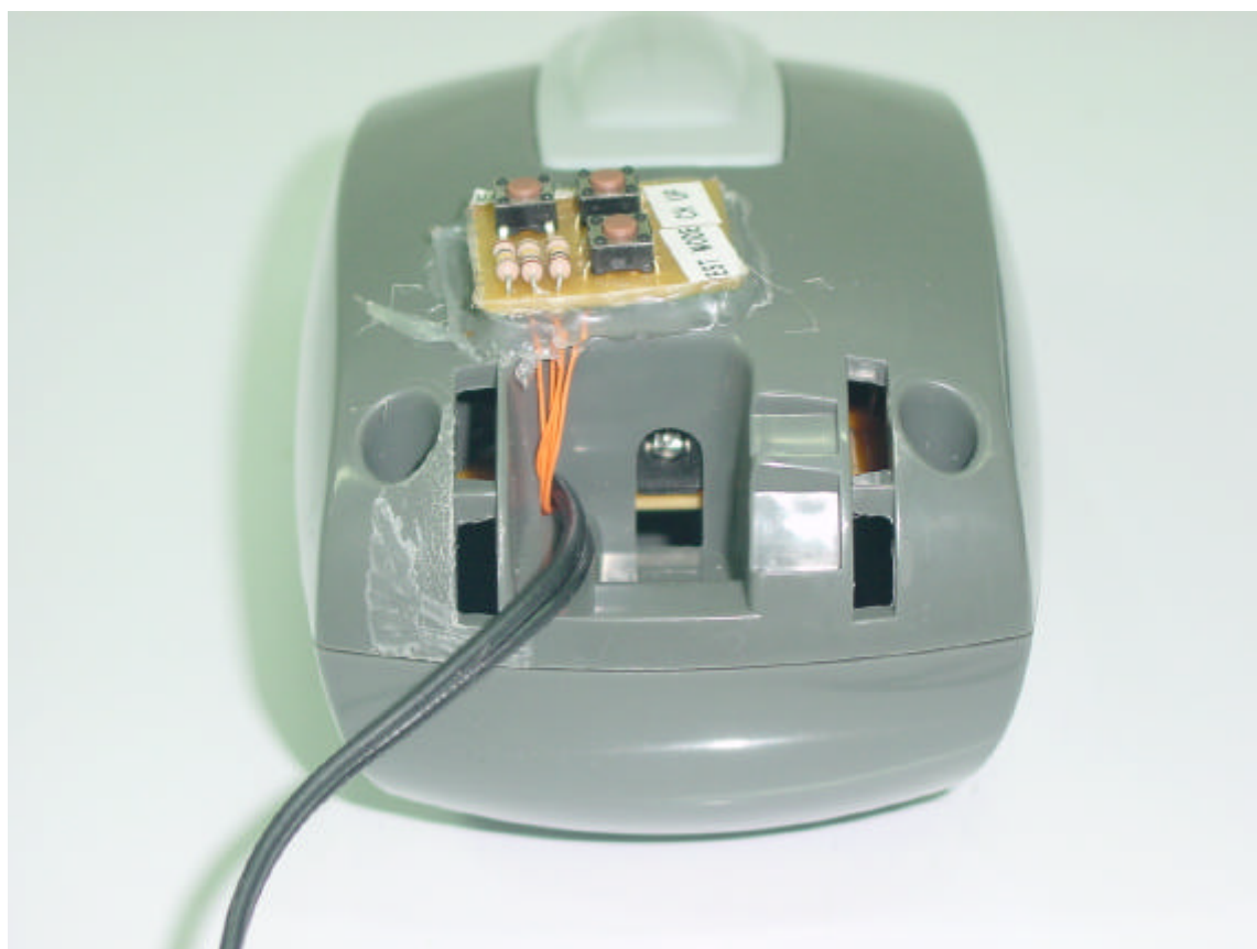
Adaptor Jack (The outside PCB only for switching channel in during test)
