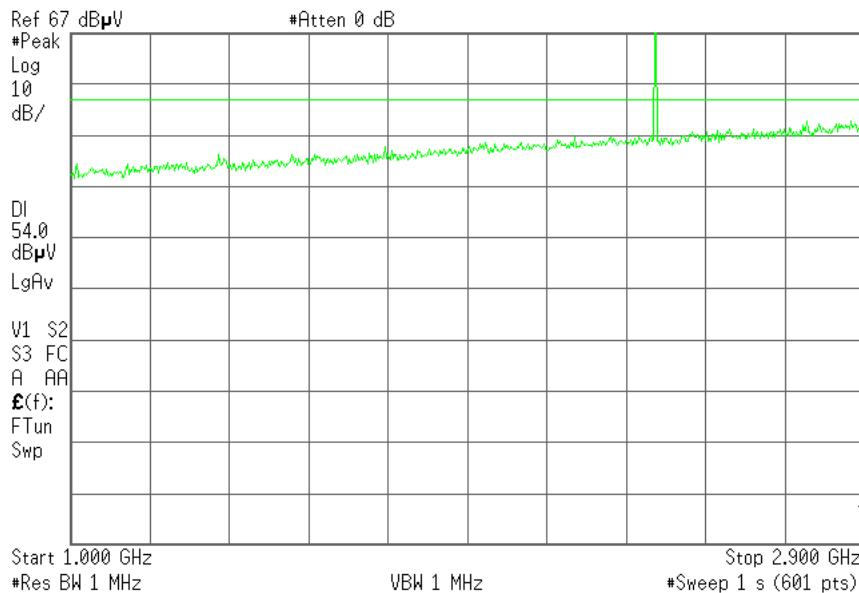
Note: The peak above the limit is the carrier frequency.
