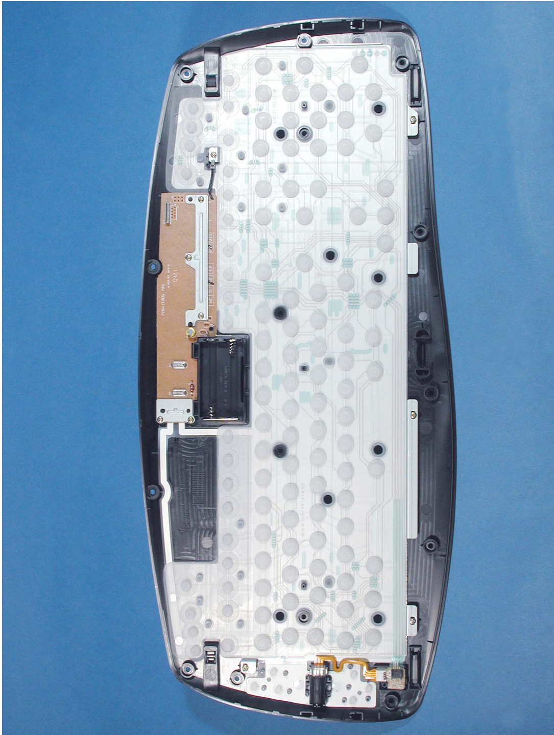
Photograph 1: Y-RR54 internal view (membrane)
