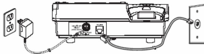
To retain full operation of ClearVoice 50B, 100B or 200B during power failures insert 4 AA batteries (not included) into the battery compartment located at bottom of unit. You may do this by simply disconnecting the AC adaptor from the power source, then removing the battery cover, connecting the batteries and replacing the cover. Then immediately connect AC Adaptor to AC outlet to assure battery life is not being affected. Note: The AA batteries should be alkaline.
