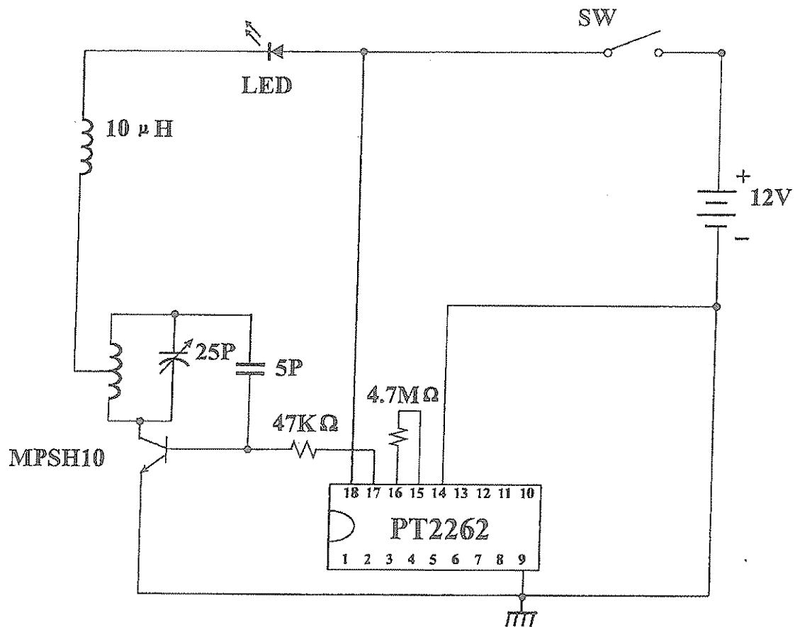
UHF Band Address-only (Zero Data) Zero-Stand-by Transmitter Circuit is recommended.
