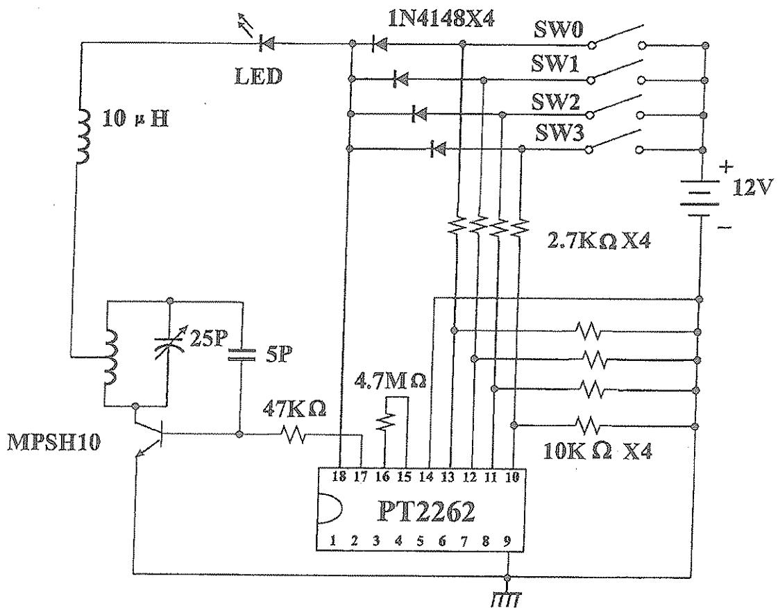
UHF Band 4 Data Transmitter Circuit is recommended.
