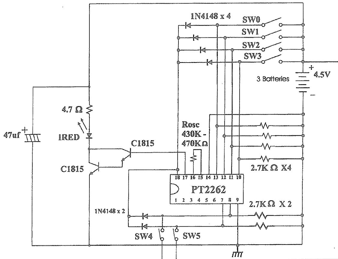
Infrared Ray 6-Data Circuit. Adjust Rosc to get 38 KHz Carrier Pulse at DOUT Pin is recommended.
