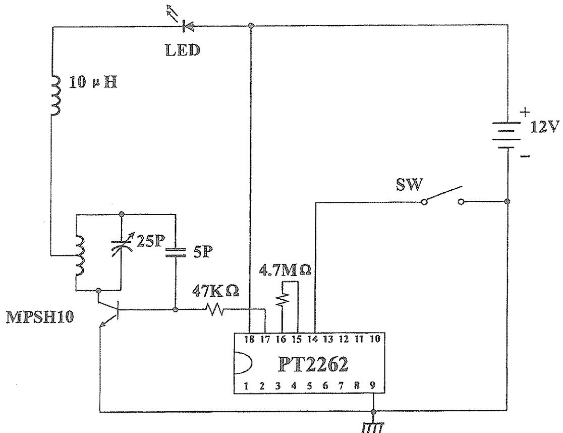
UHF Band Address-only (Zero Data) Transmitter Circuit is recommended.
