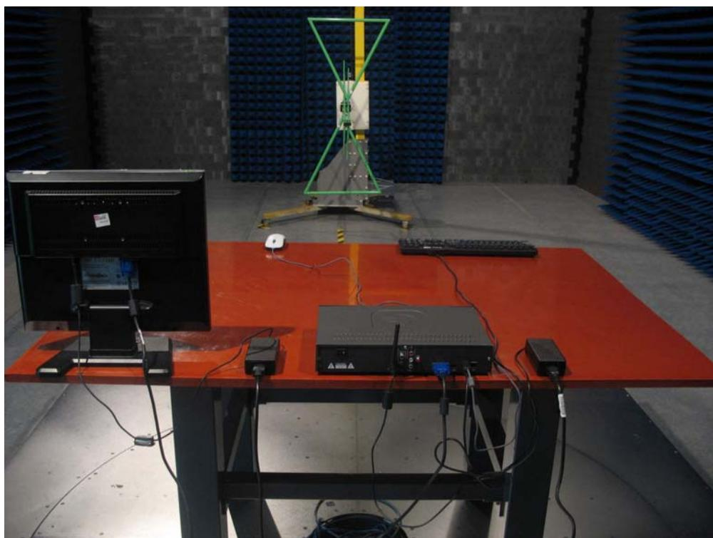
Test Mode: Mode 2: Transmit by 802.11g
