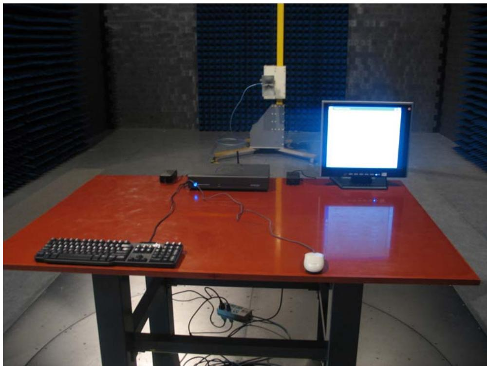
Test Mode: Mode 1: Transmit by 802.11b
