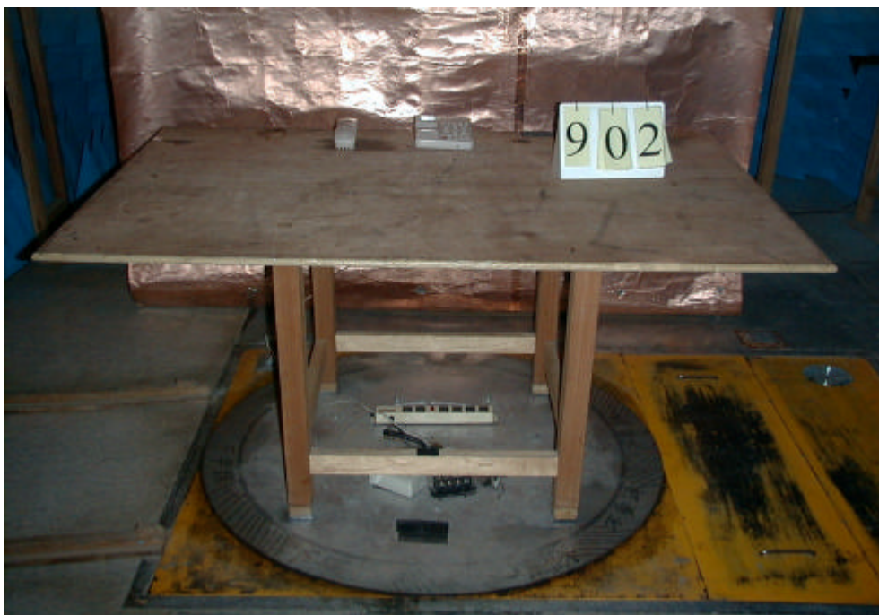
Fig. 1 Conducted Emissions Test Configuration (Operating only)
