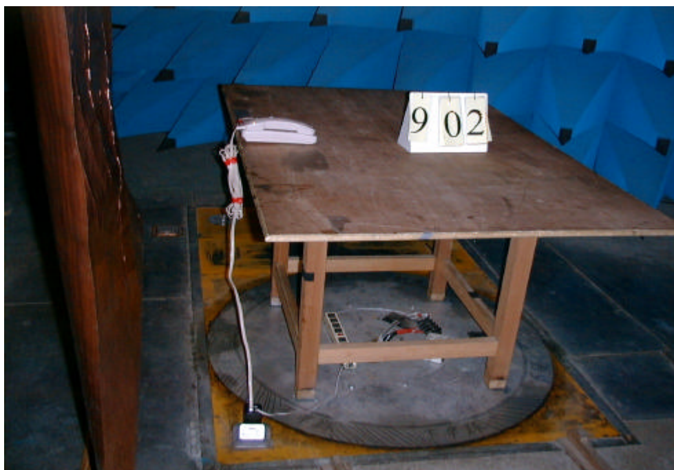
Fig. 2 Conducted Emissions Test Configuration (Charging only)
