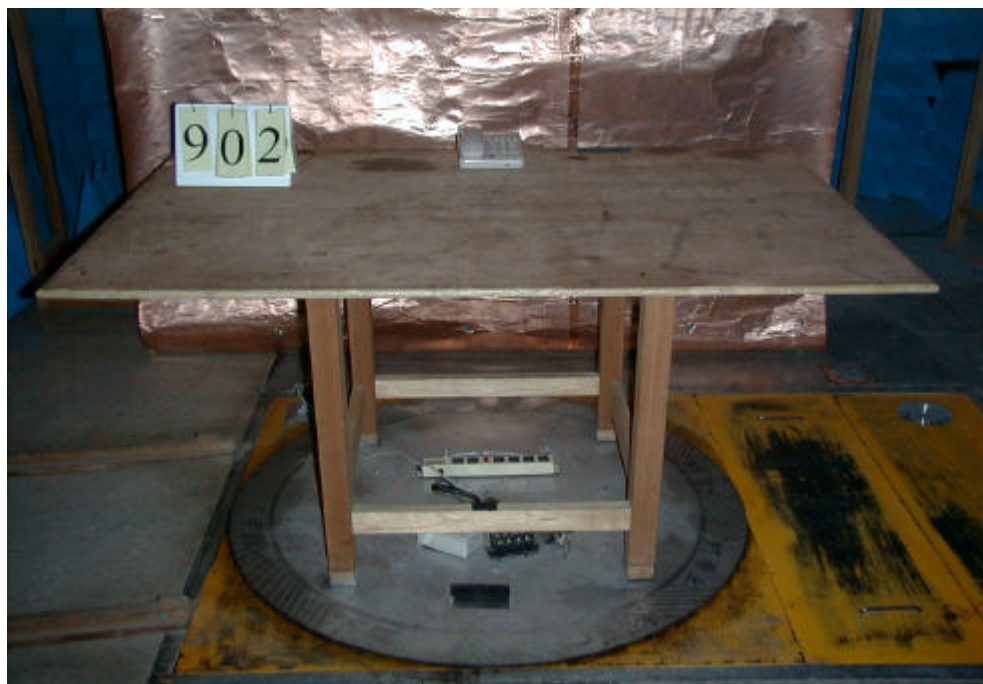
Fig. 1 Conducted Emissions Test Configuration (Charging only)
