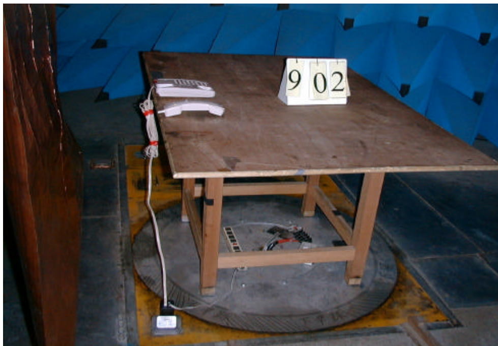
Fig. 2 Conducted Emissions Test Configuration (Operating only)
