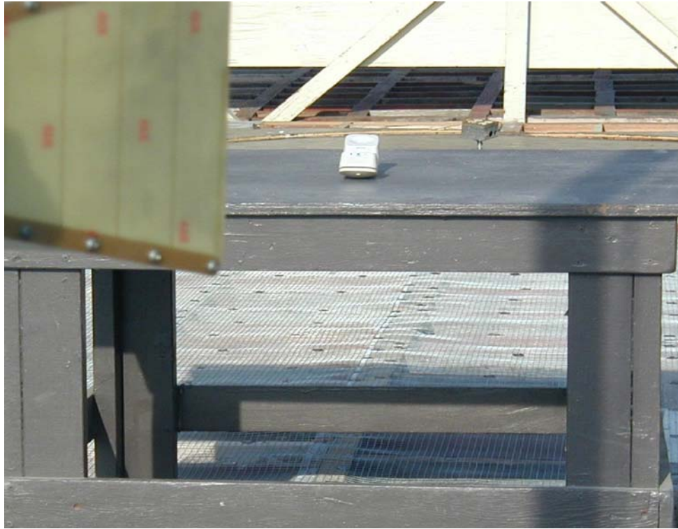
Figure 11: Front View: Harmonic, Spurious and Restricted Bands Test Setup for Headset Unit
