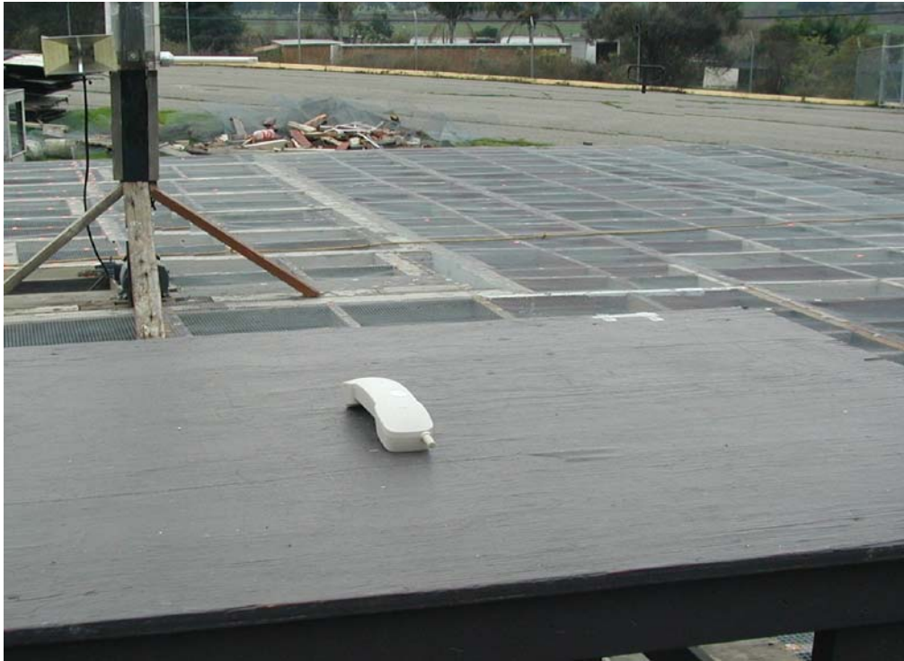
Figure 5: Handset Unit – Test Set-up Photo for Maximum Peak Output and Spectrum Density
