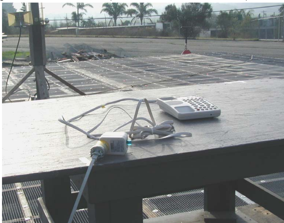
Figure 10: Rear View: Harmonic, Spurious and Restricted Bands Test Setup for Base Unit
