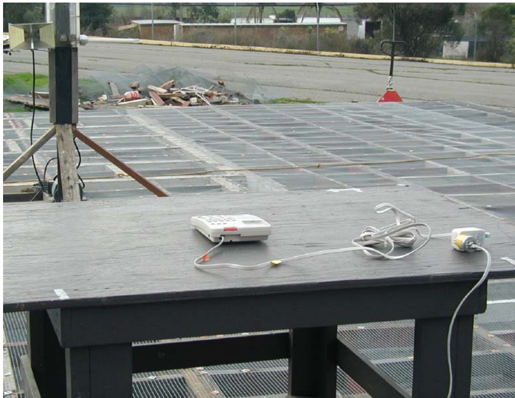
Figure 2: Base Unit – Band-Edge and 6dB Bandwidth Test Set-up Photo (Rear View)
