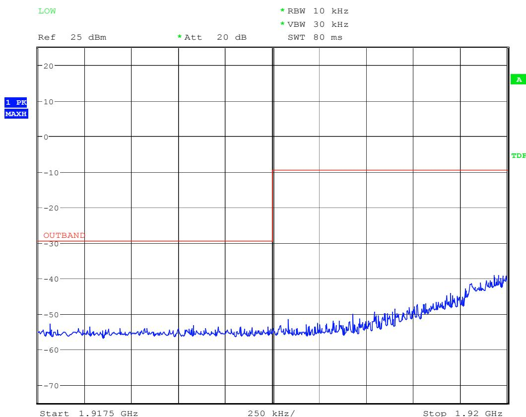
**Out-of-band Unwanted Emissions: CH F<sub>L</sub>.**
