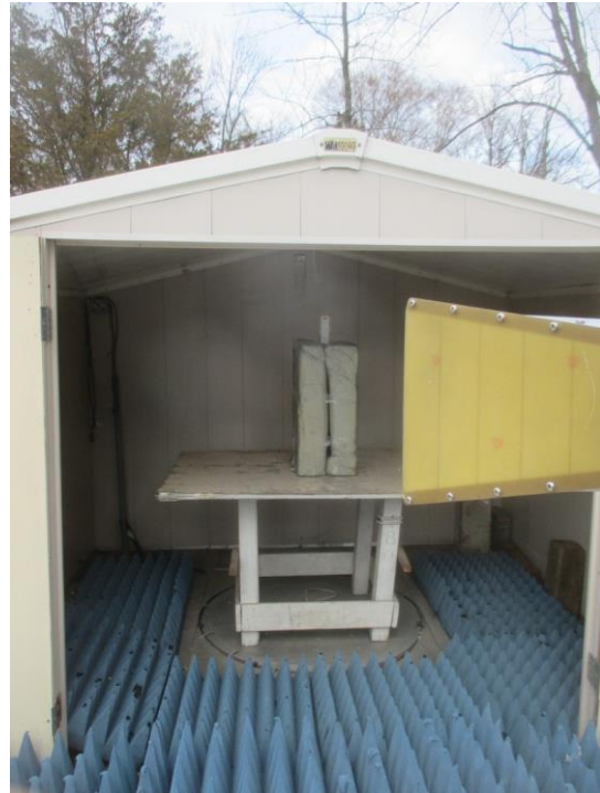
Figure 3.1 Radiated Test Setup
