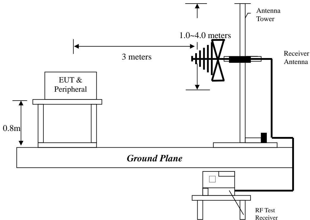
Radiated emissions were investigated over the frequency range from 30MHz to 1000MHz using a receiver RBW of 120kHz record QP reading, and the frequency over 1GHz using a spectrum analyzer RBW of 1MHz and 10Hz VBW record Average reading. (15.209 paragraph), the Peak reading (1MHz RBW/ 3MHz VBW) recorded also on the report.
