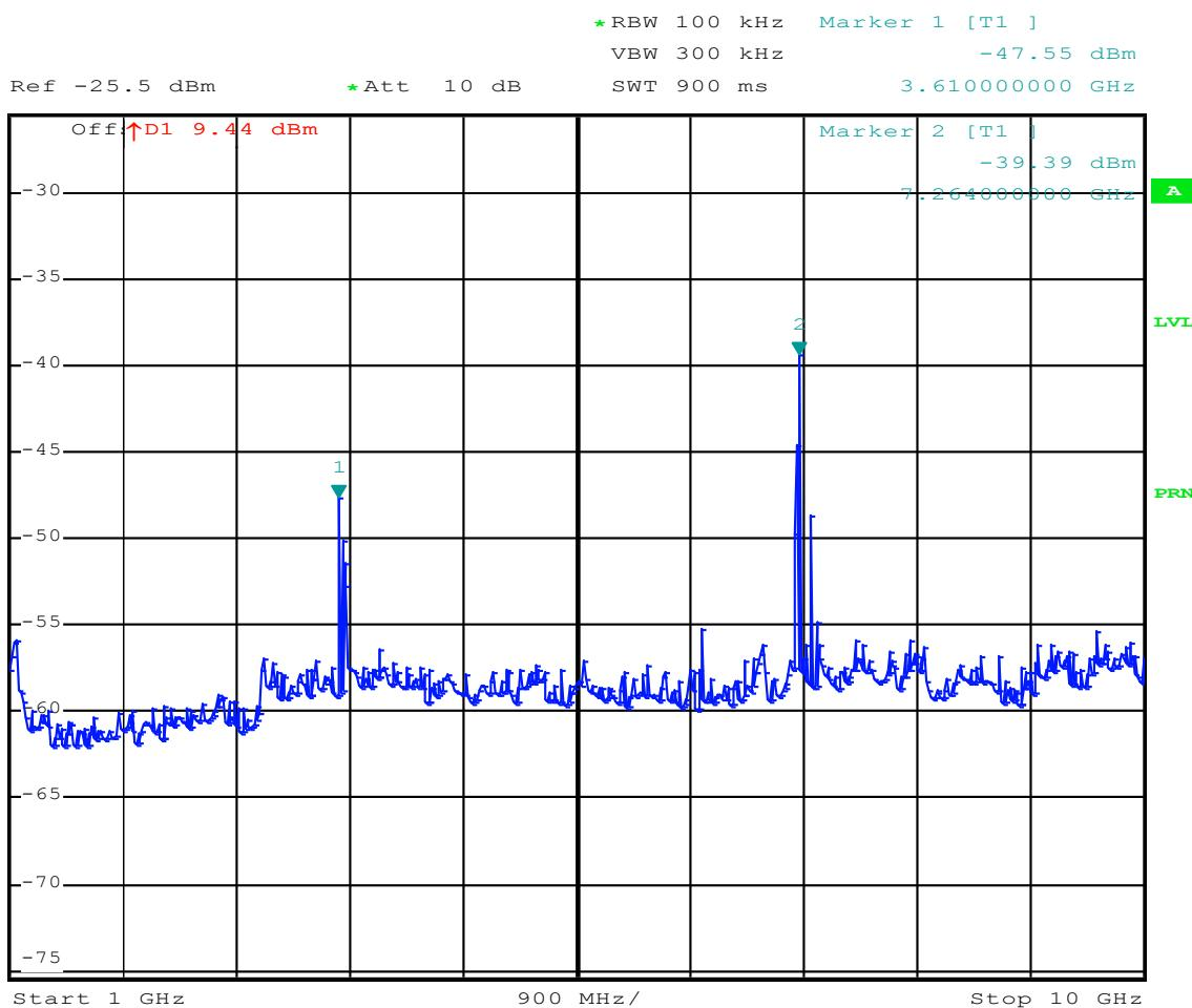
Note: Signal level no. 1 and no. 2 are located in restricted band.
