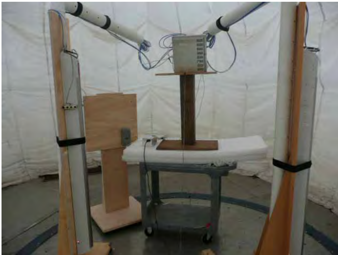
Figure 14 – Fundamental Emissions Test Setup - Configuration 2: Vertical Mount
