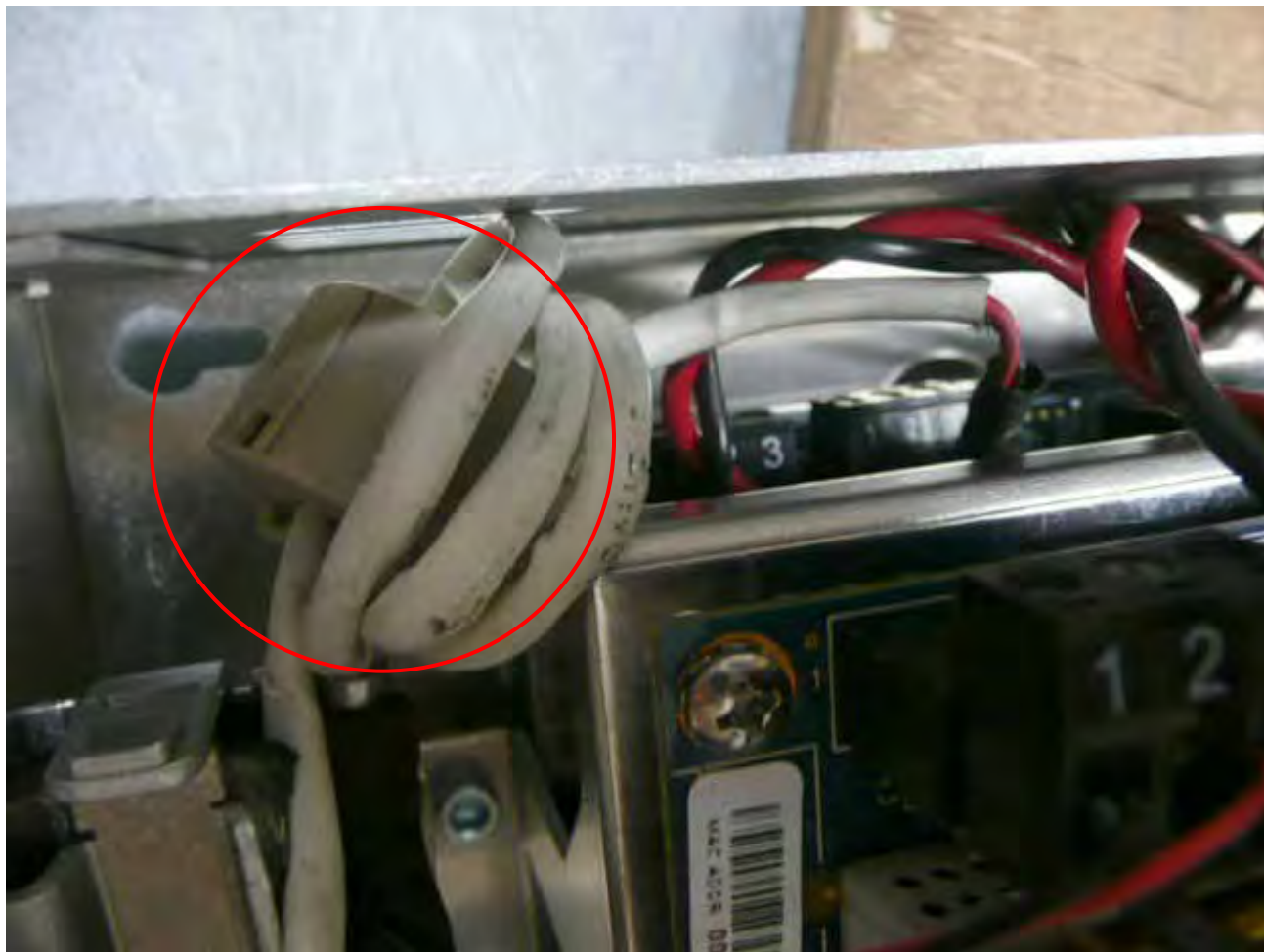
Figure 2 – Ferrite on DC side of Power Supply
