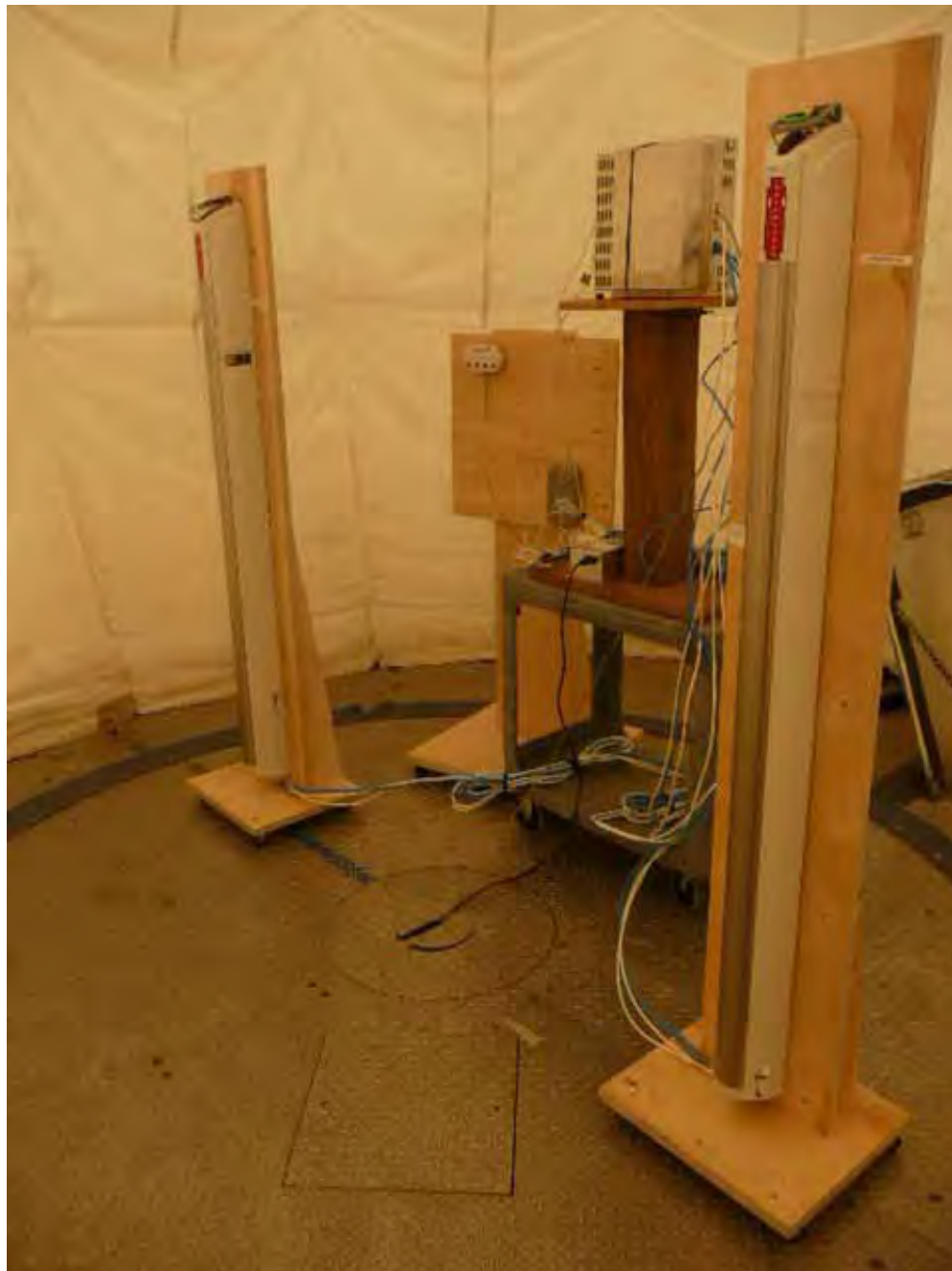
Figure 12 - Fundamental Emissions Test Setup - Configuration 1: Vertical Mount
