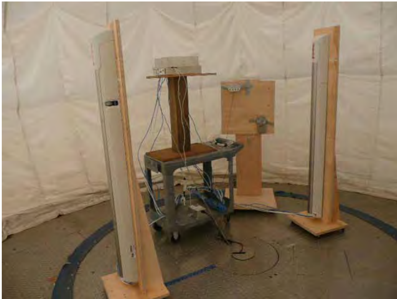
Figure 17 - Radiated Emissions (3m OATS) Test Setup. Configuration 1
