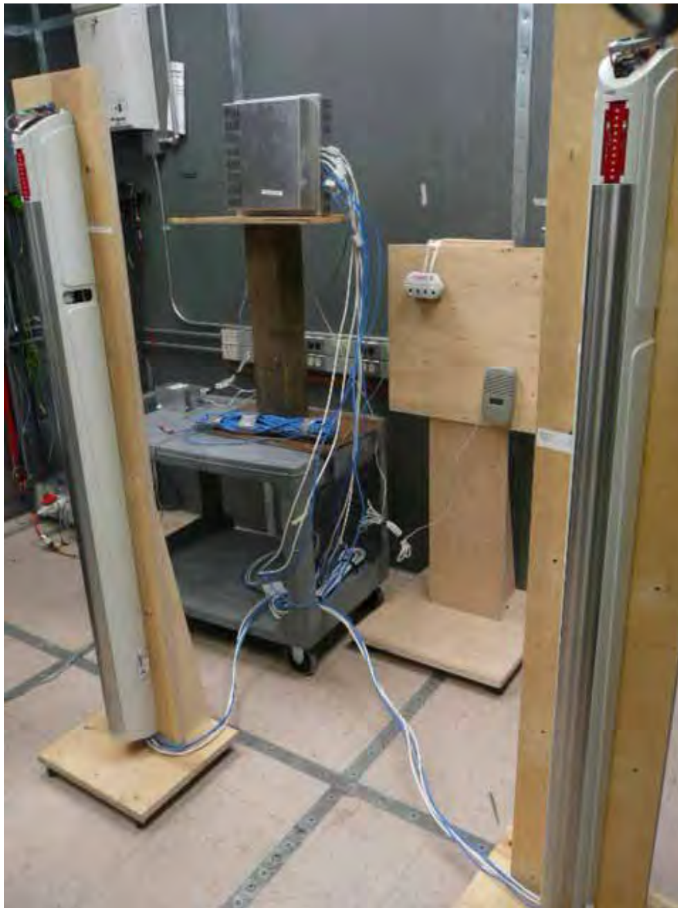
Figure 15 –Conducted Emissions Test Setup Configuration 1
