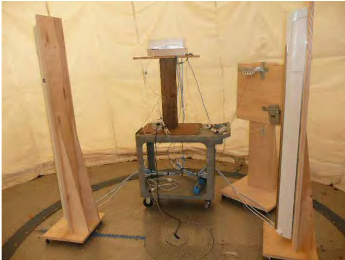
Figure 11 - Fundamental Emissions Test Setup - Configuration 1: Horizontal Mount
