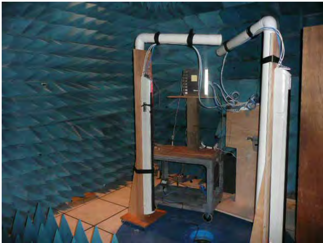
Figure 18 – Radiated Emissions Pre-scan Test Set-Up. Configuration 2
