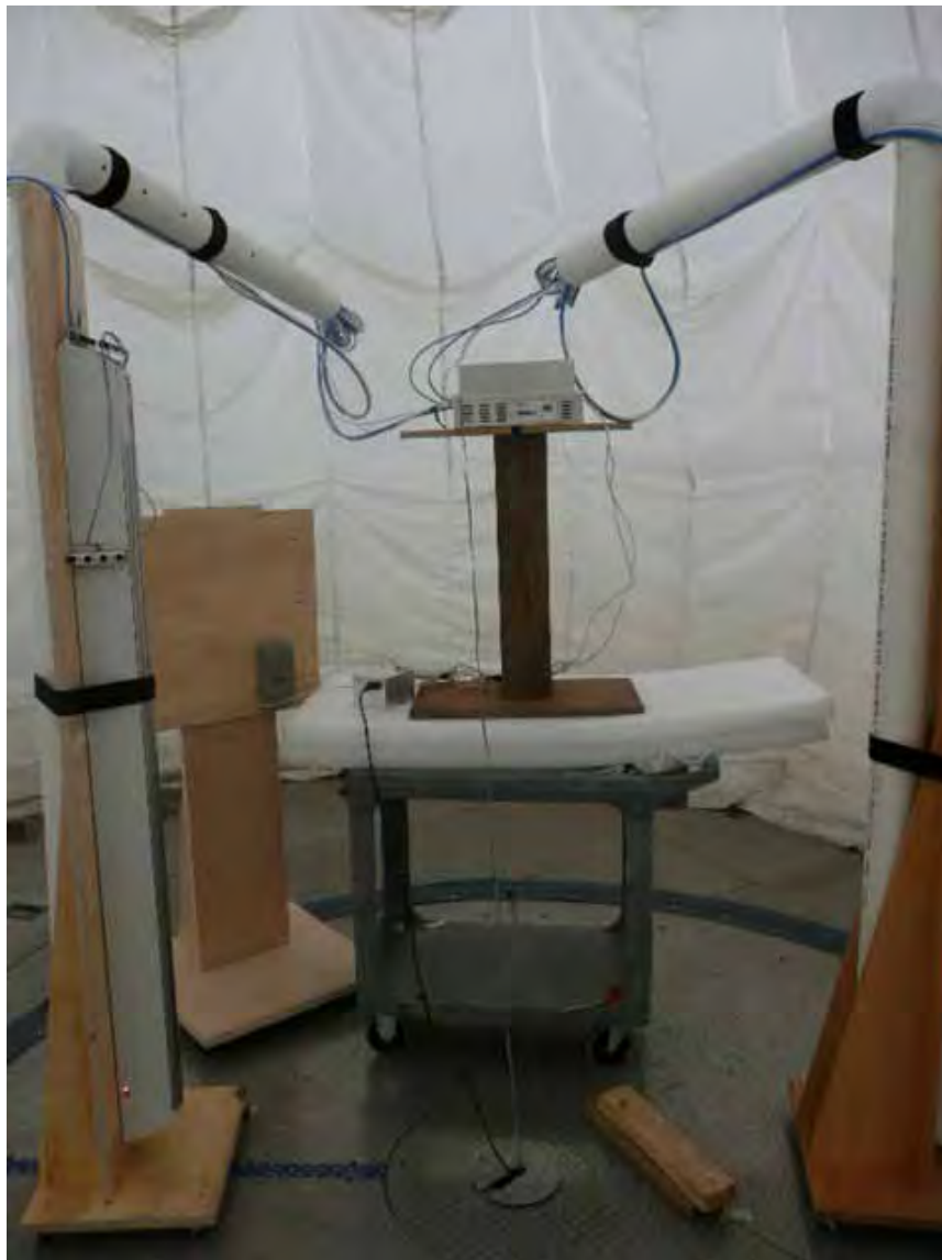
Figure 13 – Fundamental Emissions Test Setup - Configuration 2: Horizontal Mount
