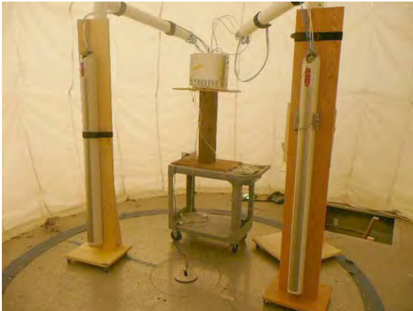
Figure 19 - Radiated Emissions (3m OATS) Test Setup. Configuration 2
