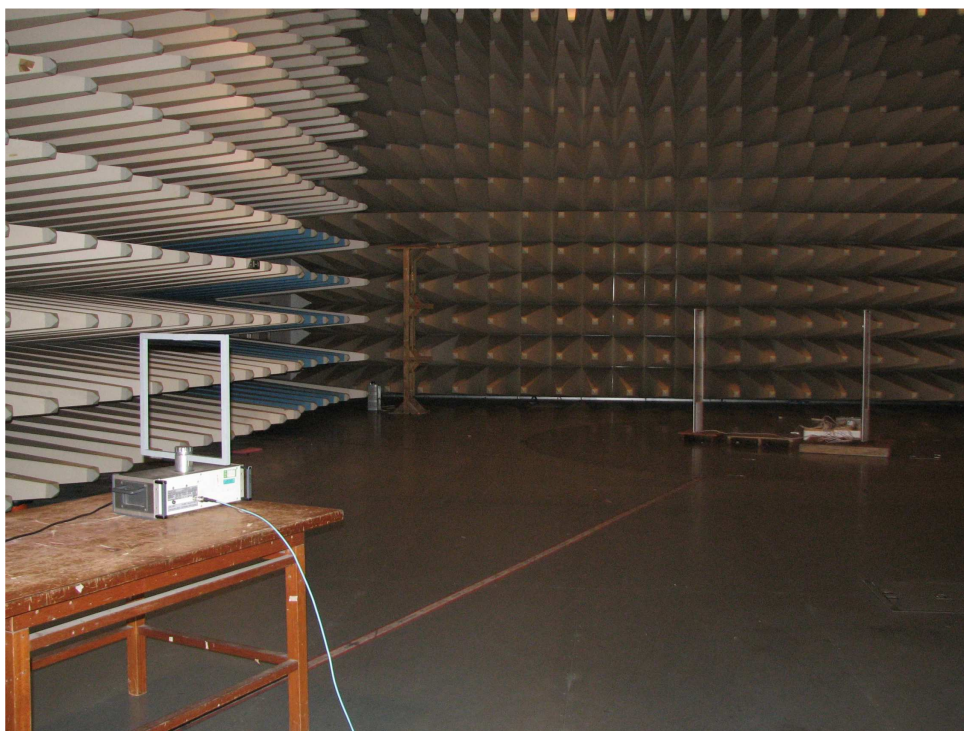
Photograph 2: Set-up for radiated emission (9kHz - 30MHz)
