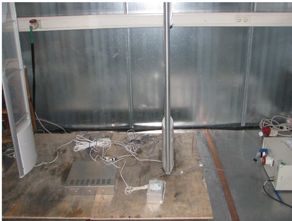
Photograph 2: Set-up for radiated emission (9kHz - 30MHz)
