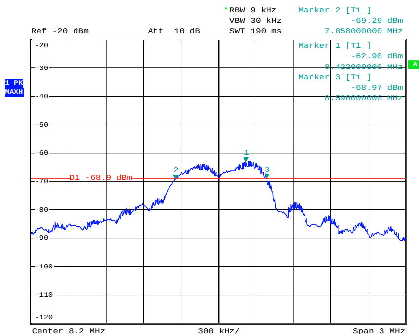
Figure 3: Spectral diagram, emission bandwidth measurement
