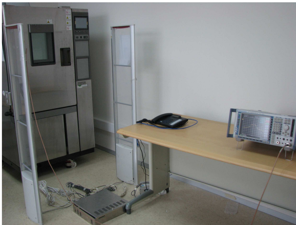
Photograph 4: Set-up for emission bandwidth & duty cycle
