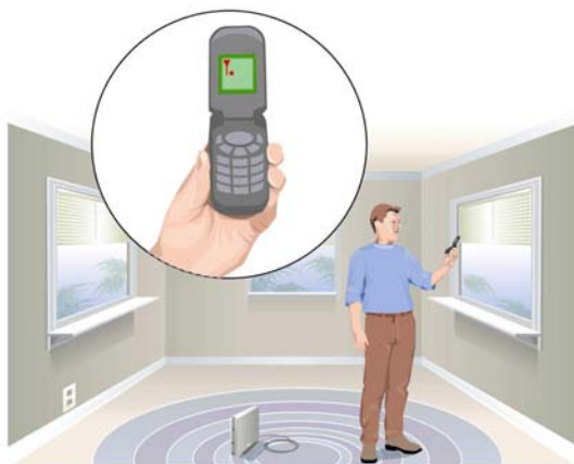
Testing signal strength at each window/installation location
