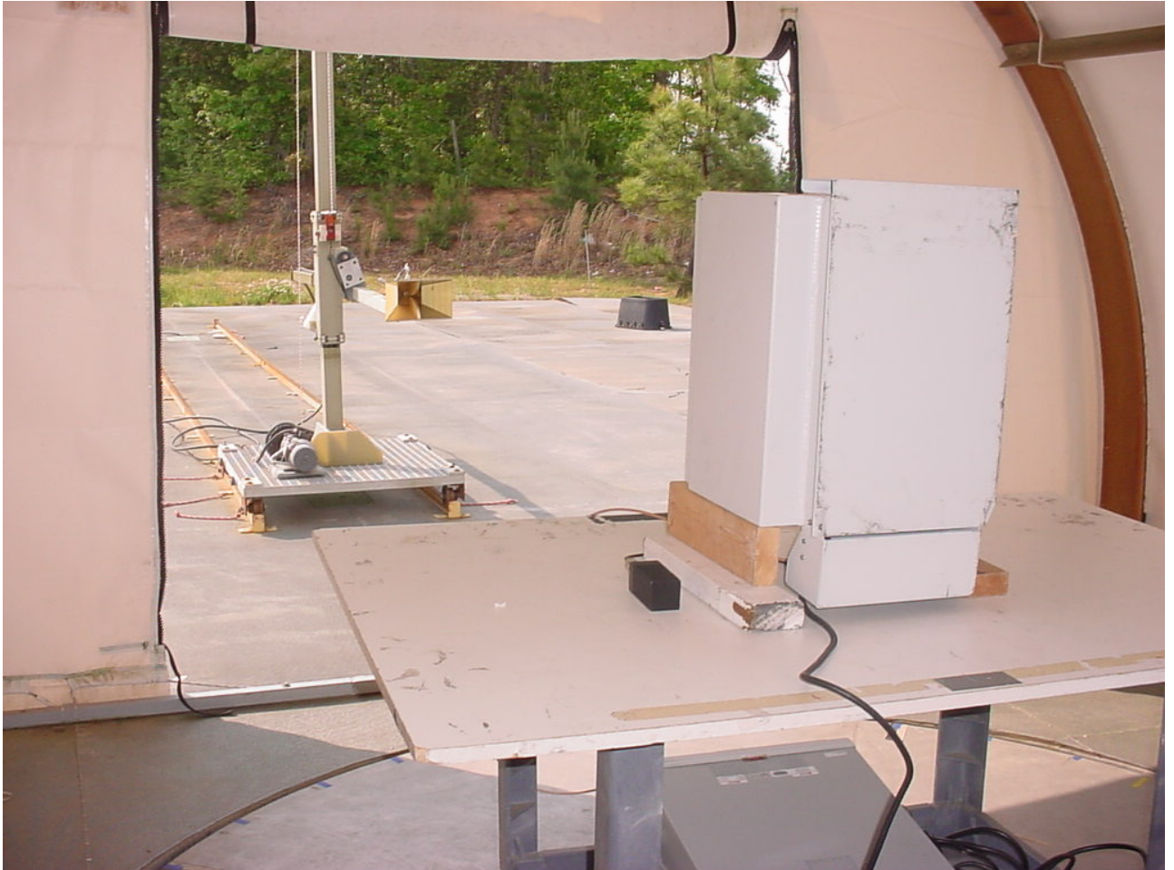
Figure 2: Test Setup - Radiated Emissions - Intentional
