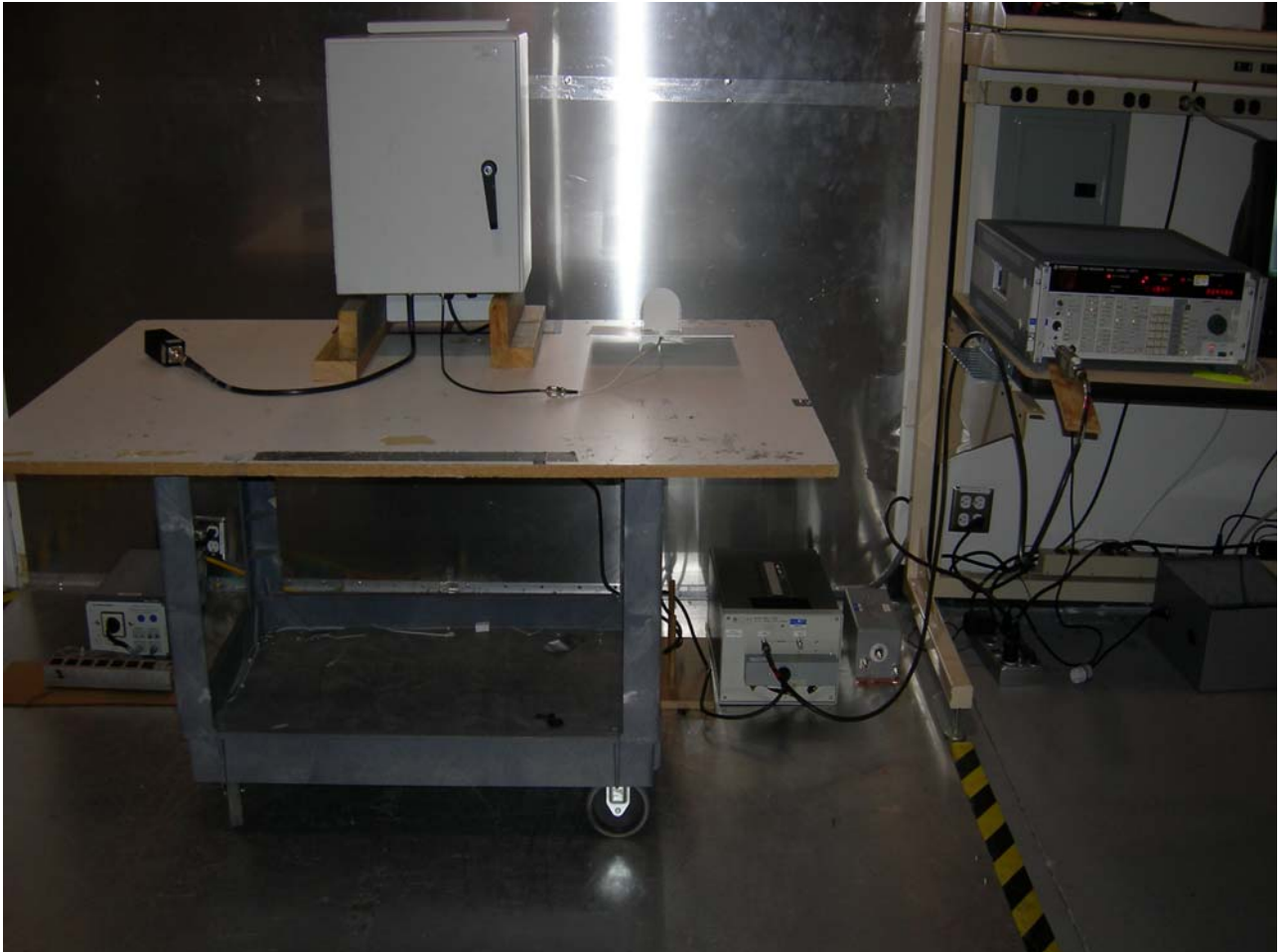
Figure 5: Line Conduction Emissions Front
