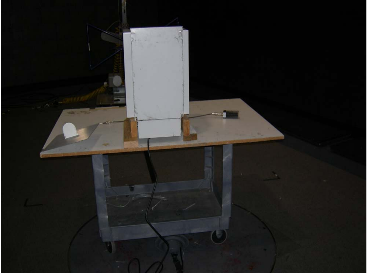
Figure 4: Test Setup - Radiated Emissions - Unintentional
