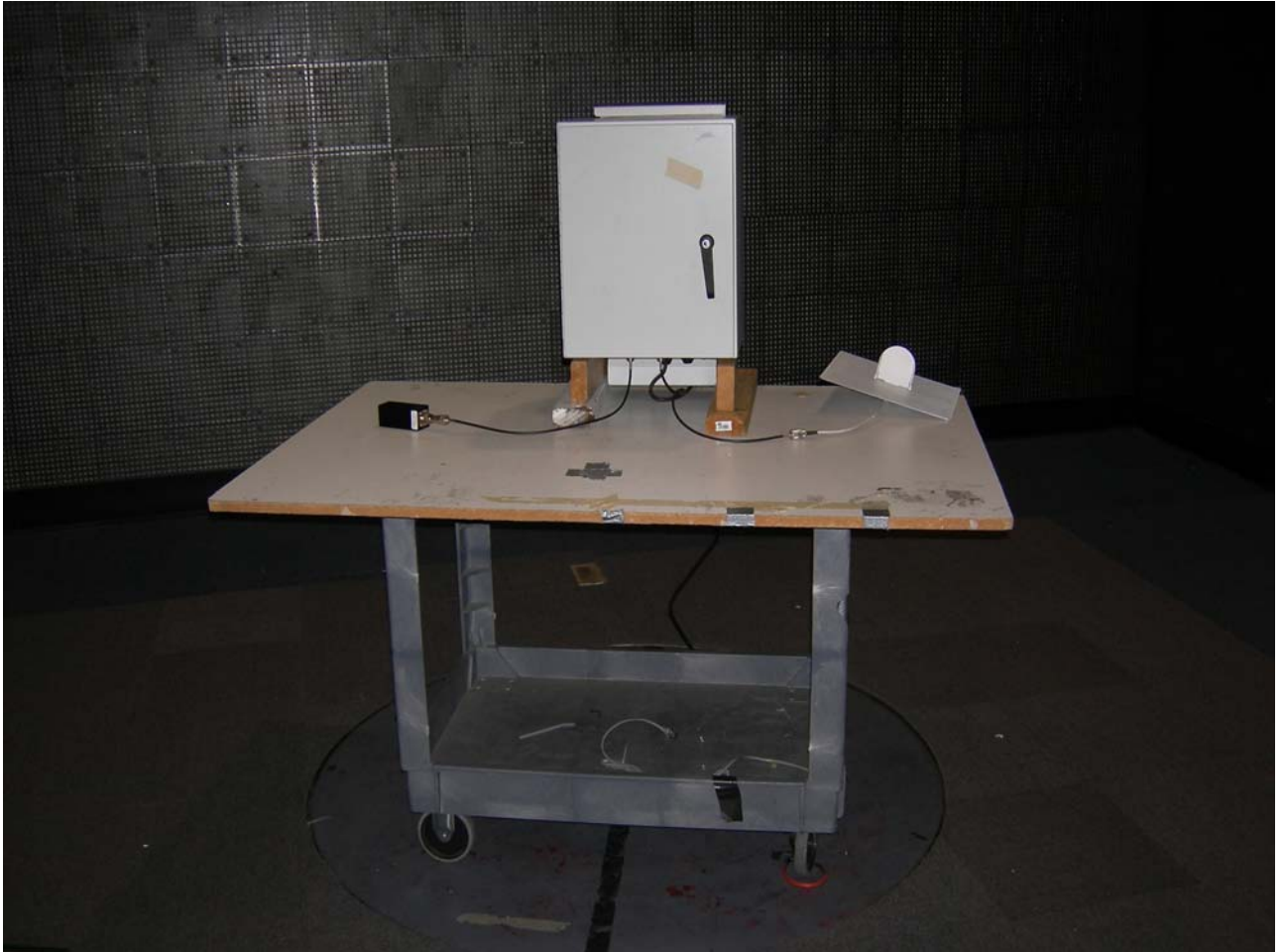
Figure 3: Test Setup – Radiated Emissions - Unintentional
