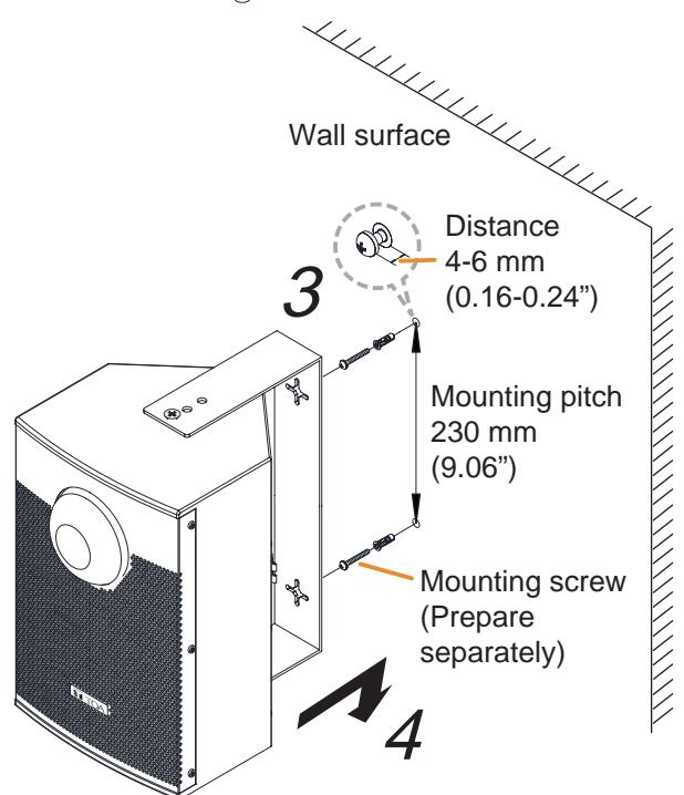
**Step 4.** Hook the **MAIN UNIT** or **SUB UNIT** with the wall mounting bracket installed to the wall mounting screws.
