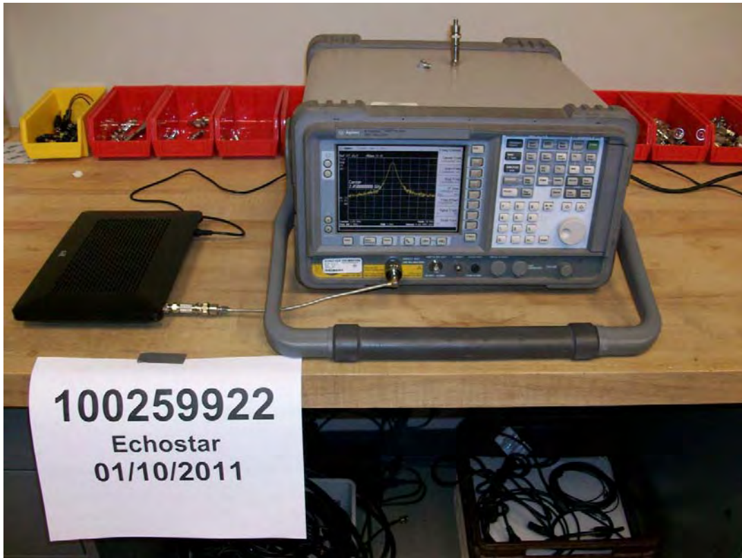
Test setup – RF Conducted Port Measurements
