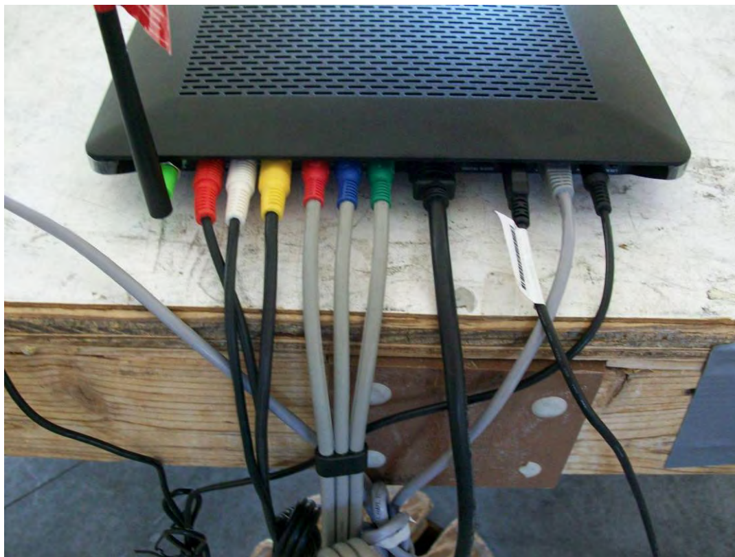
Test setup – Field Strength Measurements (Rear View)
