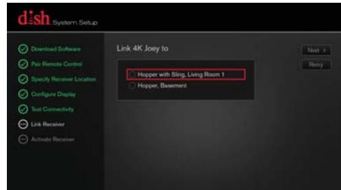
**b.** Wait while your 4K Joey links to your Hopper. If your 4K Joey cannot link to your Hopper, check both receivers' cable connections. Then, using your remote control, highlight "Retry" and then press the SELECT button on your remote control.
