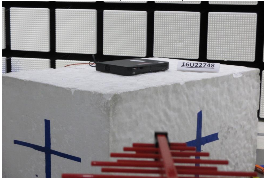
RADIATED FRONT PHOTO (BELOW 1 GHz)
