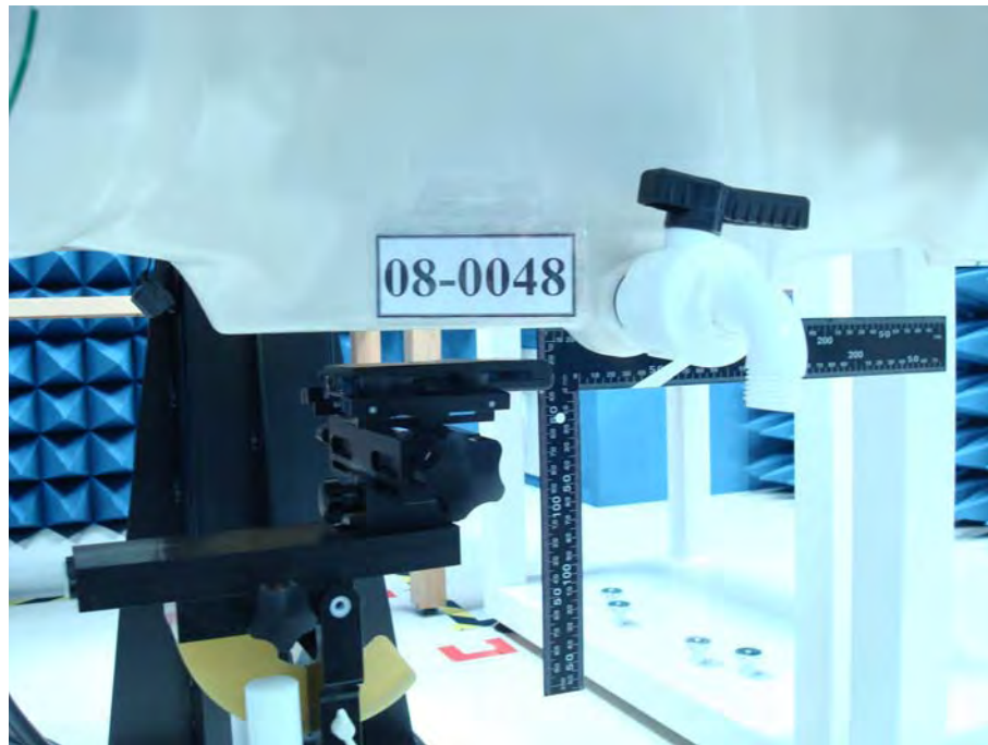
Figure 17.Body SAR Test Setup (Flat Section) _ 20 mm separation
