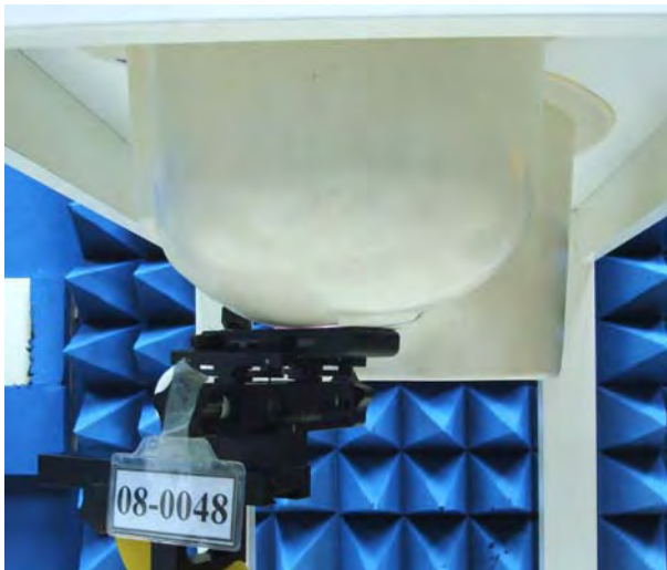
Figure 15. Left Head SAR Test Setup (Cheek)
