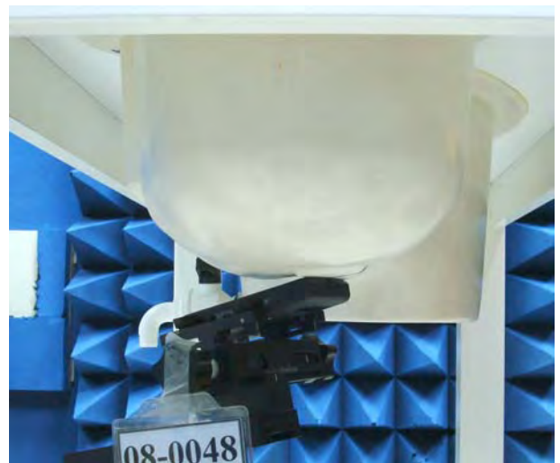
Figure 16. Left Head SAR Test Setup (Tilted)
