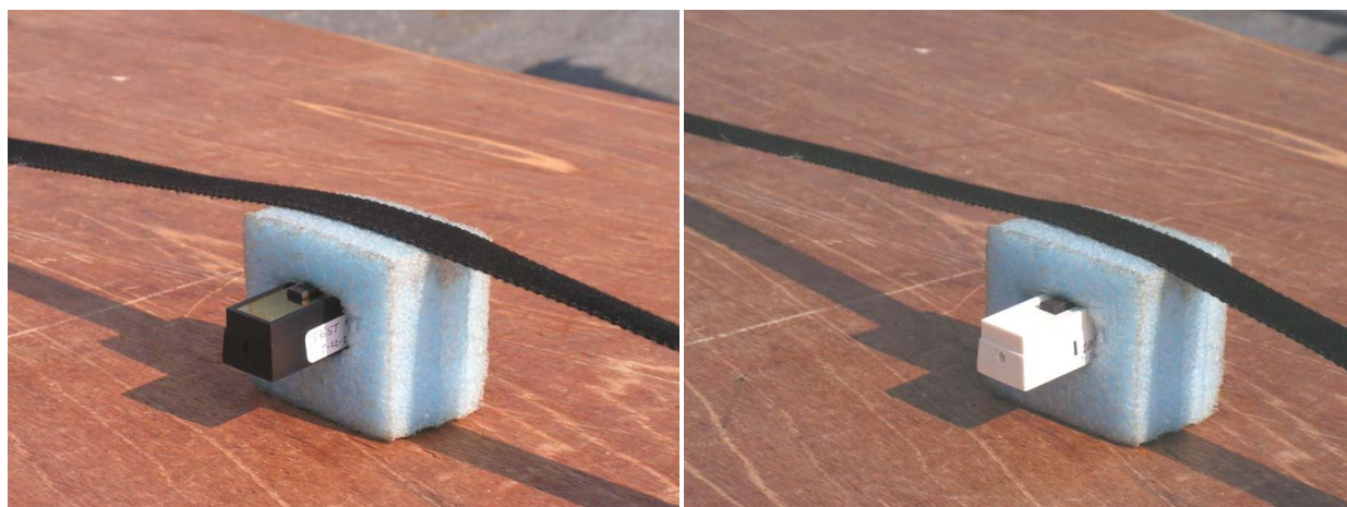
Photograph 6.6. Close-up of DUT on OATS (one of three axes tested)
