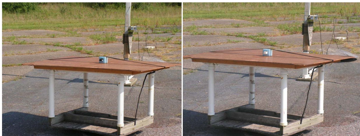
Photograph 6.5. DUT on OATS (one of three axes tested)
