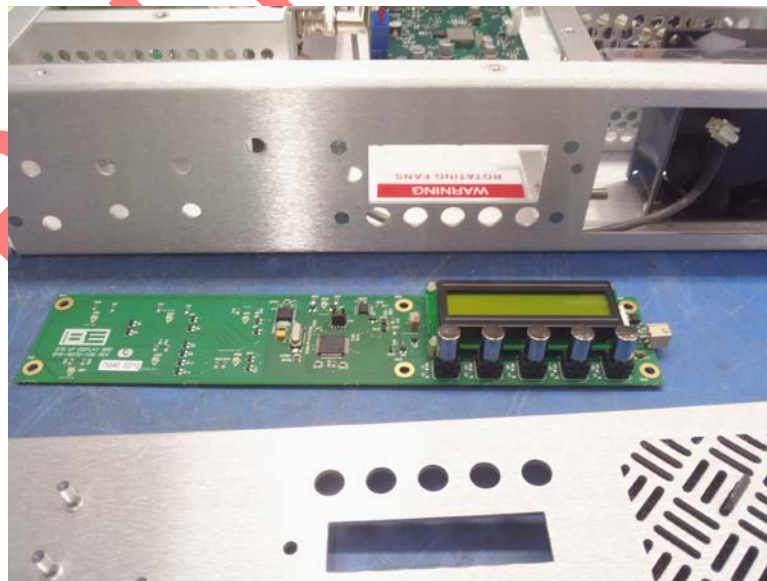
Figure 31 – Front Panel Board Assembly
