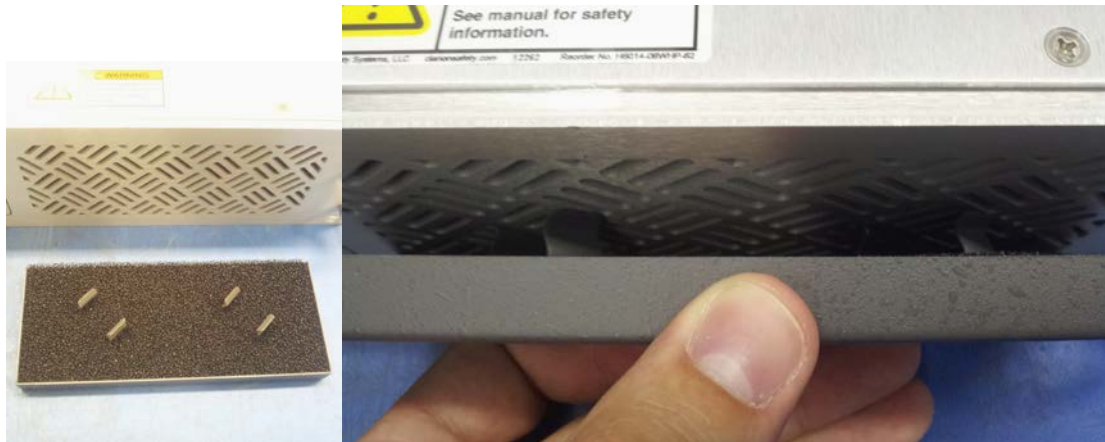
Figure 17 – Re-insertion of Air Filter
