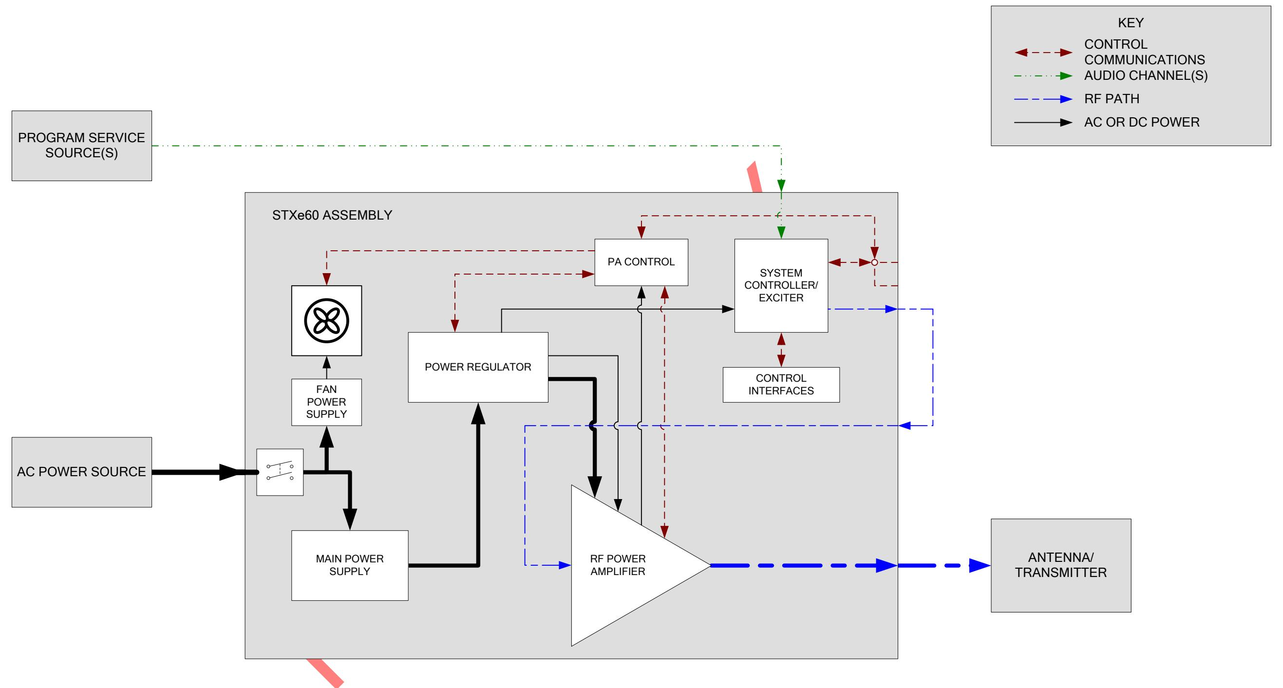
Figure 10 – STXe60 System Block Diagram
