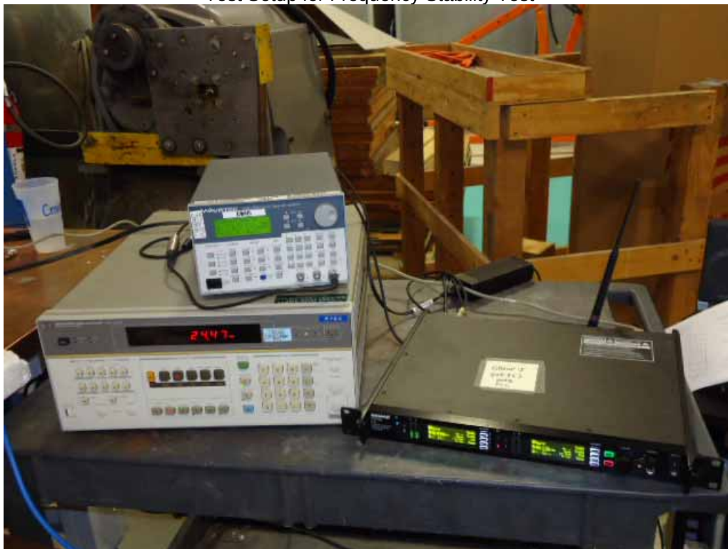
Test Setup for Occupied Bandwidth Test
