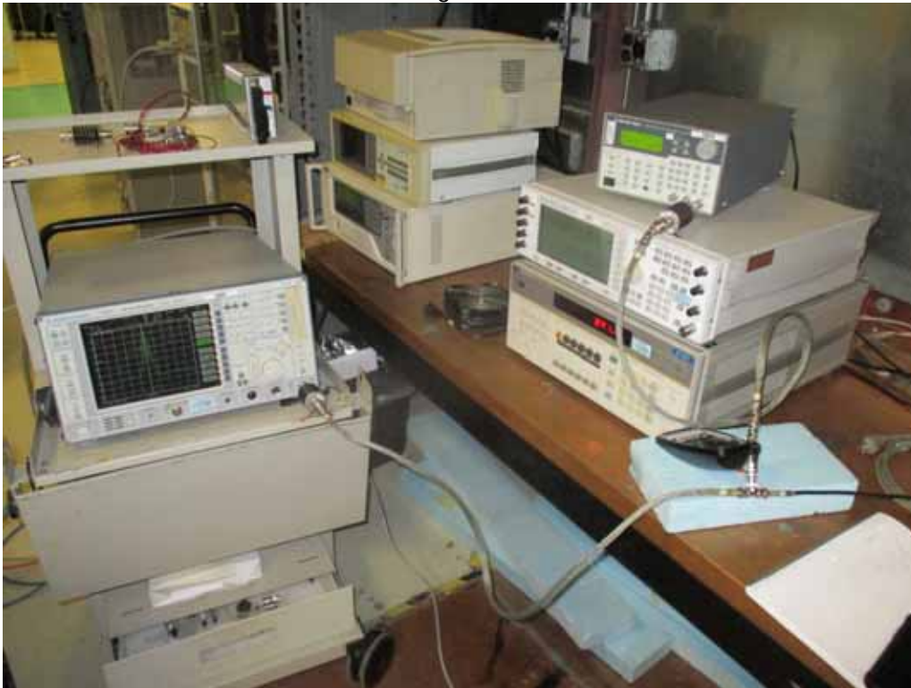
Test Setup for Occupied Bandwidth Test
