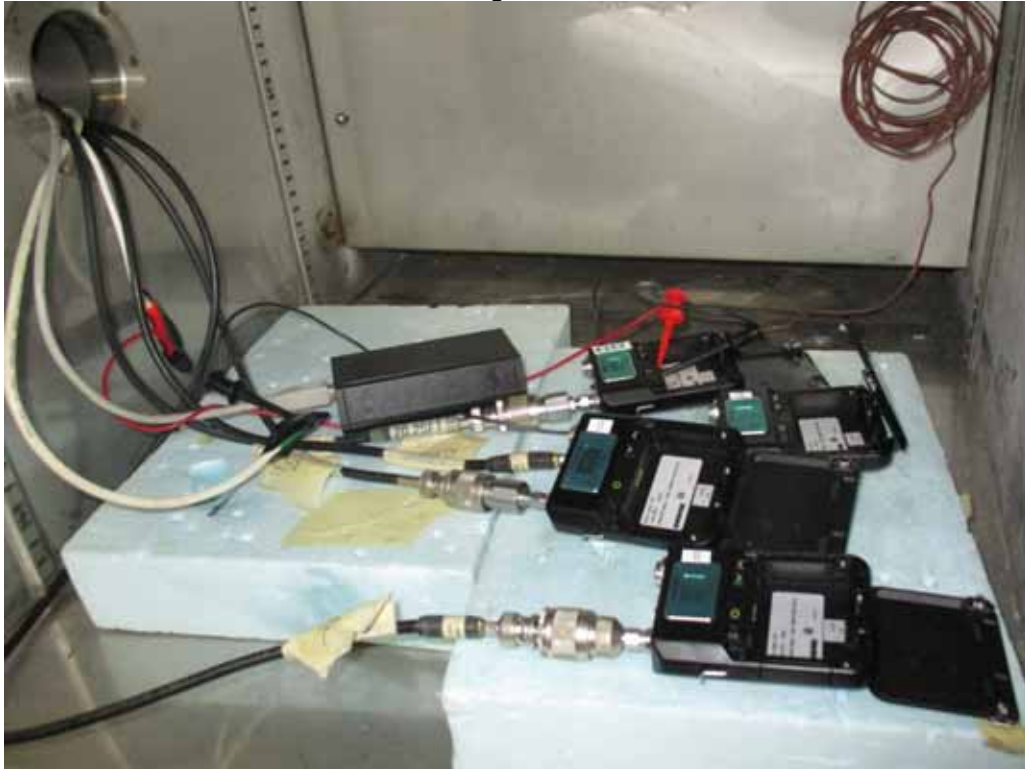
Test Setup for Frequency Tolerance Tests
