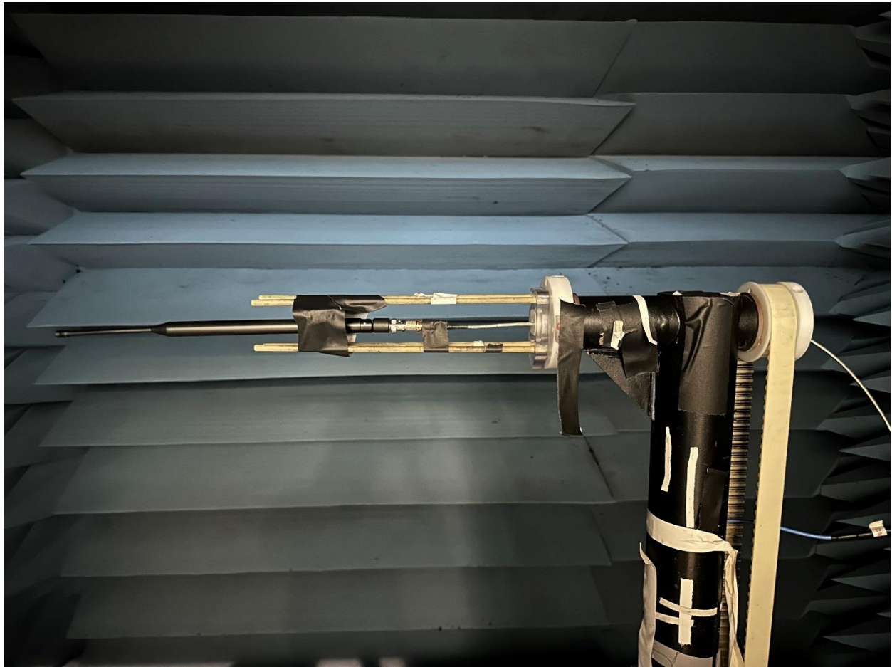
Figure 4 Photo of Shure UA8 in Antenna Chamber
