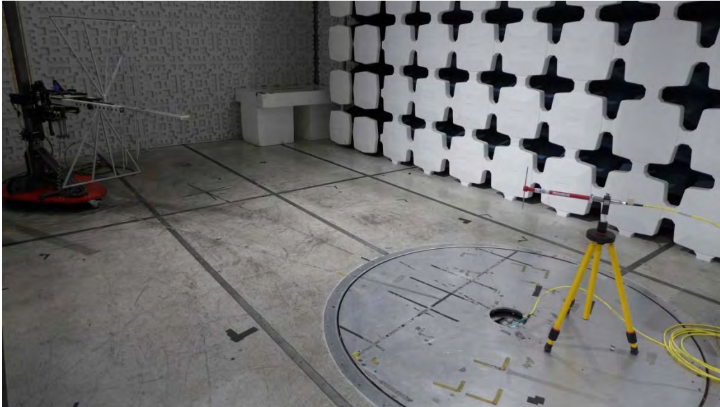
Figure E-5 - Test Setup for Spurious Emissions Matching 30MHz to 10GHz
