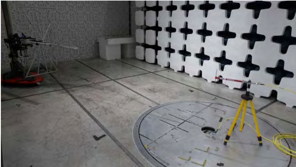
Figure E-7 - Test Setup for Spurious Emissions Matching 25MHz to 1GHz
